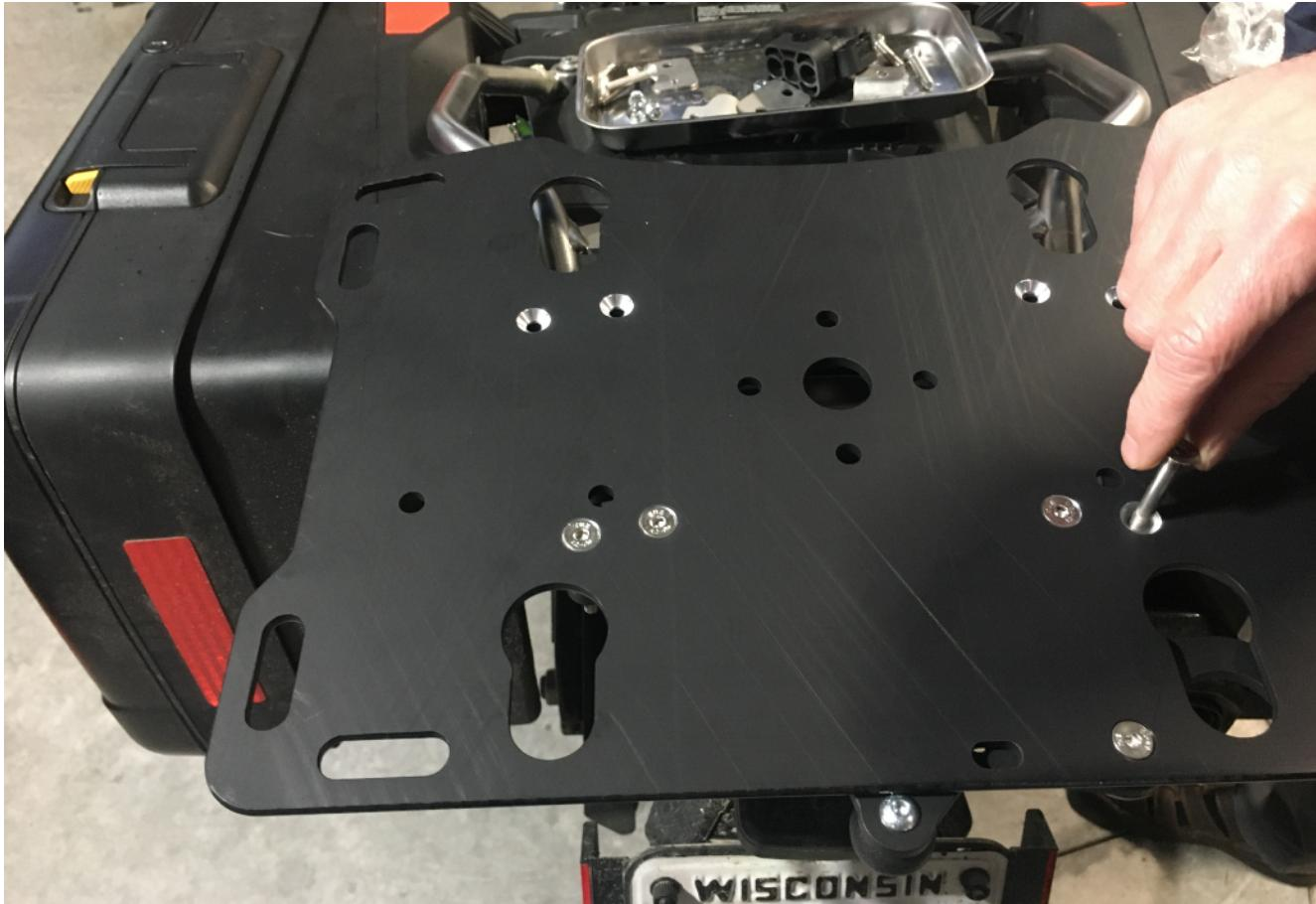
**Step 2** Place the Slider Plate on top of the clamp halves and insert the four M6 x 45 flat head screws through the plate and clamp halves in the rear.
