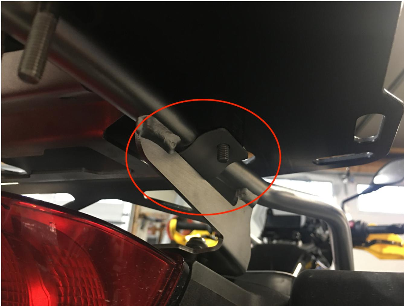
**Step 3** Insert the formed clamp bottoms into the slot of the OEM tube rack and insert the four M6 x 30 flat head screws as shown.
