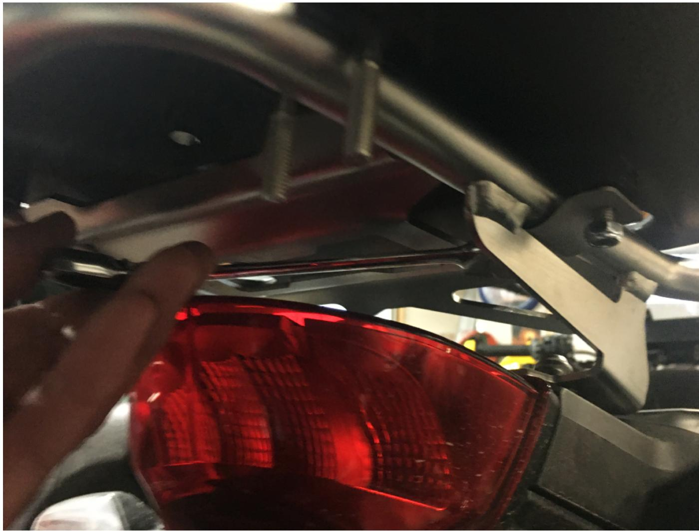
**Step 4** Thread the M6 lock nuts onto the front four flat head screws.
