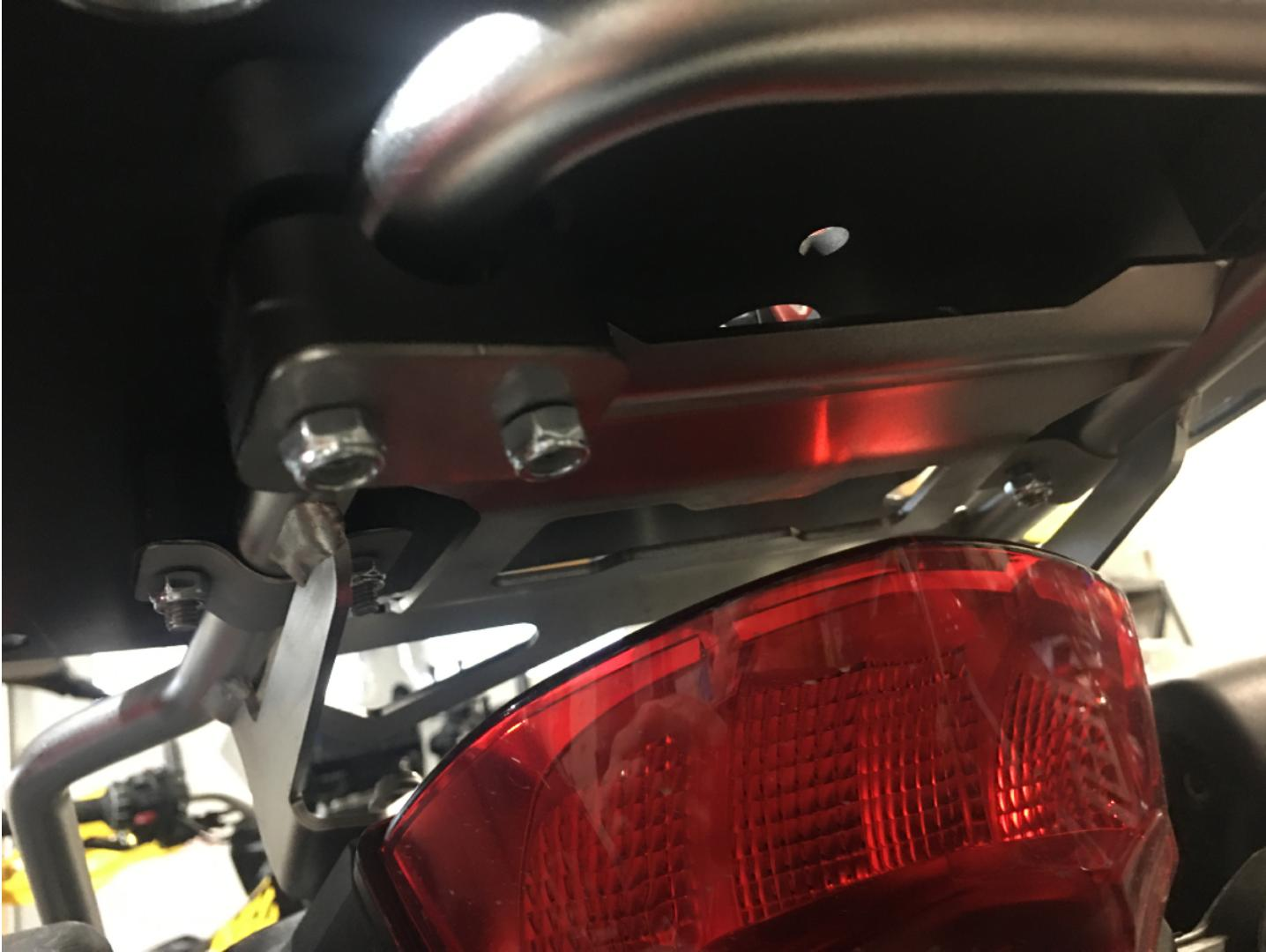
**Step 5** Install the nylon bottom clamp halves, stainless steel plates and M6 lock nuts on the rear clamp screws as shown in the photo. Install both LH and RH sides.
