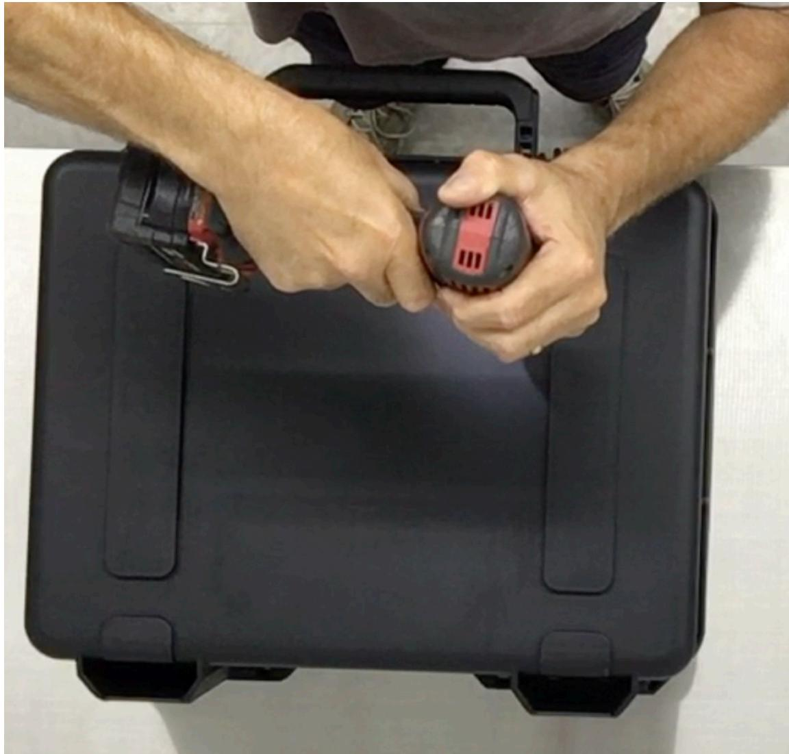
**Step 13** Remove the Slider plate from the case. Use the 21/64" drill bit and electric drill to enlarge the 1/4" pilot hole.
