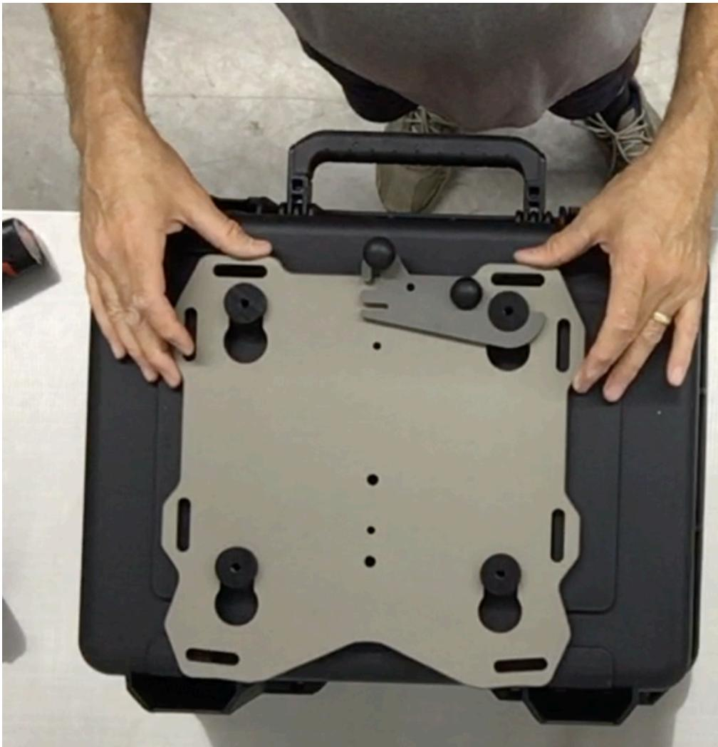
**Step 10** Place the case on a table or other work surface. Remove the 4 flat head screws holding the Slider plate onto the motorcycle. Place the Slider plate with the pucks installed onto the case.
