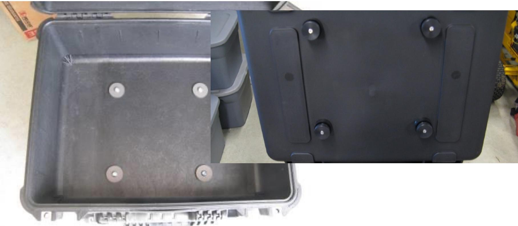
**Step 20** Install all pucks onto the case using the M8 flat washers and M8 button head cap screws. Lightly snug the puck screws at this time, later they will be fully tightened.
