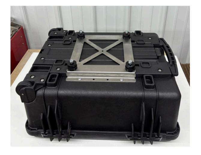
**Step 9** Attach the adapter plate to the case using <u>eight</u> 1/4" x 5/8" button head screws, 1/4" flat washers and 1/4" lock nuts. Fully tighten all 8 lock nuts with the hex wrench and 7/16" combination wrench. **Note1:** The flat washers <u>must</u> be located inside the case. **Note 2:** The button head screw can be inserted from outside the case (shown above) or from the inside of the case which ever orientation is preferred.
