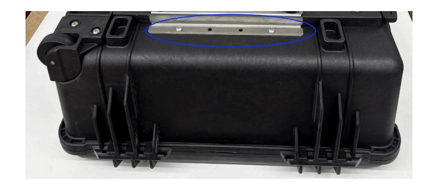
**Step 2** Use the adapter as a drill guide, drill one 1/4" hole in the case and then insert a 1/4"x 5/8" button head screw in the hole. Repeat with the other 7 holes, insert a screw after drilling each hole. **Note:** It works best to drill the second hole on the opposite side of the adapter diagonally across from the first hole drilled.
