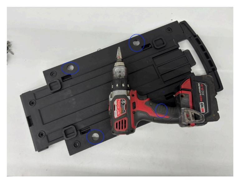
**Sept 6** Use a step drill to enlarge the 1/4" holes to 3/4" holes.
