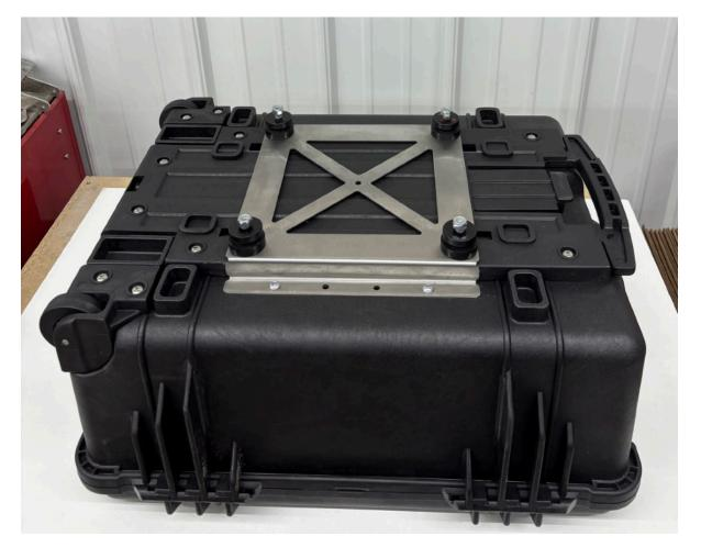
**Step 7** Re-install the handle cover. **Note:** be careful not to strip the screw bosses in the case.
