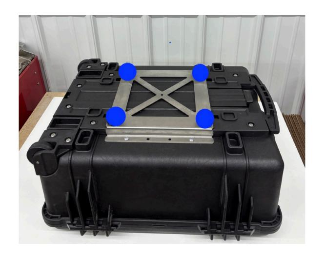
**Step 3** The 1560's handle cover will have to be removed to drill puck screw head clearance holes. Use the adapter plate as a template and mark the cover handle at the hole locations identified by the blue dots (a pencil or paint marker will work good for this).
