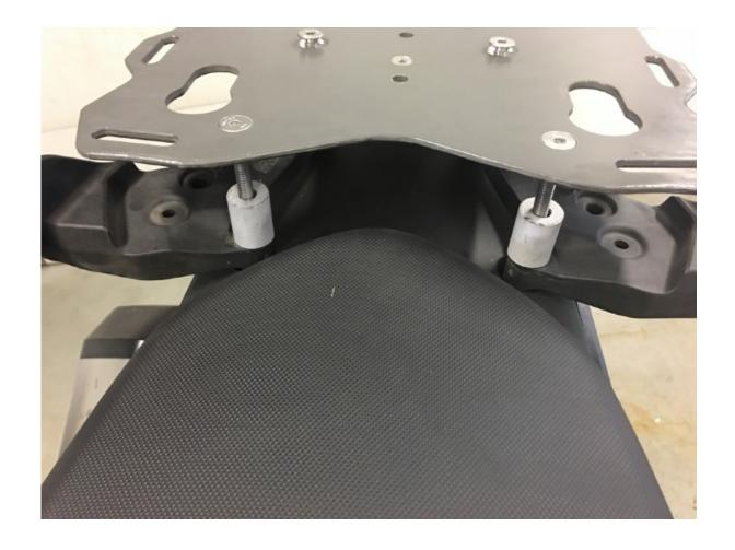
Step 6 Place the long angled spacers over the front holes of the grab handles. The spacer angled end must face upward and with the lowest point of the spacer facing toward the front of the motorcycle. Insert the 2 remaining 70mm BRE screws.
