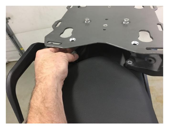
Step 5 Remove the front OEM screws.
