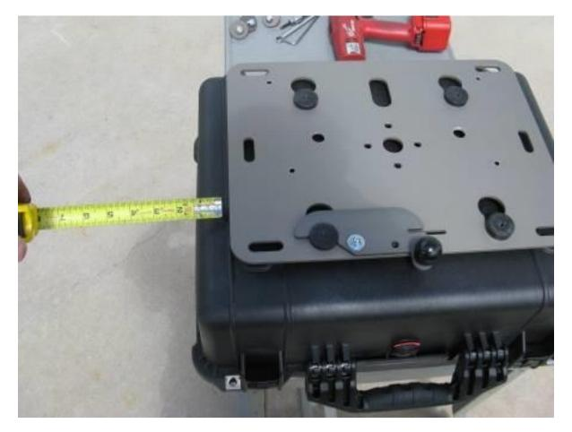
Step 13 Locate the puck marker on the box and align the master puck up with the mark as it was on the bike.
