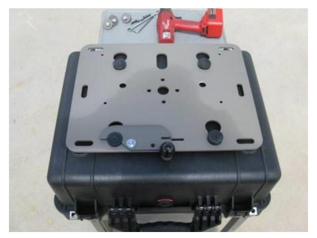
Step 12 Place the box on a table or other work surface. Remove the 4 flat head screws and nuts holding the rack onto the mounting brackets.
