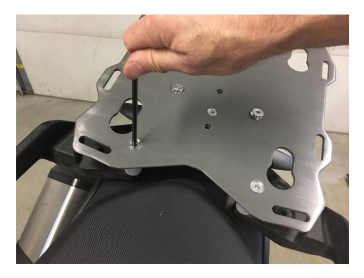
Step 7 Snug the four flat head screws with a 5mm hex wrench. Verify that the angled spacers are positioned correctly with the angled low point facing the front of the motorcycle.
