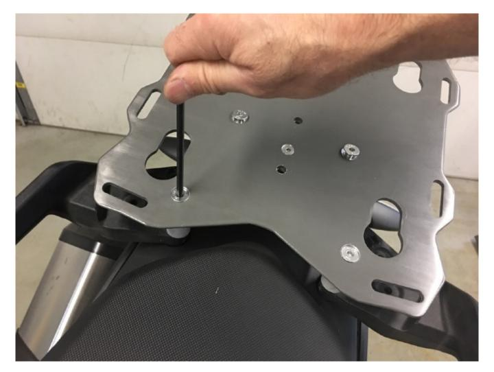
Step 23 Re-install the plate on the spacers. Re-install the M8 flat head screws and torque to 17 ftlbs.
