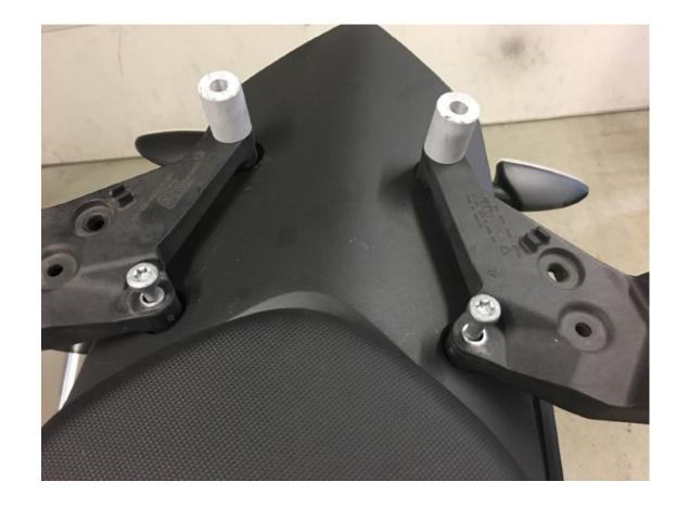
Step 3 Place the short spacers over the rear mounting holes of the handles. The spacer must be positioned with the angled cut on top with the lowest point of the spacer facing the front of the motorcycle.
