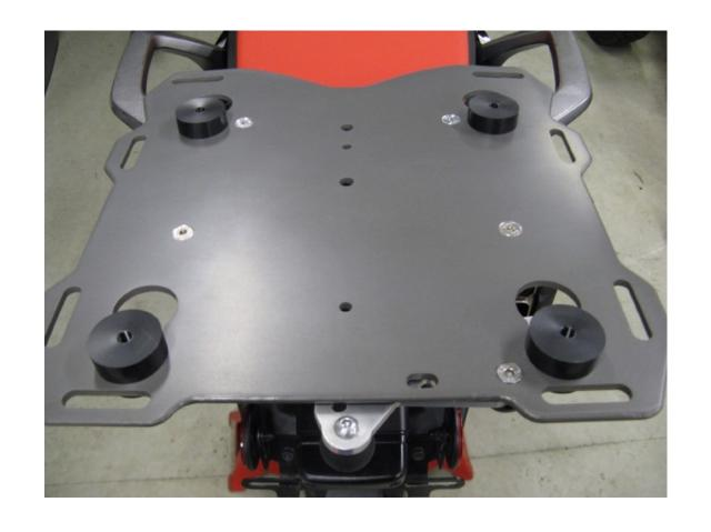
Step 10 Insert the 3 remaining pucks into the keyholes in the plate.
