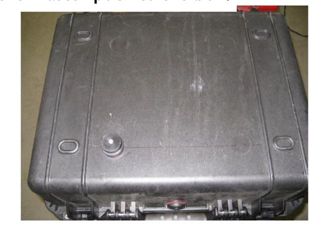
Step 16 Use the 5/16" button head cap screw and 1 1/2" aluminum washer to attach the master puck to the box.
