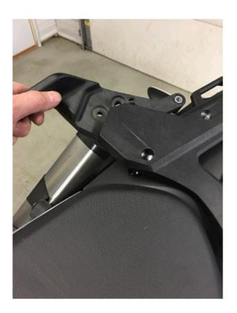
Step 1 Remove the OEM top plate and grab handles by removing the four T45 head bolts.
