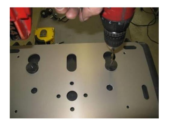
Step 18 With the 1/4" drill bit, use the puck diagonally across from the master puck as a drill guide and drill a second pilot hole in the box.
