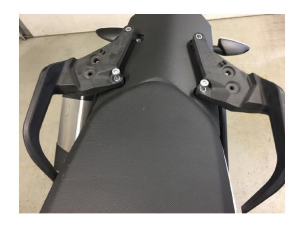
Step 2 Re-install the grab handles using only the front OEM screws to retain the handles. Tighten the screws only 2 - 3 revolutions.
