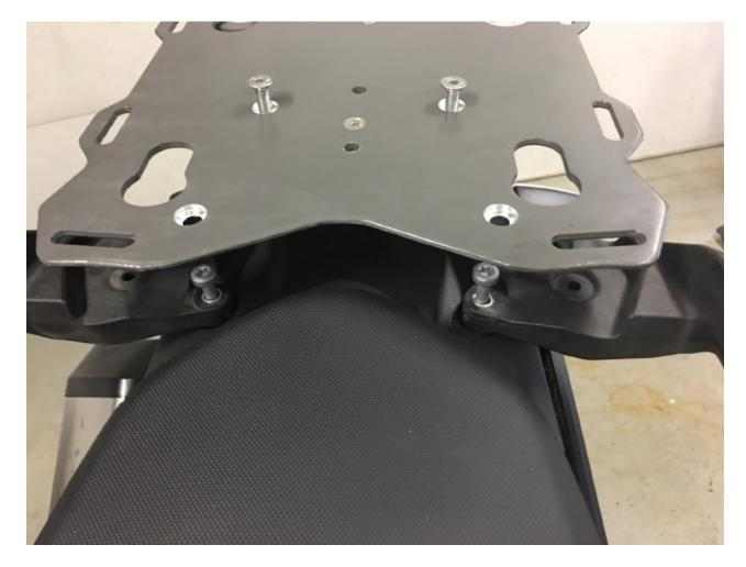
Step 4 Install the plate with the 2 rear BRE 65mm screws. Insert the screws through the spacers and thread into the subframe. Tighten the screws only 2- 3 revolutions at this time.
