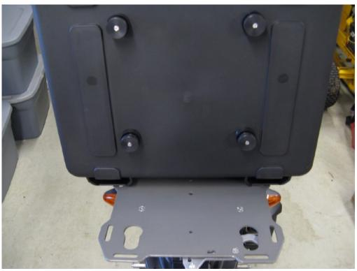
Step 22 Install all pucks onto the box using the 1 1/2" aluminum washers and 5/16" button head cap screws.
