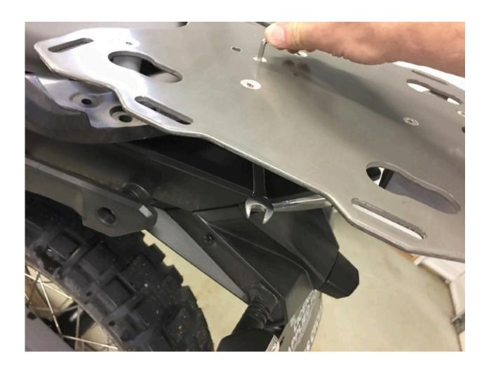
Step 8 Tighten the sub plate's two 6 mm screws and lock nuts using a hex key wrench and a 10mm combination wrench.
