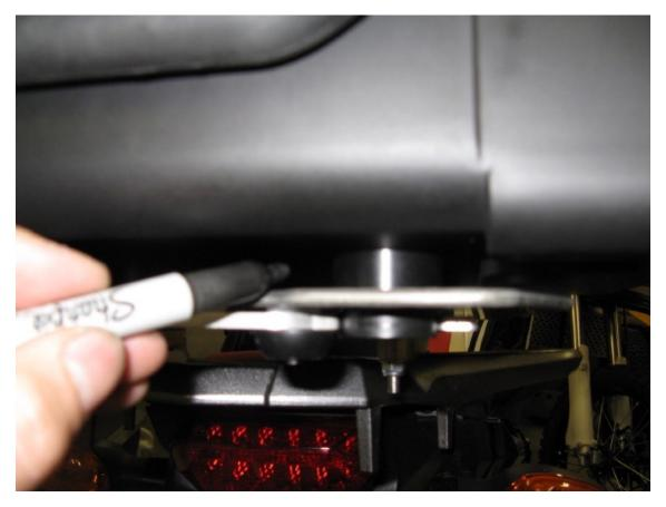
Step 11 Position the box on top of the pucks. Determine the for/aft location (side to side will be determined later). Position the box as far forward as possible without interfering with passenger comfort. Also consider if you will be placing any gear on the seat or if you want to be able to remove the seat with the box in place. Use a marker to mark the master puck location on the box.
