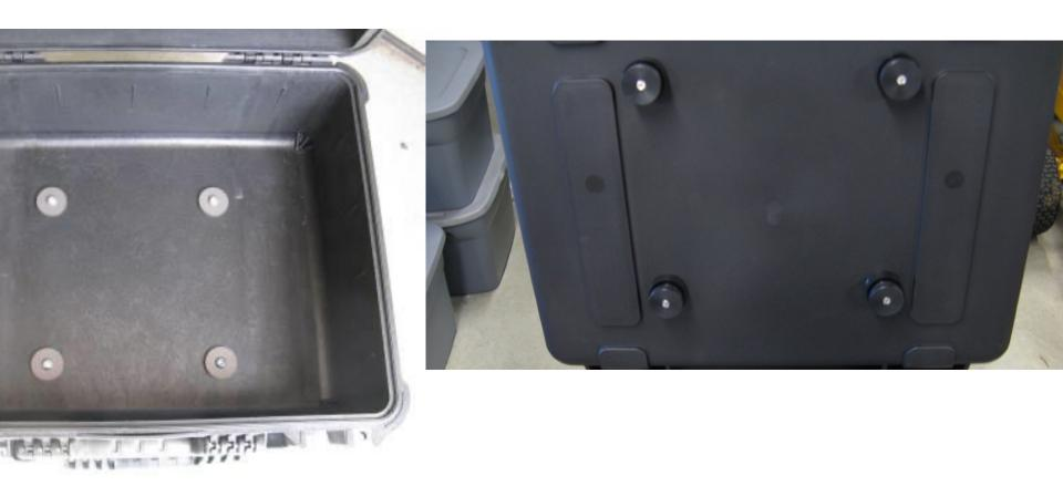
**Step 18** Install all pucks onto the case using the M8 flat washers and M8 button head cap screws. Lightly snug the puck screws at this time, later they will be fully tightened.
