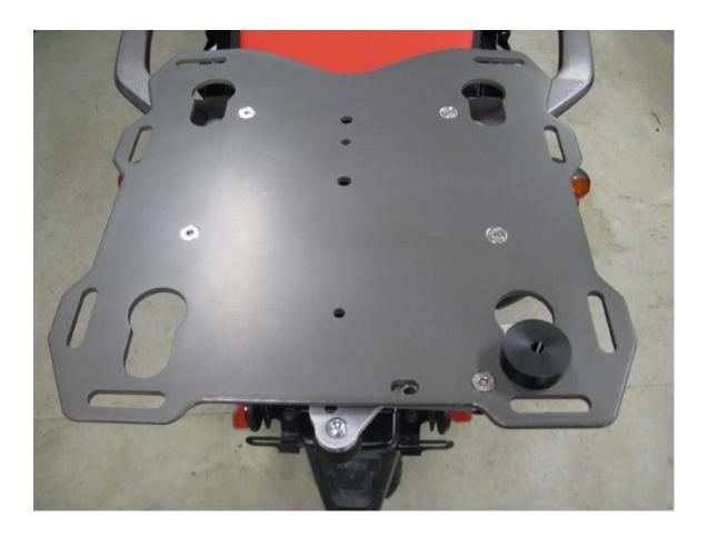
Step 5 Install one of the black plastic pucks into the key hole with the cam lever. Lock the puck into place with the cam lever. This will be referred to as the "Master Puck" Note: Remove the large washer and screw from the puck before putting into the plate. The screws and washers are installed into the pucks for shipment as part of our QA process.
