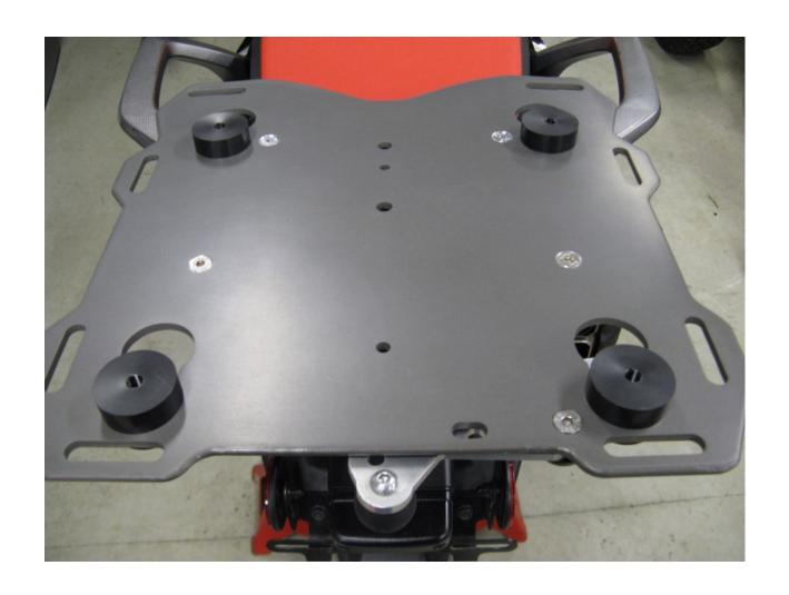
**Step 6** Insert the 3 remaining pucks into the keyholes in the plate.
