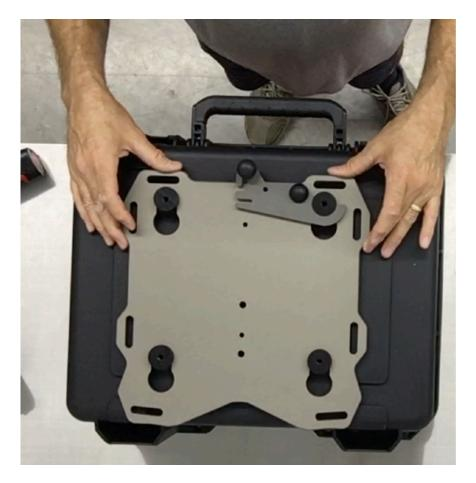
**Step 8** Place the case on a table or other work surface. Remove the 4 flat head screws and nuts holding the Slider plate onto the OEM rack. Place the Slider plate with the pucks installed on the case.
