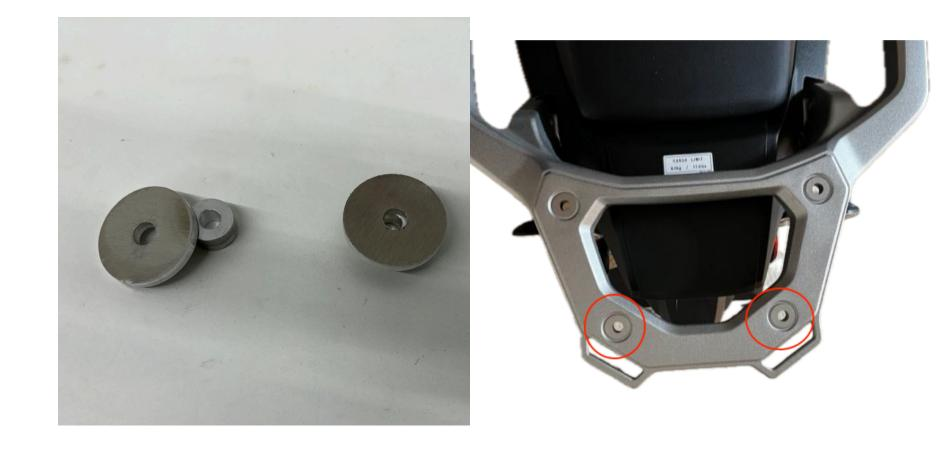
**Step 2** Stack the 41 x 5 mm aluminum spacers on top of 22 x 8 mm aluminum spacers. Place a spacer stack over each of the rear holes as shown. **Note:** Make certain the uncoated side of the large diameter spacer faces upward toward the Slider plate.
