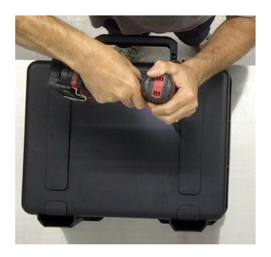
**Step 11** Remove the Slider plate from the case. Use the 21/64" drill bit and electric drill to enlarge the ½" pilot hole.
