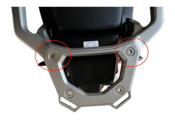
**Step 1** Install the 22 x 13 long aluminum spacers at the front of the OEM rack in the location shown.
