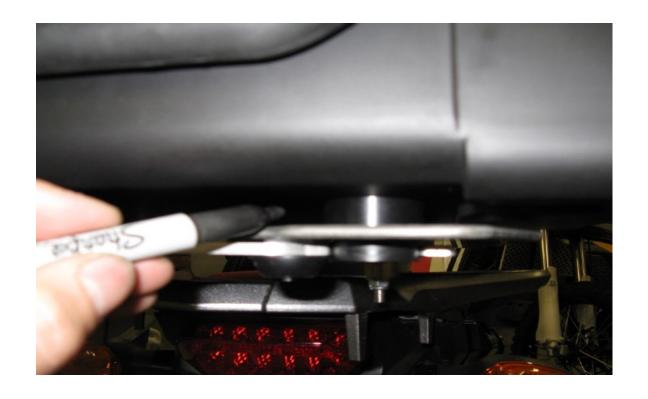
**Step 7** Position the case on top of the pucks. Determine the for/aft location (side to side will be determined later). Position the box as far forward as possible without interfering with passenger comfort. Also consider if you will be placing any gear on the seat or if you want to be able to remove the seat with the box in place. Use a marker to mark the master puck location on the box.
