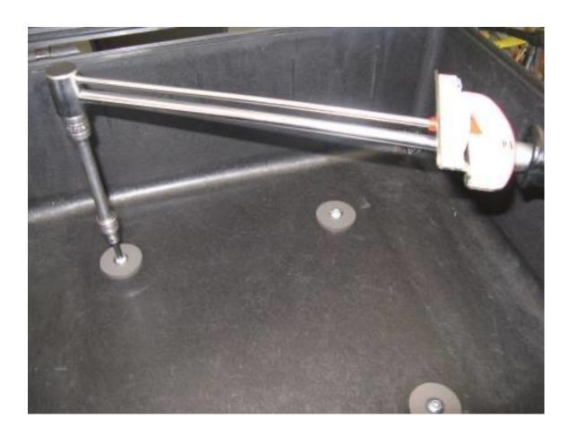
**Step 22** Torque the puck screws to 9 ft.lb. or 12.2 Nm.
