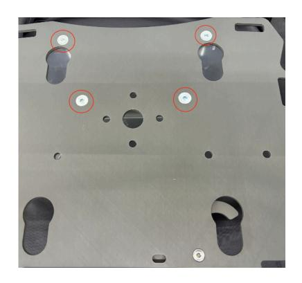
**Step 19** Re-install the plate onto the bike using the M8 flat head screws and lock nuts.
