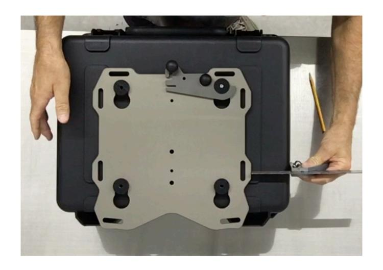
**Step 13** Place the Slider plate with the other 3 pucks onto the master puck and latch it into position. Square up the plate and box to each other (last chance).
