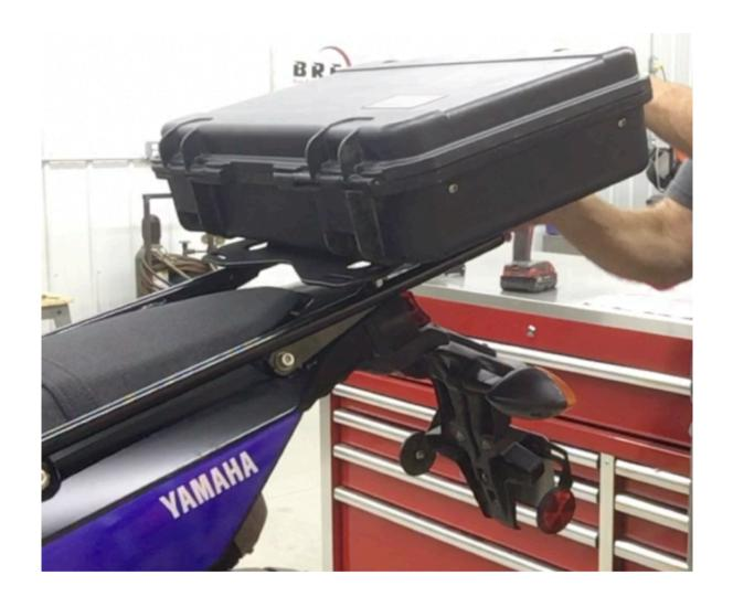
**Step 21** Install the case onto rack and latch it into place with the cam lever.
