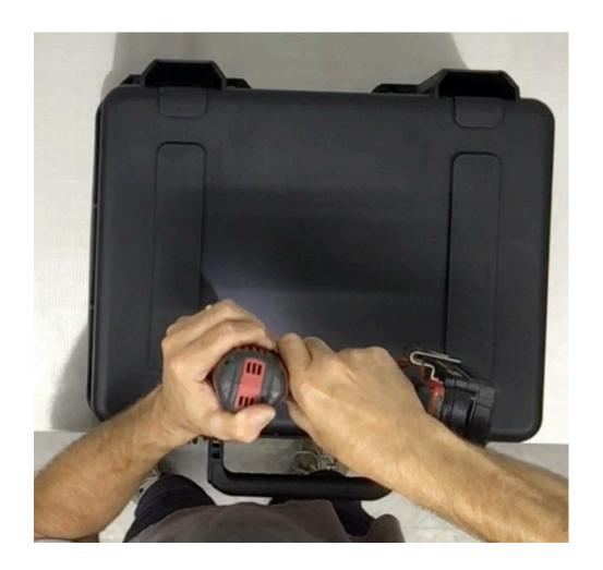
**Step 6** Remove the Slider plate from the case. Use the 21/64" drill bit and electric drill to enlarge the ½" pilot hole.
