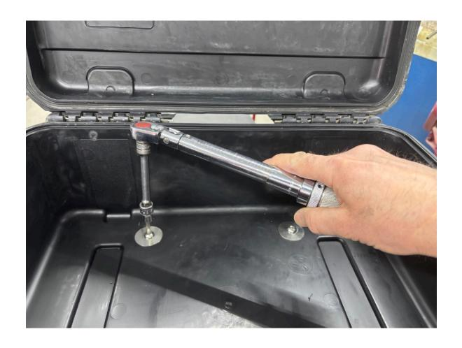
**Step 14** Once the Slider rack is installed on the motorcycle slide the case into the Slider and latch the cam lever. Torque the four puck screws to 9 ft.lb. or 12.2 Nm.
