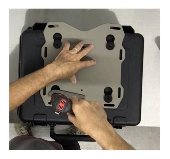
**Step 5** With one hand apply downward force on the Slider plate, use your other hand to drill the case. With a ¼" drill bit and electric drill use the master puck as a drill guide and drill a pilot hole through the case.
