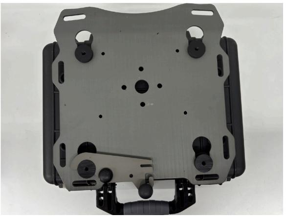
**Step 3** Rotate the pucks until the ribs on the case drop into the machined grooves in the pucks. **Note:** Verify the pucks are fully seated in the keyholes and verify the grooves and ribs are lined up allowing the pucks to sit flat on the case.
