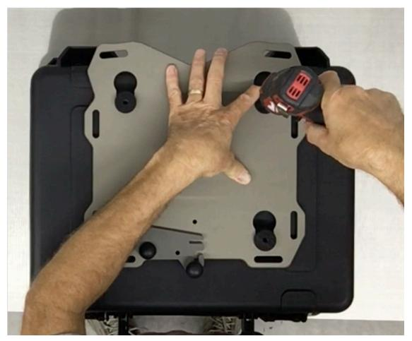
**Step 9** With the ¼" drill bit, use the puck diagonally across from the master puck as a drill guide and drill a second pilot hole in the case.
