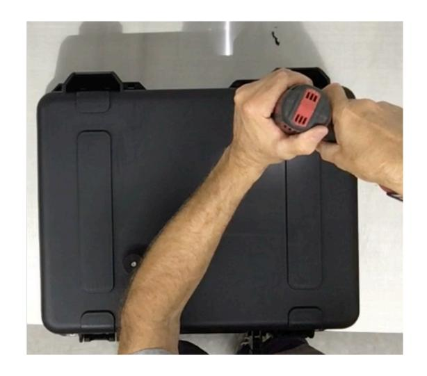
**Step 10** Remove the Slider plate from the case and use the 21/64" drill bit to enlarge the second 1/4" pilot hole.
