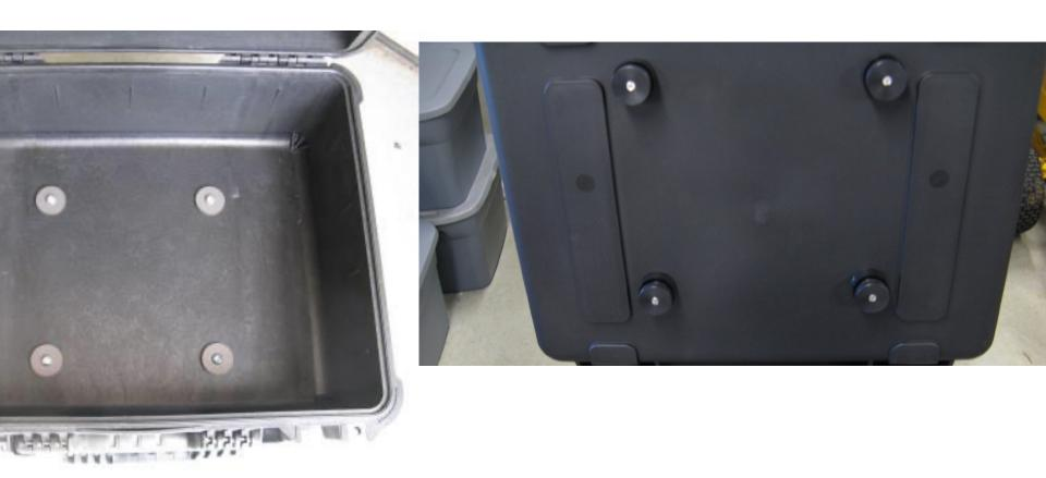
**Step 13** Install all pucks onto the case using the M8 flat washers and M8 button head cap screws. Lightly snug the puck screws at this time.
