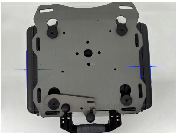
**Step 4** Using a rule or combination square verify the side to side location is equal. Once the checks in step 3 & 4 are complete you are ready to drill.
