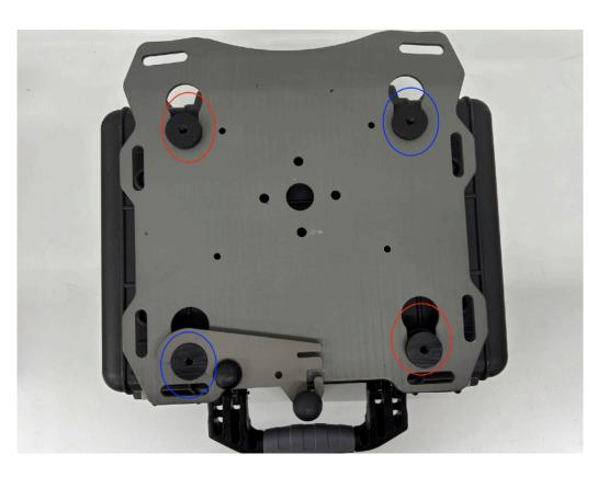
**Step 2** locate the other Red and Blue pucks and insert them into the Slider plate in the correct location, see Note on page 1.
