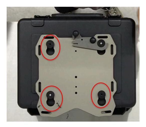
Step 11 Attach the second puck to the case with the M8 hardware. Place the Slider rack on the case and latch it into position. With the ¼" drill bit use the 2 remaining pucks as drill guides and drill the last two 1/4" holes Note: Apache 3800 case verify the case ribs are seated in the puck grooves.
