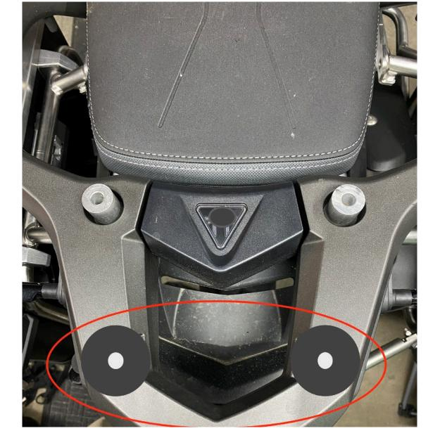
Step 3 Place one 38 mm OD x 9.5 ID x 5 mm long aluminum spacer over each of the short (rear) spacers.
