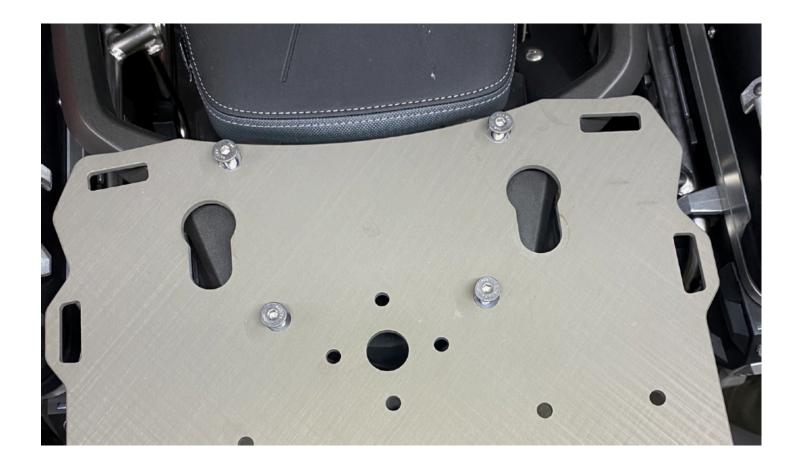
**Step 4** Position plate over the spacers as shown. Insert the screws into the four holes and through the spacers. **Note: Add Loctite to the screws at this time if you are not going to be removing the plate for locating case holes.**
