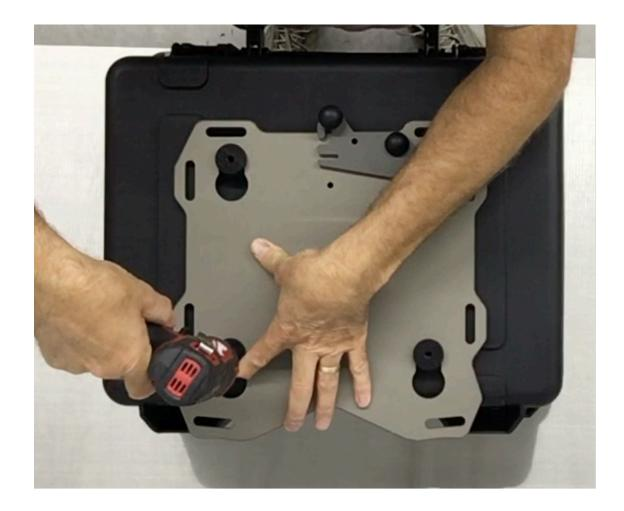
**Step 16** With the <sup>1</sup>/<sub>4</sub>" drill bit, use the puck diagonally across from the master puck as a drill guide and drill a second pilot hole in the case.
