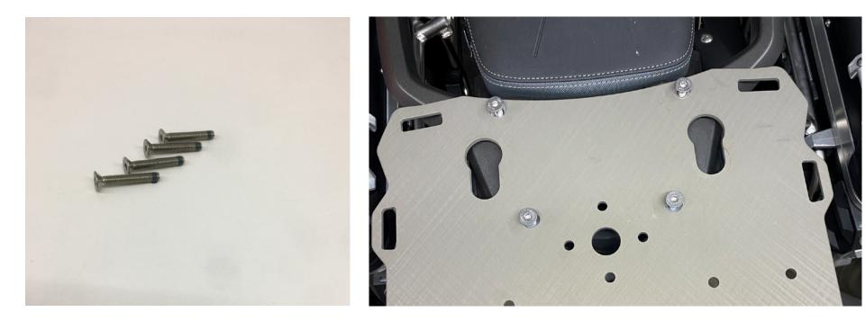
**Step 21** Apply blue 242 Loctite or equivalent the four M8 flat head screws. Re-Install the BRE plate using **step 2** through **4**.
