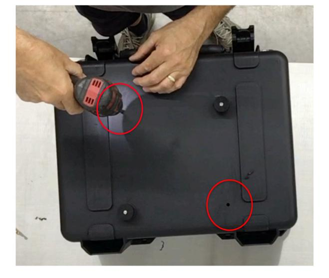
**Step 19** Remove the Slider rack and pucks from the case. Use the 21/64" drill bit and electric drill to enlarge the last 2 <sup>1</sup>/<sub>4</sub>" pilot holes.
