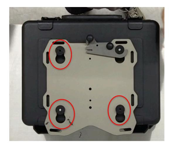
**Step 18** Attach the second puck to the case with the M8 hardware. Place the Slider rack on the case and latch it into position. With the <sup>1</sup>/<sub>4</sub>" drill bit use the 2 remaining pucks as drill guides and drill the last two 1/4" holes.
