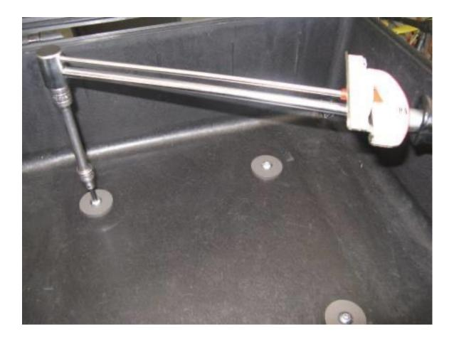
Step 24 Torque the puck screws to 9 ft. lbs. (12.2 Nm).
