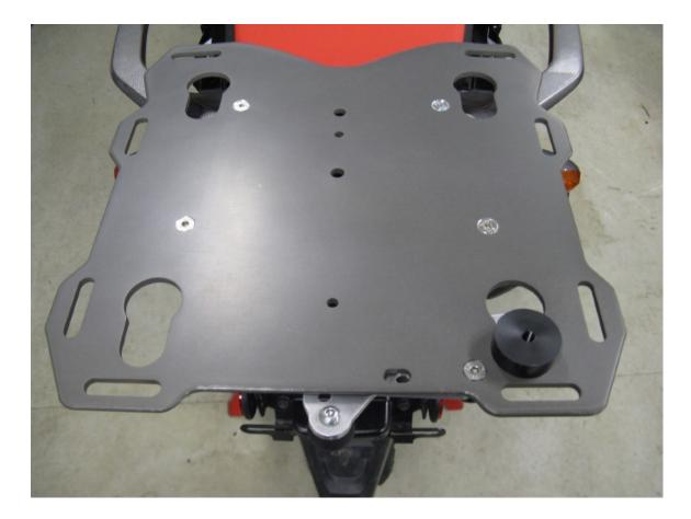
**Step 7** Install one of the black plastic pucks into the key hole with the cam lever. Lock the puck into place with the cam lever. This will be referred to as the "Master Puck"
