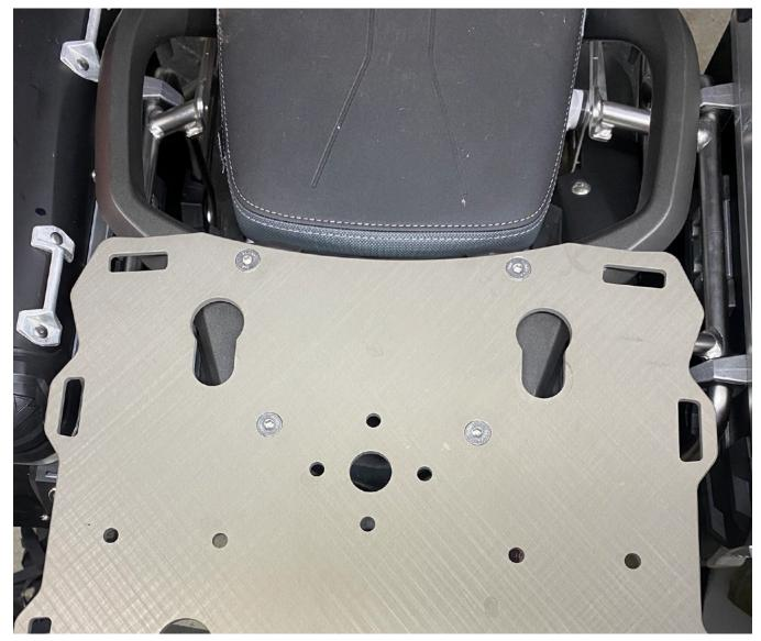
Step 5 Using a 5mm hex wrench snug the screws. Note: If you are not removing the plate for locating case holes, torque the screws to 17 in.lb (23.0 Nm).
