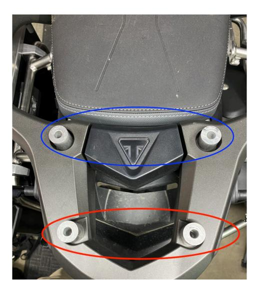
Step 2 Insert the 22 mm OD x 9.5 mm ID x 25 mm aluminum spacers (long) closest to the seat (blue). Install the 22 mm OD x 9.5 ID x 20.6 mm aluminum spacers (short) to the rear of the bike (red).
