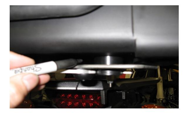
**Step 9** Position the case on top of the pucks. Determine the for/aft location (side to side will be determined later). Position the case as far forward as possible without interfering with passenger comfort. Also consider if you will be placing any gear on the seat or if you want to be able to remove the seat with the case in place. Use a marker to mark the master puck location on the case.
