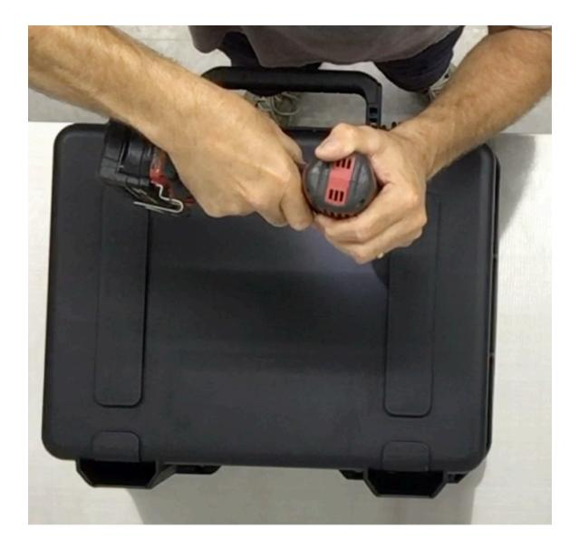
Step 13 Remove the Slider plate from the case. Use the 21/64" drill bit and electric drill to enlarge the  $\frac{1}{4}$ " pilot hole.
