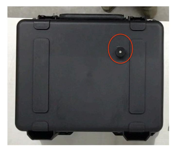
**Step 14** Use a M8 x 38 flat washer and the M8 button head cap screw to attach the master puck to the case.
