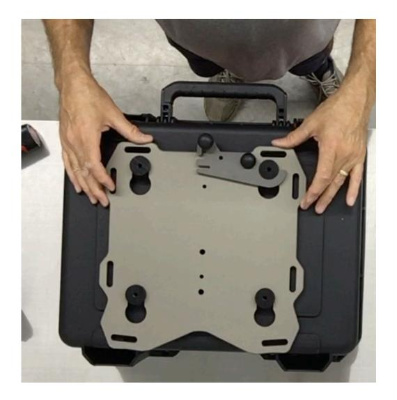
**Step 10** Place the case on a table or other work surface. Remove the 4 screws holding the Slider plate onto the motorcycle. Place the Slider plate with the pucks installed onto the case.
