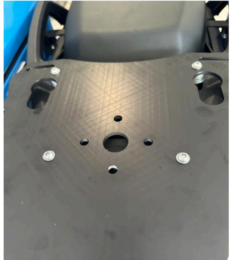
**Step 21** Apply blue 242 Loctite or equivalent the four M6 button head screws. Re-Install the BRE plate using step 5 through 6.
