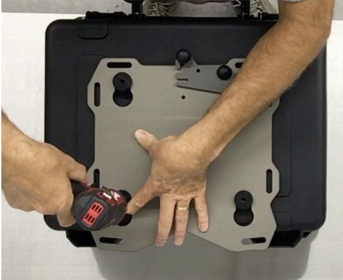
**Step 16** With the ¼” drill bit, use the puck diagonally across from the master puck as a drill guide and drill a second pilot hole in the case.
