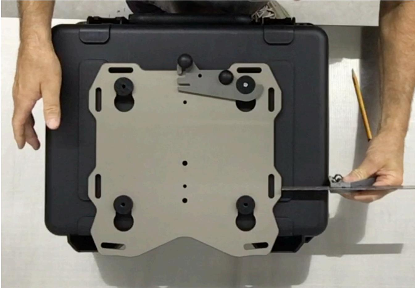
**Step 15** Place the Slider plate with the other 3 pucks onto the master puck and latch it into position. Square up the plate and box to each other (last chance).
