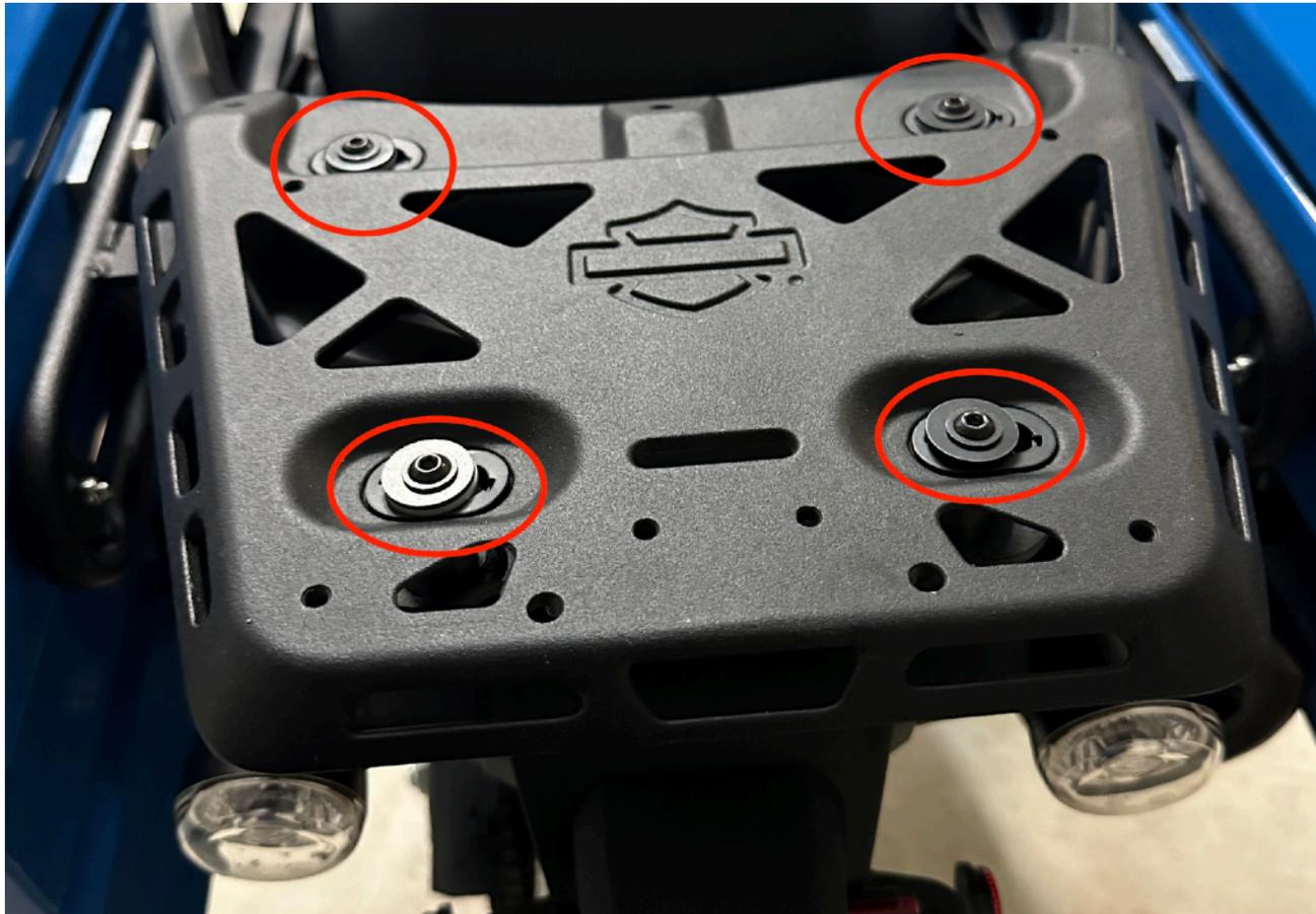
**Step 1** Remove the 4 OEM fasteners from the top case mount.
