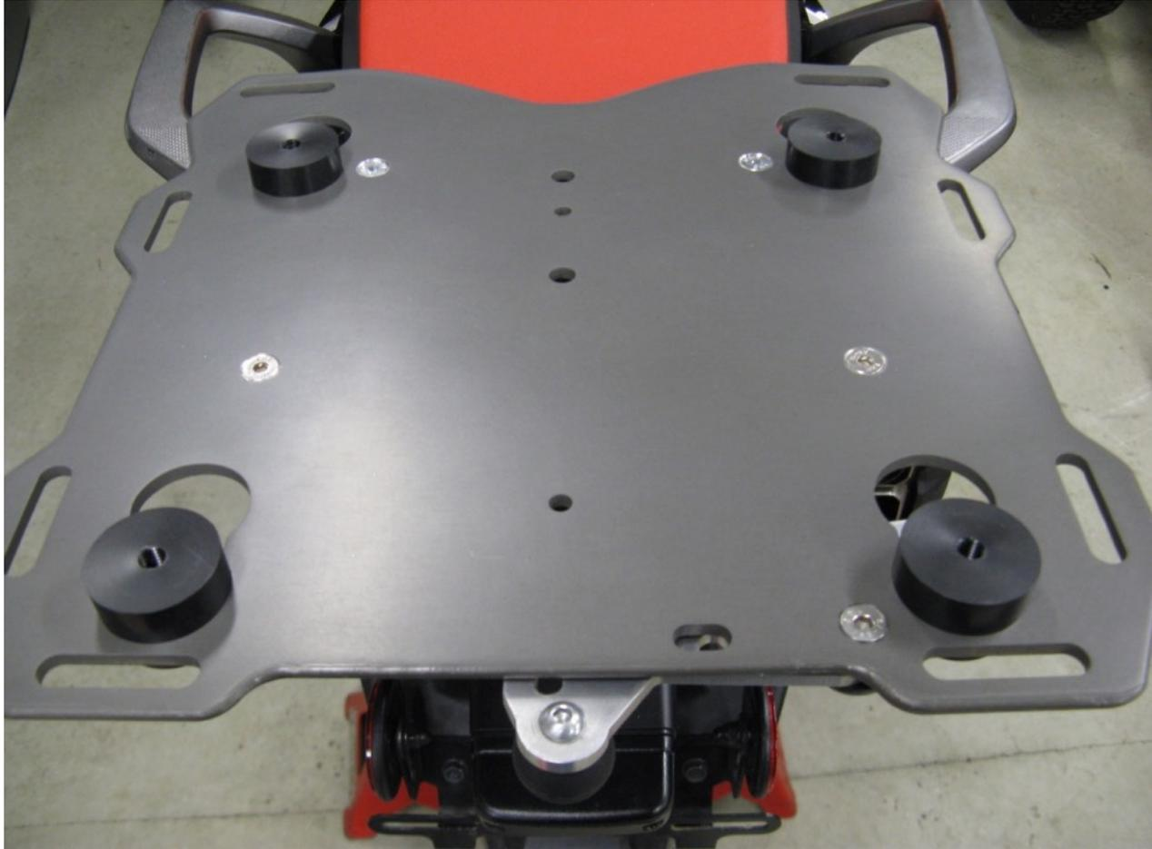
**Step 8** Insert the 3 remaining pucks into the keyholes in the plate.
