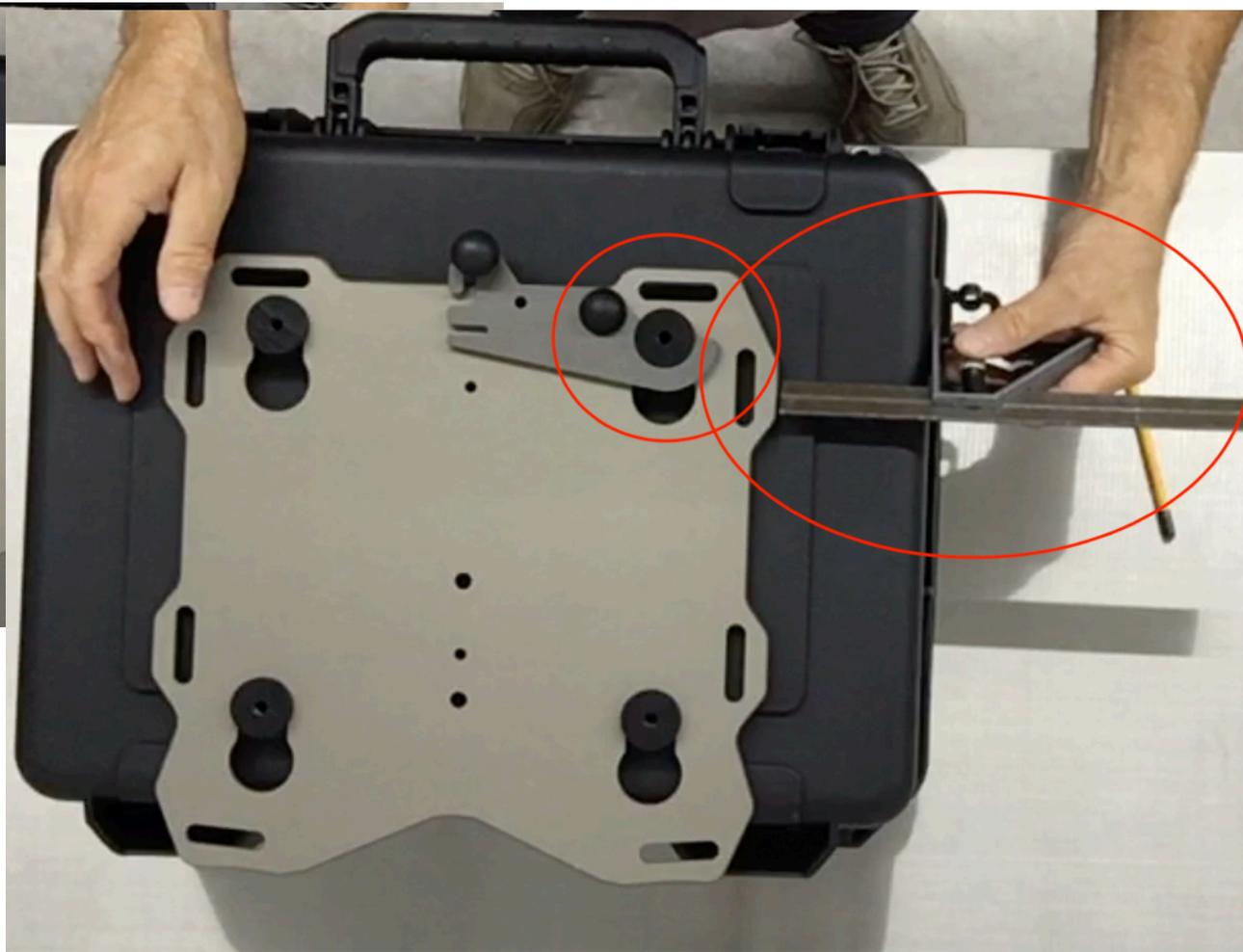
**Step 11** Locate the puck mark on the case and align the master puck with the mark as it was on the bike. Adjust the box side to side and make any final adjustments to the location.
