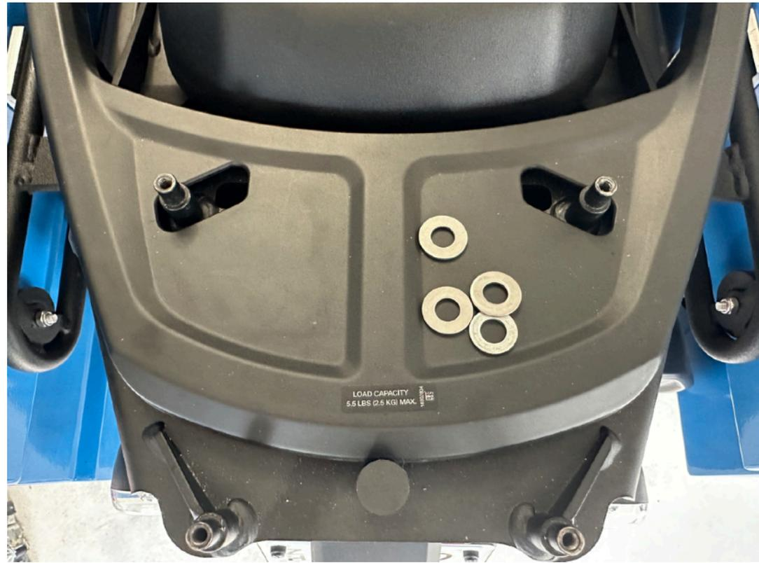
**Step 2** Remove the top plate and hardware, only the silver colored steel washers will be reused.
