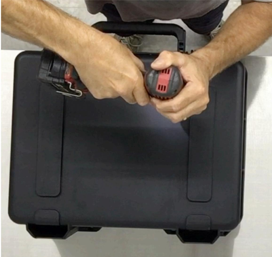
**Step 13** Remove the Slider plate from the case. Use the  $\frac{21}{64}$ " drill bit and electric drill to enlarge the  $\frac{1}{4}$ " pilot hole.
