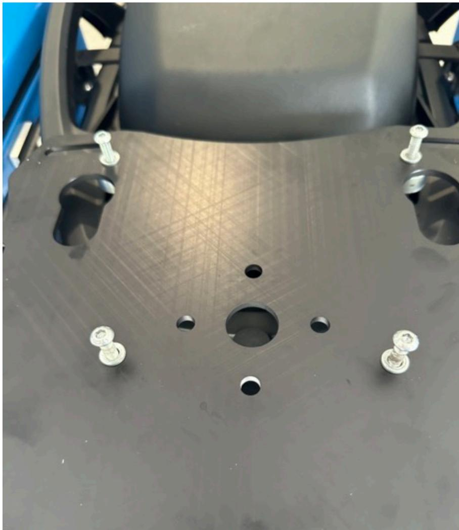
**Step 5** Place the BRE Slider plate on top of the bosses, install the M6 flat washers and M6 x 22 button head screws. Hand thread each of the screw a few turns.
