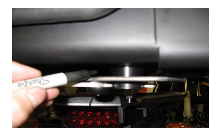
**Step 12** Position the box on top of the pucks. Determine the for/aft location (side to side will be determined later). Position the box as far forward as possible without interfering with passenger comfort. Also consider if you will be placing any gear on the seat or if you want to be able to remove the seat with the box in place. Use a marker to mark the master puck location on the box.
