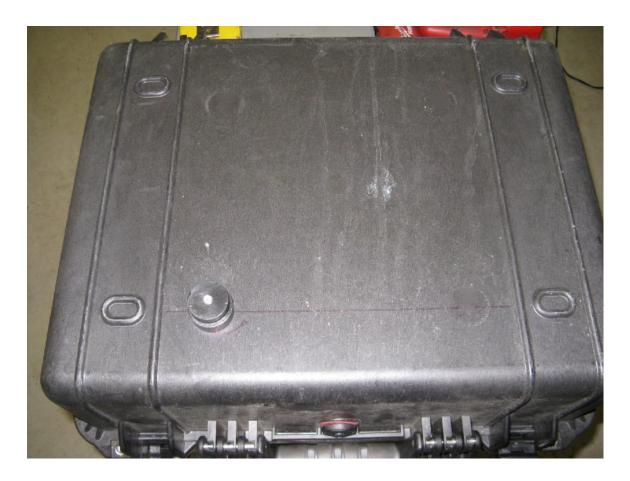
**Step 18** Use the 5/16" button head cap screw and  $1\frac{1}{2}$ " aluminum washer to attach the master puck to the box.
