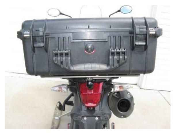
**Step 24** Install the box onto rack and latch it into place with the cam lever.
