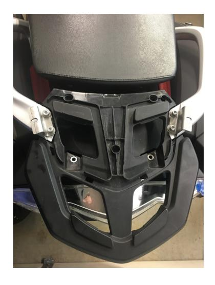
**Step 4** Install the LH and RH front "Z" brackets as shown using 4 M6 x 25mm SHCS and 4 M6 flat washers. **Note:** The top of the brackets angle downwards towards the front of the bike. Do not tighten the screws completely. **Note:** flat washers go on top of "Z" bracket.
