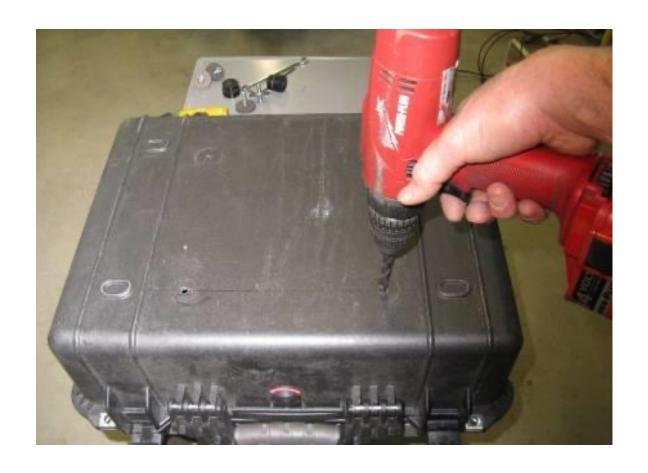
Step 23 Remove the rack and pucks from the box. Use the 21/64" drill bit and electric drill to enlarge the last 2 1/4" pilot holes.
