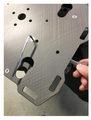
**Step 25** Re-install the plate on the "Z" brackets. Tighten the 4 lock nuts.
