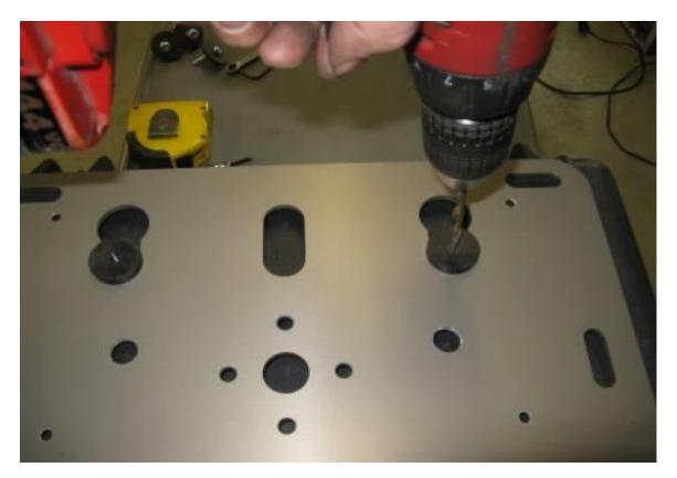
**Step 20** With the ¼" drill bit, use the puck diagonally across from the master puck as a drill guide and drill a second pilot hole in the box.
