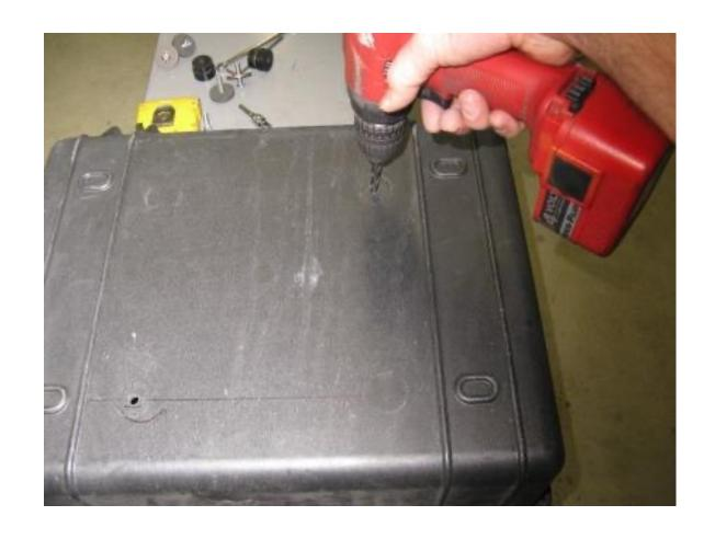
**Step 21** Remove the rack from the box. Use the 21/64" drill bit and electric drill to enlarge the  $\frac{1}{4}$ " pilot hole.
