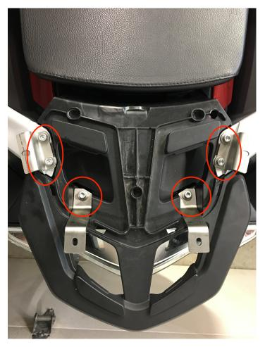
**Step 13** The "Z" brackets are now located and tight (step 9). Remove the 4 nylock nuts (be carefull, use the taped wrench). Remove the plate from the brackets. Torque the six M6 SHCSs to 10 ft. lbs.
