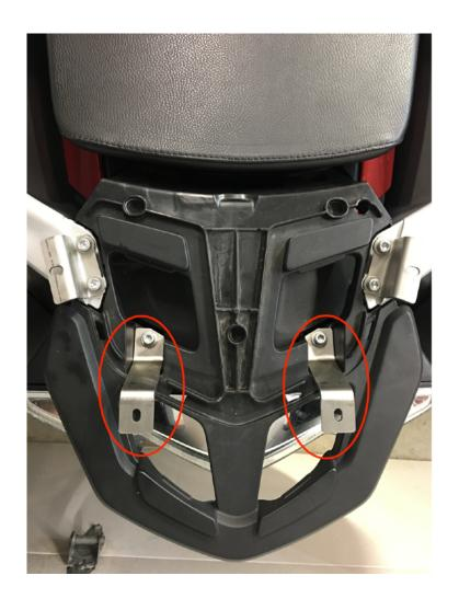
**Step 5** Install the RH and LH rear "Z" brackets as shown using 2 M6 x 40mm SHCS and 2 M6 flat washers. The base of the "Z" bracket is clearance to fit the recess on the bike so there is a RH and LH. Do not tighten the screws completely. **Note:** flat washers go on top of "Z" bracket.
