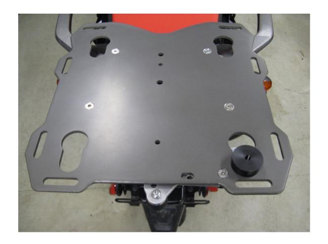
**Step 10** Install one of the black plastic pucks into the key hole with the cam lever. Lock the puck into place with the cam lever. This will be referred to as the "Master Puck"
