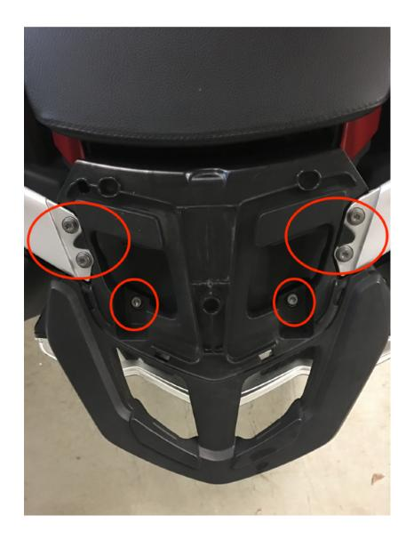
**Step 3** Remove the 4 pillion handle screws and the 2 rear screws circled in red. *These screws will not be used with the Slider rack, save these if you ever plan on removing the Slider rack.*
