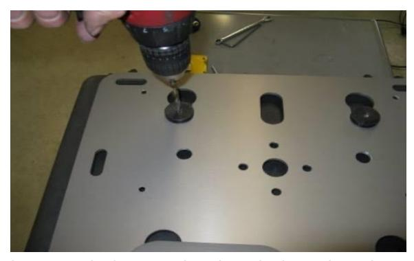
**Step 22** Bolt the second puck to the box. Place the rack on the box and latch it into position. With the ¼" drill bit use the 2 remaining pucks as drill guides and drill the last 2 pilot holes.
