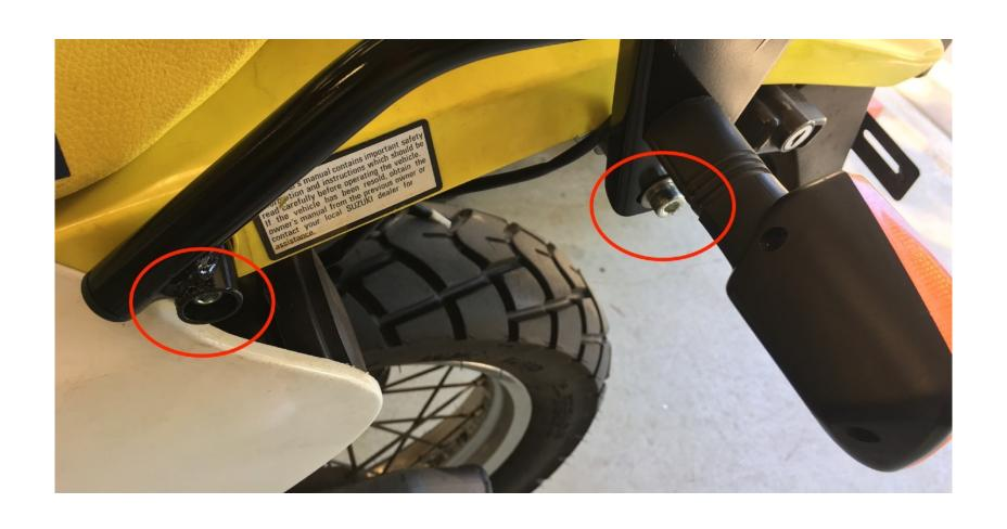
**Step 11** Torque the LH BRE tube screws to 18ft.lb.
