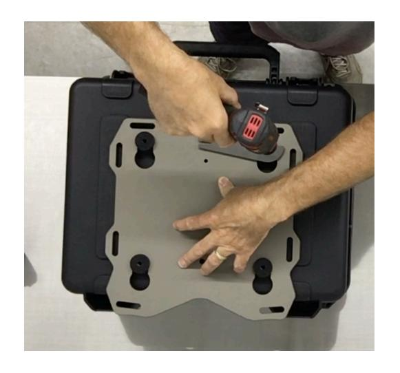
**Step 18** With one hand apply downward force on the Slider plate, use your other hand to drill the case. With a  $\frac{1}{4}$ " drill bit and electric drill use the master puck as a drill guide and drill a pilot hole through the case.
