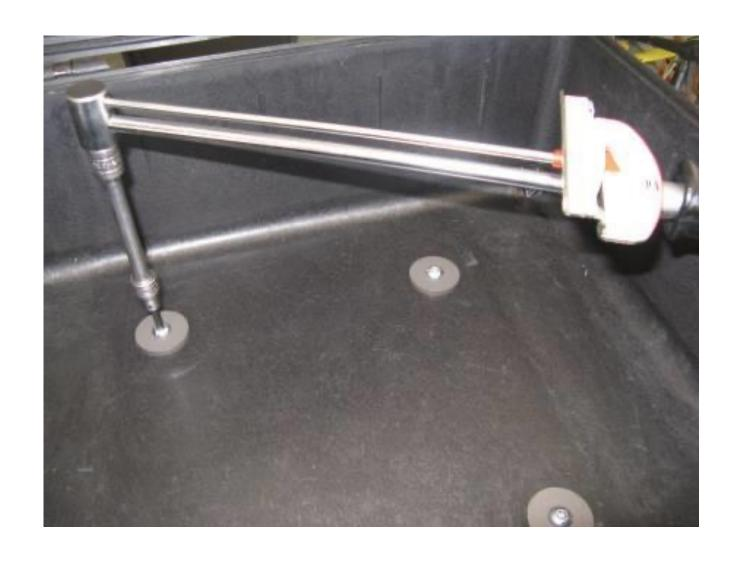
Step 31 Torque the puck screws to 9 ft.lb. or 12.2 Nm.
