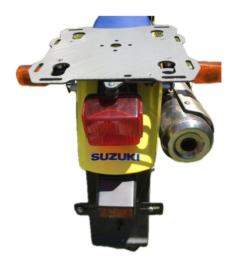
**Step 27** Re-attach the plate using the four M6 x 25 flat head screws and M6 lock nuts. **Torque** the screws to 8ft.lbs.
