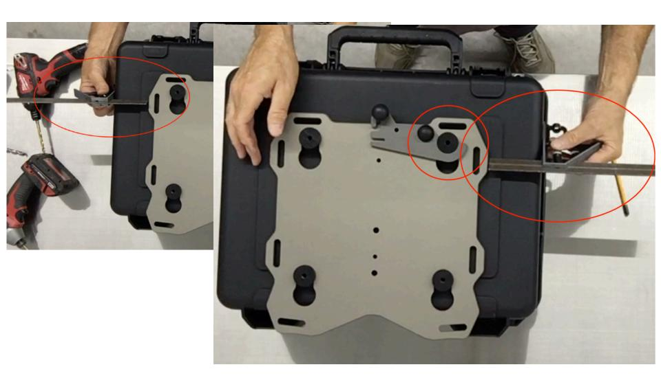
**Step 17** Locate the puck marker on the case and align the master puck with the mark as it was on the bike. Adjust the box side to side and make any final adjustments to the location.
