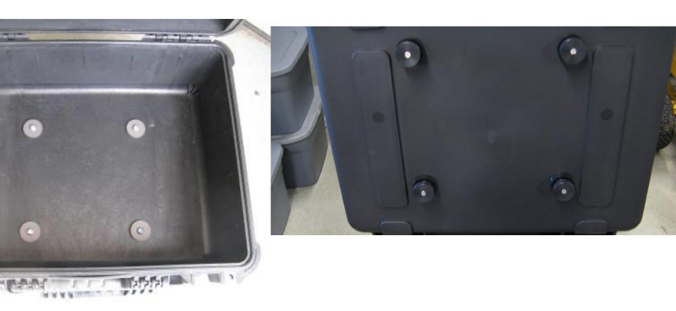
**Step 26** Install all pucks onto the case using the M8 flat washers and M8 button head cap screws. Lightly snug the puck screws at this time, later they will be fully tightened.
