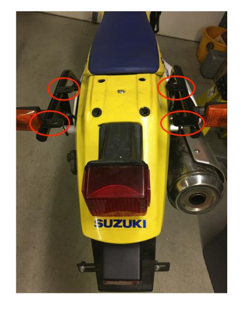
**Step 9** Locate the four 19mm OD x 11mm tall aluminum spacers and install on top of the four tabs.
