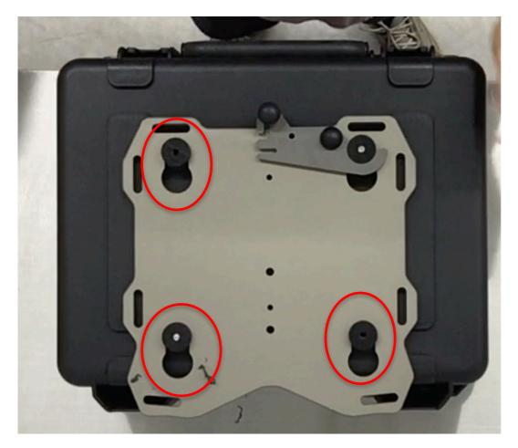
**Step 24** Attach the second puck to the case with the M8 hardware. Place the Slider rack on the case and latch it into position. With the 1/4" drill bit use the 2 remaining pucks as drill guides and drill the last two 1/4" holes.
