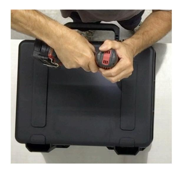
**Step 19** Remove the Slider plate from the case. Use the 21/64" drill bit and electric drill to enlarge the ¼" pilot hole.
