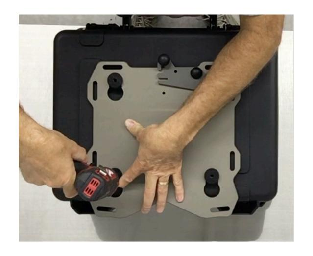
**Step 22** With the ¼" drill bit, use the puck diagonally across from the master puck as a drill guide and drill a second pilot hole in the case.
