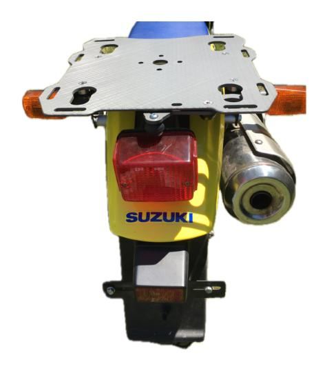
**Step 10** Attach the plate using the four M6 x 25 flat head screws and M6 lock nuts. **Torque** the screws to 8ft. lbs.
