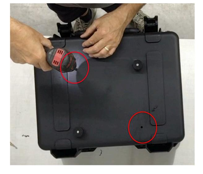
**Step 25** Remove the Slider rack and pucks from the case. Use the 21/64" drill bit and electric drill to enlarge the last two  $\frac{1}{4}$ " pilot holes.
