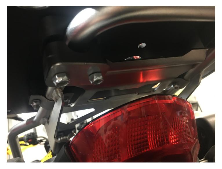
**Step 5** Install the nylon bottom clamp halves, stainless steel plates and M6 lock nuts on the rear clamp screws as shown in the photo. Install both LH and RH sides.
