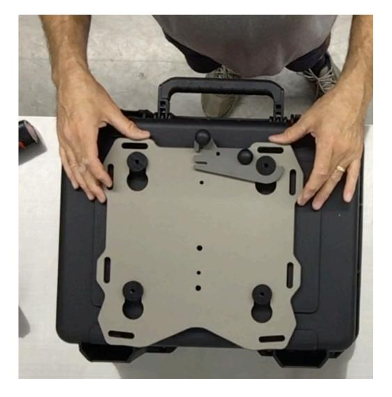
**Step 10** Place the case on a table or other work surface. Remove the 4 flat head screws holding the Slider plate onto the motorcycle. Place the Slider plate with the pucks installed onto the case.
