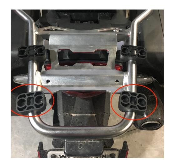
**Step 1** Place the top of the clamp halves in the locations shown in the photo. **Note:** The narrow clamp halves must be located at the rear of the grab handle.
