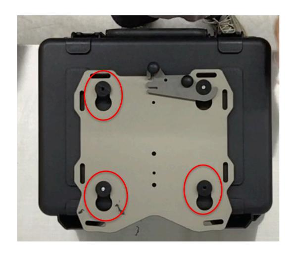
**Step 18** Attach the second puck to the case with the M8 hardware. Place the Slider rack on the case and latch it into position. With the  $\frac{1}{4}$ " drill bit use the 2 remaining pucks as drill guides and drill the last two  $\frac{1}{4}$ " holes.
