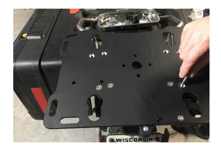
**Step 2** Place the Slider Plate on top of the clamp halves and insert the four M6 x 60 flat head screws through the plate and clamp halves in the rear.
