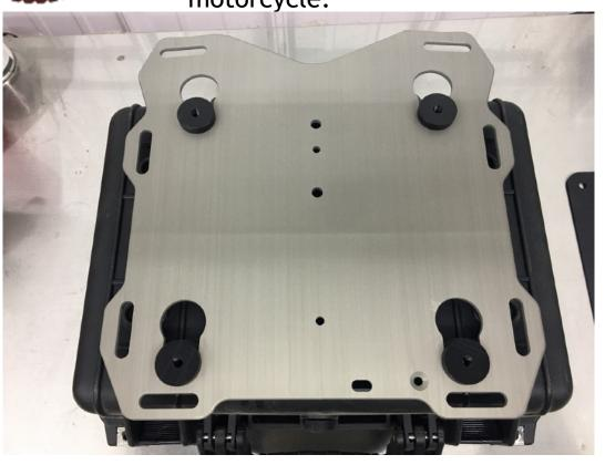
**Step 2** locate the RH and LH pucks and insert them into the Slider plate in the correct location, see Note on page 1.
