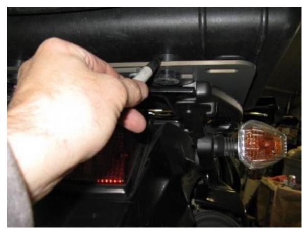
**Step 9** Mark the location of the master puck onto the top box with a marker.
