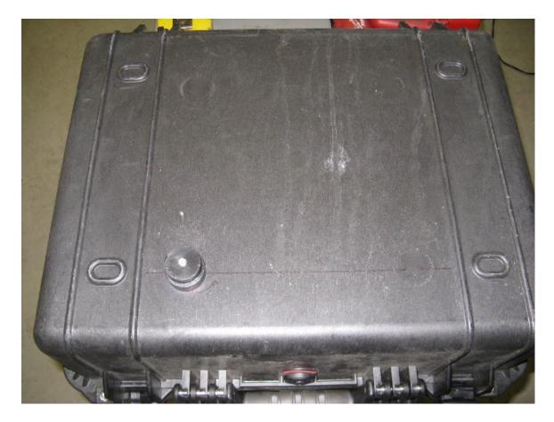
**Step 14** Use a 8mm button head cap screw and 38mm OD aluminum washer to attach the master puck to the box.
