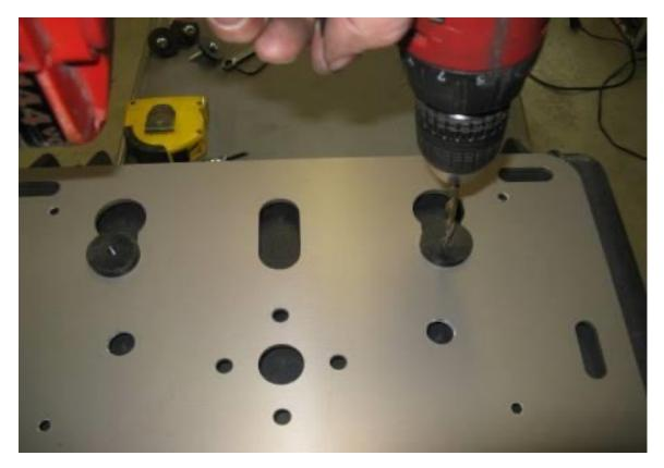
**Step 16** With the ¼" drill bit, use the puck diagonally across from the master puck as a drill guide and drill a second pilot hole in the box.
