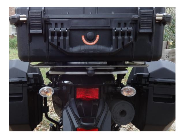
**Step 22** Install the box onto rack and latch it into place with the cam lever.
