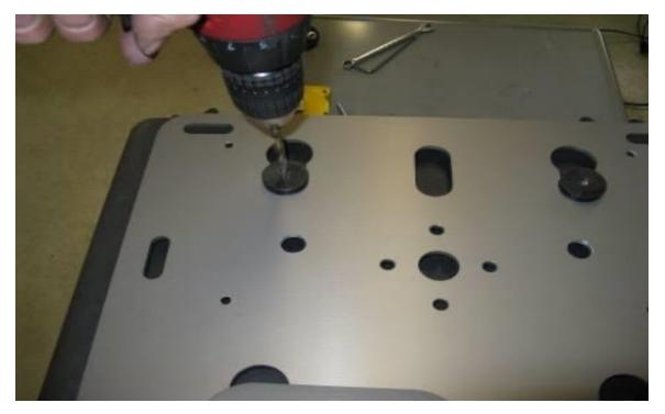
**Step 18** Bolt the second puck to the box. Place the rack on the box and latch it into position. With the 1/4" drill bit use the 2 remaining pucks as drill guides and drill the last 2 pilot holes.
