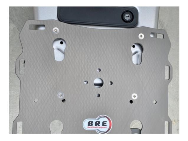
**Step 21** Apply Blue 242 Loctite to the 4 flat head screws and attach the the rack with the screws. Torque the fasteners to 216 inch pounds. This completes the rack installation.
