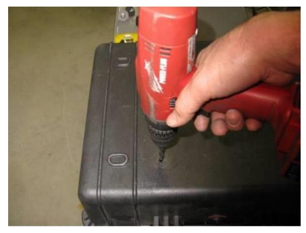
**Step 13** Remove the rack from the box. Use the 21/64" drill bit and electric drill to enlarge the <sup>1</sup>/<sub>4</sub>" pilot hole.
