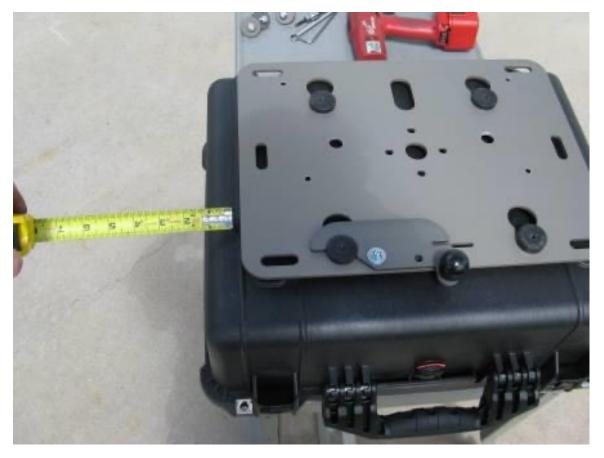
**Step 11** Locate the puck marker on the box and align the master puck up with the mark as it was on the bike.
