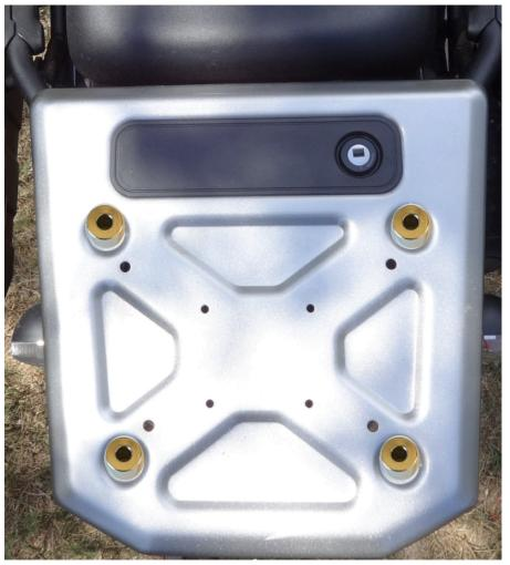
**Step 4** Install the aluminum spacers where the 6mm threaded holes are located.
