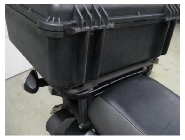
**Step 8** Place the top box on top of the pucks and position it where you would like it located.
