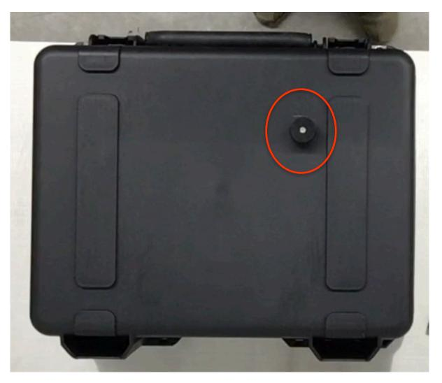
**Step 13** Use a M8 x 38 flat washer and the M8 button head cap screw to attach the master puck to the case.
