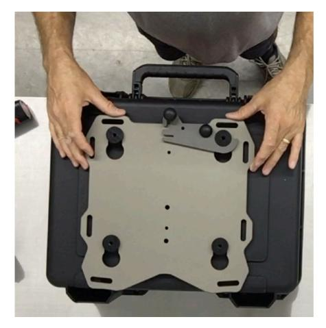
**Step 9** Place the case on a table or other work surface. Remove the 4 flat head screws holding the Slider plate onto the motorcycle. Place the Slider plate with the pucks installed onto the case.
