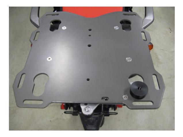
**Step 6** Install one of the black plastic pucks into the key hole with the cam lever. Lock the puck into place with the cam lever. This will be referred to as the "Master Puck" Note: Remove the large washer and screw from the puck before putting into the plate. The screws and washers are installed into the pucks for shipment as part of our QA process.
