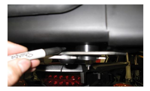
**Step 8** Position the case on top of the pucks. Determine the for/aft location (side to side will be determined later). Position the box as far forward as possible without interfering with passenger comfort. Also consider if you will be placing any gear on the seat or if you want to be able to remove the seat with the box in place. Use a marker to mark the master puck location on the box.
