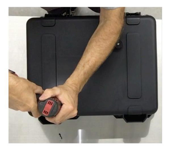
**Step 16** Remove the slider plate from the case and use the 121/64" drill bit to enlarge the second 1/4" pilot hole.
