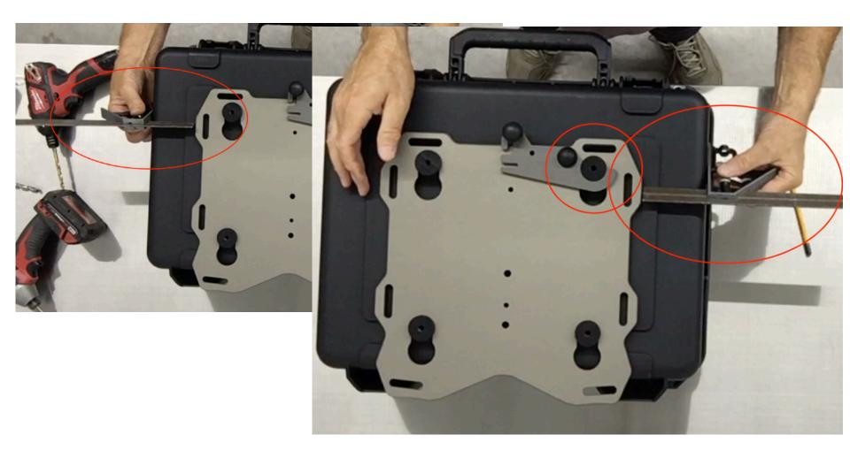
**Step 10** Locate the puck mark on the case and align the master puck with the mark as it was on the bike. Adjust the box side to side and make any final adjustments to the location.
