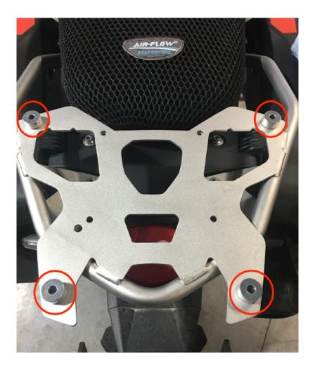
**Step 2** Install the 4 aluminum spacers where the outer screws were.
