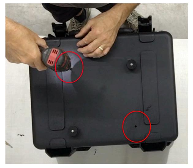
**Step 18** Remove the Slider rack and pucks from the case. Use the 21/64" drill bit and electric drill to enlarge the last 2 1⁄4" pilot holes.
