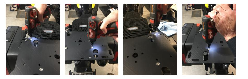
Step 3 Install the BRE plate over the spacers.
