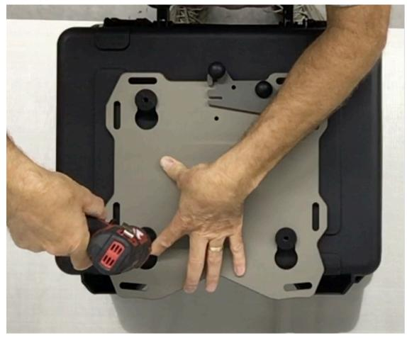
**Step 15** With the ¼" drill bit, use the puck diagonally across from the master puck as a drill guide and drill a second pilot hole in the case.
