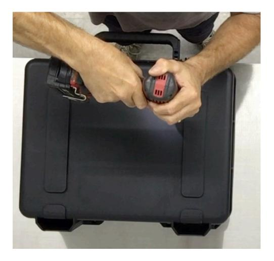
Step 12 Remove the Slider plate from the case. Use the 21/64" drill bit and electric drill to enlarge the  $\frac{1}{4}$ " pilot hole.
