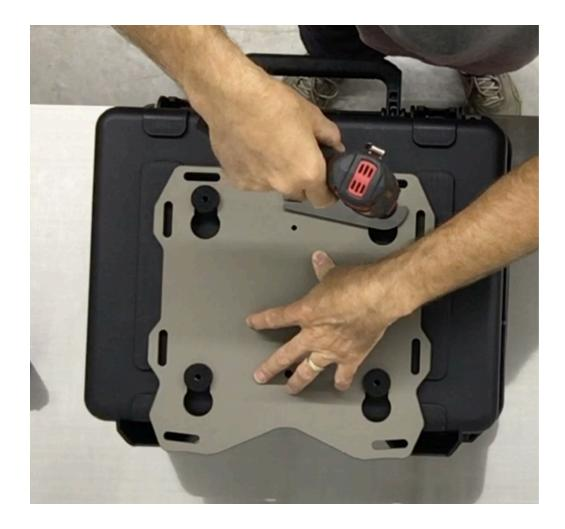
**Step 11** With one hand apply downward force on the Slider plate, use your other hand to drill the case. With a ¼" drill bit and electric drill use the master puck as a drill guide and drill a pilot hole through the box.
