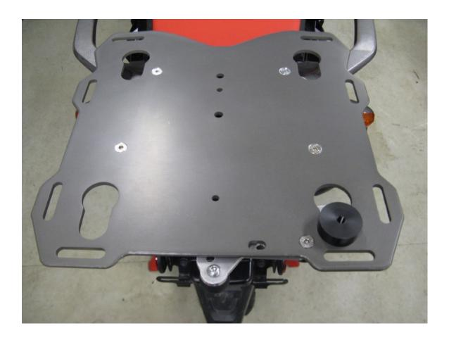
**Step 10** Install one of the black plastic pucks into the key hole with the cam lever. Lock the puck into place with the cam lever. This will be referred to as the "Master Puck" Note: Remove the large washer and screw from the puck before putting into the plate. The screws and washers are installed into the pucks for shipment as part of our QA process.
