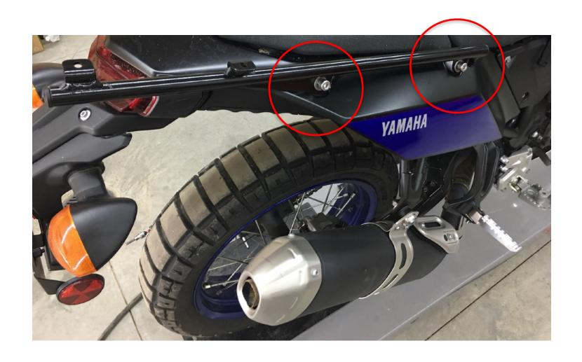
**Step 5** Insert the two spacers and and attach the RH tube with two M8 flat washers and two M8 x 50 SHCSs. DO NOT tighten at this time.
