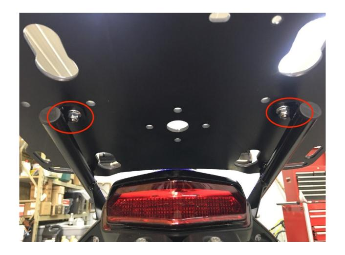
**Step 8** Thread the four M6 flange head lock nuts onto the four M6 x 18 flat head screws. Using a 10 mm open end or combination wrench and 4 mm hex driver tighten the flange nuts completely. NOTE only rear screws are visible in photo.
