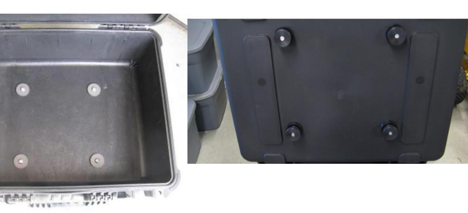
**Step 23** Install all pucks onto the case using the M8 flat washers and M8 button head cap screws. Lightly snug the puck screws at this time, later they will be fully tightened.
