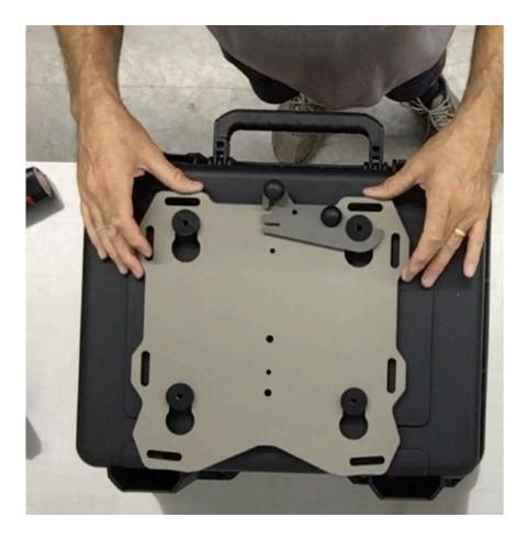
**Step 13** Place the case on a table or other work surface. Remove the 4 flat head screws and nuts holding the Slider plate onto the mounting tubes. Place the Slider plate with the pucks installed on the case.
