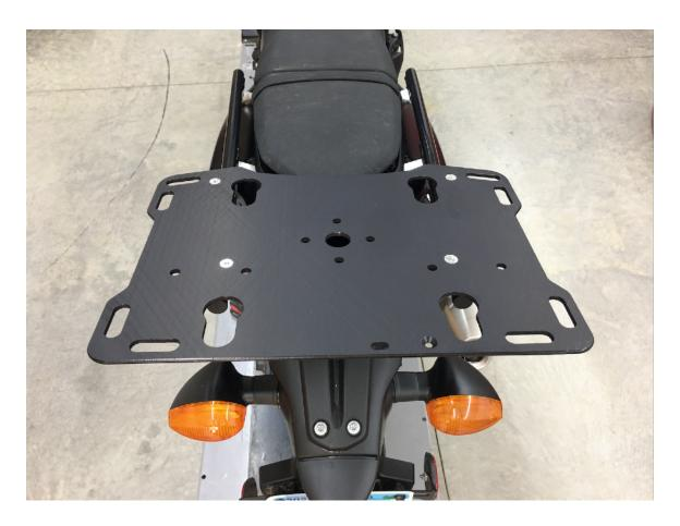
**Step 7** Adjust the plate so it is square to the bike, the next step is to tighten the screws.
