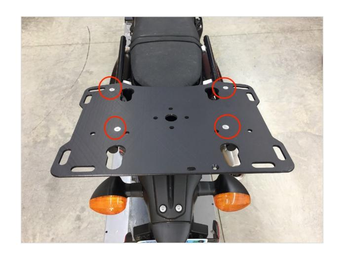
**Step 24** Re-install the plate onto the bike using the M6 flat head screws and lock nuts.
