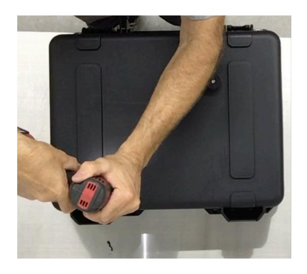
**Step 20** Remove the slider plate from the case and use the 121/64" drill bit to enlarge the second 1/4" pilot hole.
