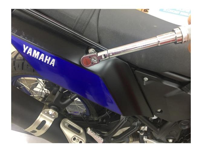
**Step 9** Use a torque wrench and 6mm hex bit and torque the four M8 x 50 SHCSs to 18 ftlb or 24.4 Nm.
