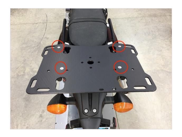
**Step 6** Place the plate on top of the tubes and line up the mounting holes. Insert the 4 M6 x 18 flat head screws in the mounting holes shown.
