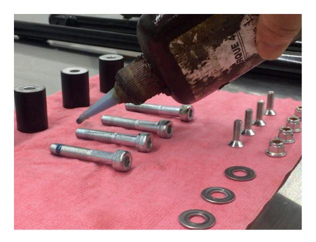
**Step 3** Apply Blue 242 Loctite or equivalent to the threads of the four M8 x 50 SHCSs.
