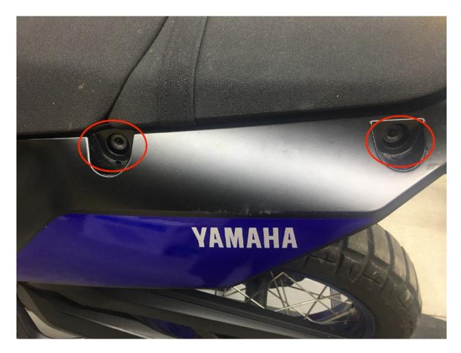
**Step 1** Using the T40 driver remove the 2 OEM tie downs on the RH side and LH side of the bike (4 total).
