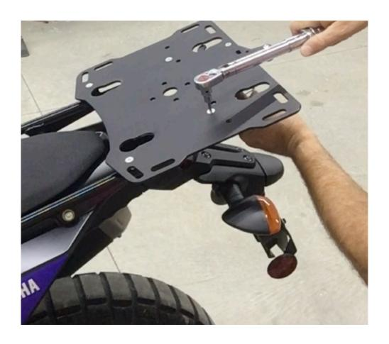
**Step 25** Use a torque wrench, 4mm hex bit and open end wrench and torque the four M6 x18 FHCSs to 8 ftlb or 10.8 Nm.
