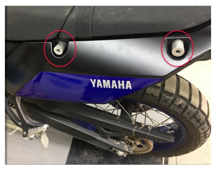
**Step 2** On the LH side of the bike insert the BRE supplied spacers into the openings on the cowling. NOTE: make sure the spacers go through the holes in the plastic cowling.
