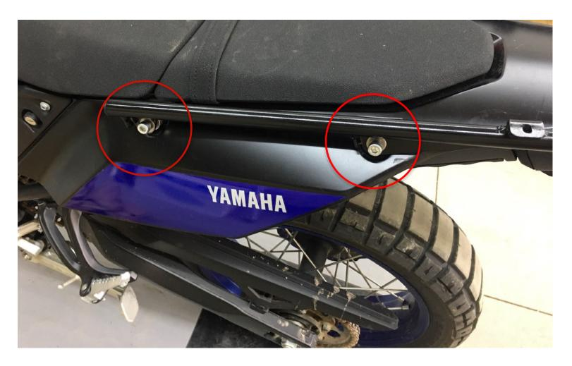
**Step 4** Using the two M8 flat washers and two M8  $\times$  50 SHCS attach the LH tube. Snug the bolts, DO NOT tighten at this time.
