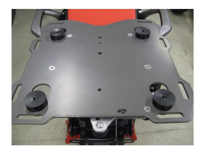
**Step 9** Insert the 3 remaining pucks into the keyholes in the plate.
