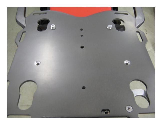
**Step 21** Re-install the plate on the spacers. Re-install the M6 flat head screws and tighten the clamps.
