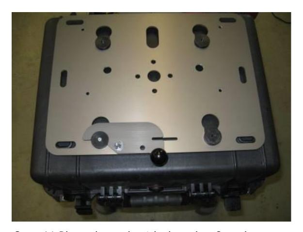
**Step 16** Place the rack with the other 3 pucks onto the master puck and latch it into position. Square up the plate and box to each other (last chance).
