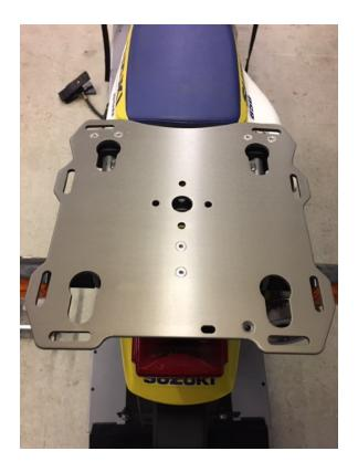
**Step 3** Place the BRE plate on top of the spacers and insert the four 60mm screws in the front clamps and the 50 mm screws in the rear clamp.
