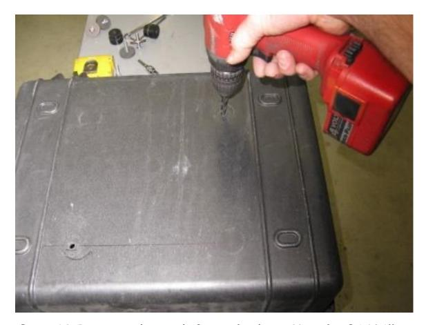
**Step 18** Remove the rack from the box. Use the 21/64" drill bit and electric drill to enlarge the ¼" pilot hole.
