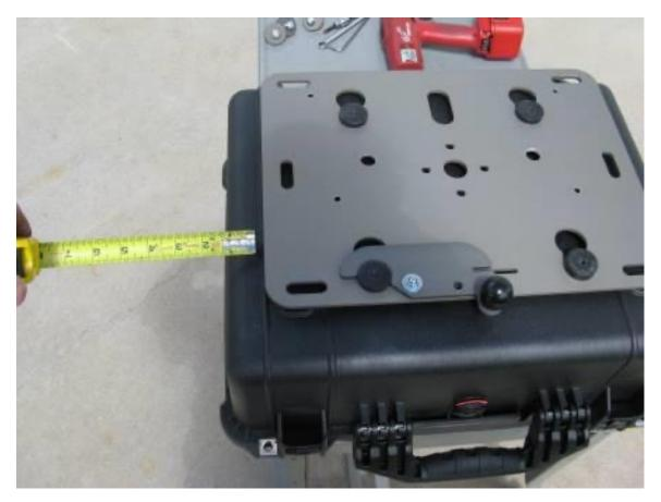
**Step 12** Locate the puck marker on the box and align the master puck up with the mark as it was on the bike.
