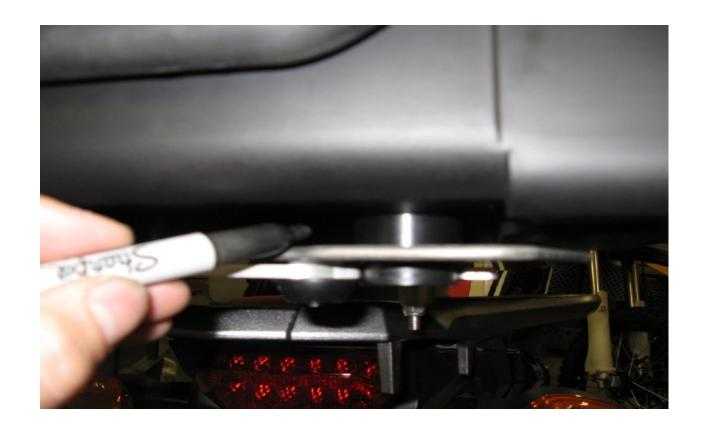
**Step 10** Position the box on top of the pucks. Determine the for/aft location (side to side will be determined later). Position the box as far forward as possible without interfering with passenger comfort. Also consider if you will be placing any gear on the seat or if you want to be able to remove the seat with the box in place. Use a marker to mark the master puck location on the box.
