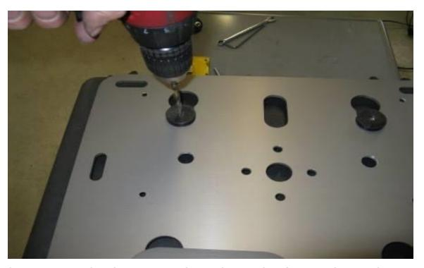
**Step 19** Bolt the second puck to the box. Place the rack on the box and latch it into position. With the ¼" drill bit use the 2 remaining pucks as drill guides and drill the last 2 pilot holes.
