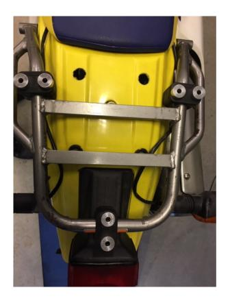
**Step 2** Place the low profile clamp on the rear tube of the OEM rack and the other 2 clamps on the side tubes as shown in the photo. Place 6 aluminum spacers on top of the clamps.
