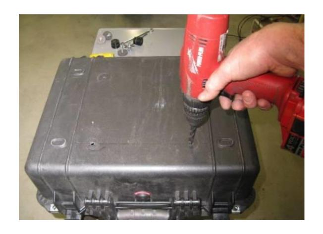
**Step 19** Remove the rack and pucks from the box. Use the 21/64" drill bit and electric drill to enlarge the last 2 1/4" pilot holes.
