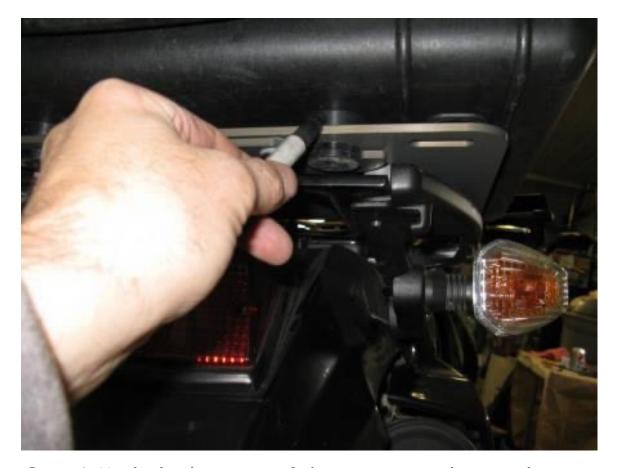
**Step 9** Mark the location of the master puck onto the top box with a marker.
