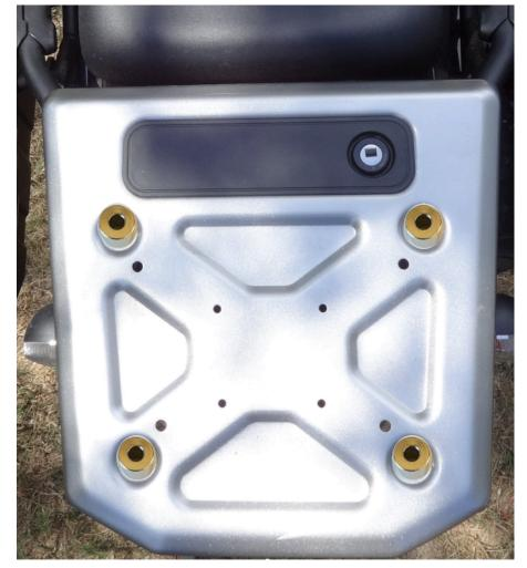
**Step 4** Install the aluminum spacers where the 6mm threaded holes are located.
