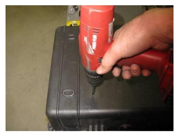
**Step 13** Remove the rack from the box. Use the 21/64" drill bit and electric drill to enlarge the ¼" pilot hole.
