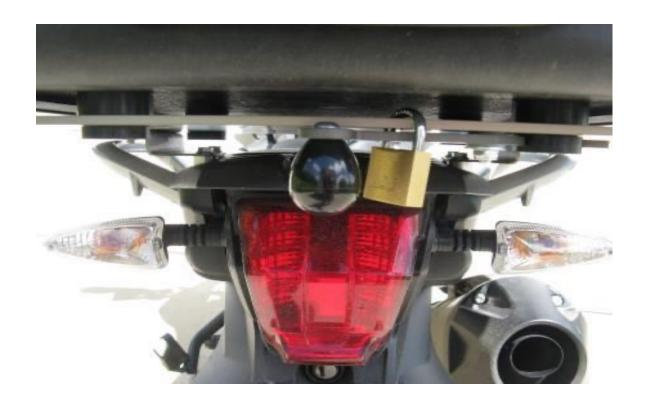
That completes the installation process. Test ride the motorcycle and then check all the fasteners for tightness. Also check the fasteners again after 1000 miles and at every oil change after that.
