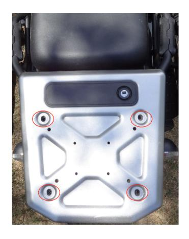
**Step 1** Remove the 4 tail cover screws.
