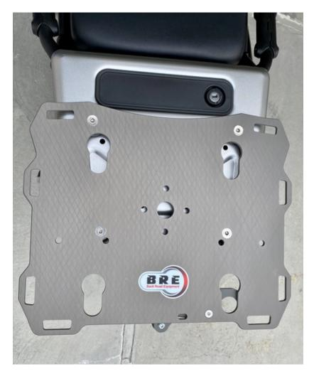
**Step 6** Attach the rack to the motorcycle with the 4 flat head screws as shown. Just snug the screws for now as you will be removing them in a later step.
