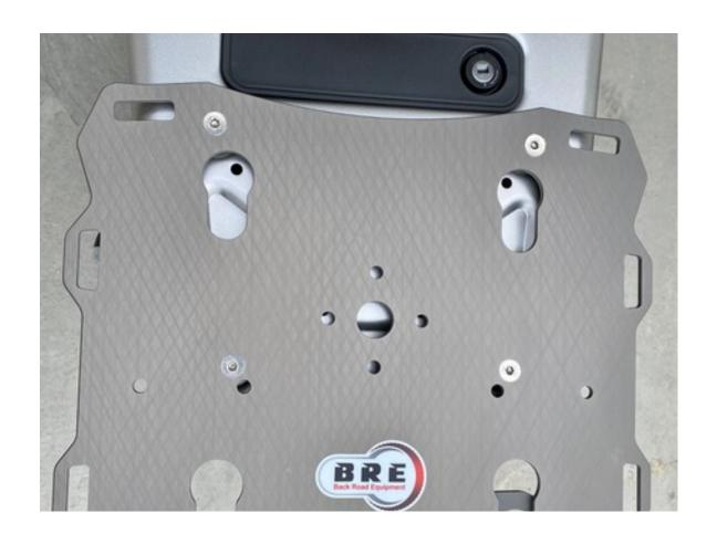
**Step 21** Apply Blue 242 Loctite to the 4 flat head screws and attach the rack with the screws. Torque the fasteners to 216 inch pounds. This completes the rack installation.
