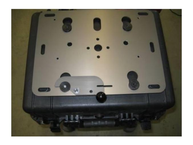
Step 17 Place the rack with the other 3 pucks onto the master puck and latch it into position. Square up the plate and box to each other (last chance).
