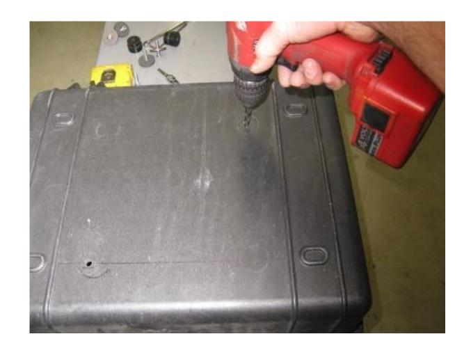
Step 19 Remove the rack from the box. Use the 21/64" drill bit and electric drill to enlarge the 1/4" pilot hole
