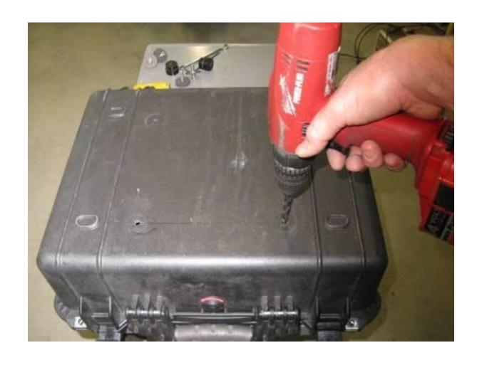
Step 21 Remove the rack and pucks from the box. Use the 21/64" drill bit and electric drill to enlarge the last 2 1/4" pilot holes.
