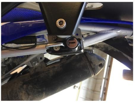
**Step 7** Attach the left hand BRE tube with the M8 x 70 screw. The screw will pass through the tube bracket, the large diameter spacer, the small diameter spacer and the helmet lock relocation bracket. Hand tighten the screw at this time. **Note:** Installing the OEM helmet lock is optional.
