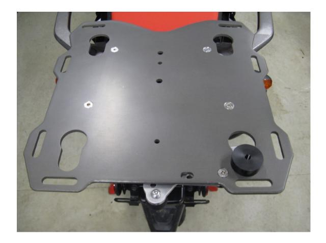
**Step 14** Install one of the black plastic pucks into the key hole with the cam lever. Lock the puck into place with the cam lever. This will be referred to as the "Master Puck"
