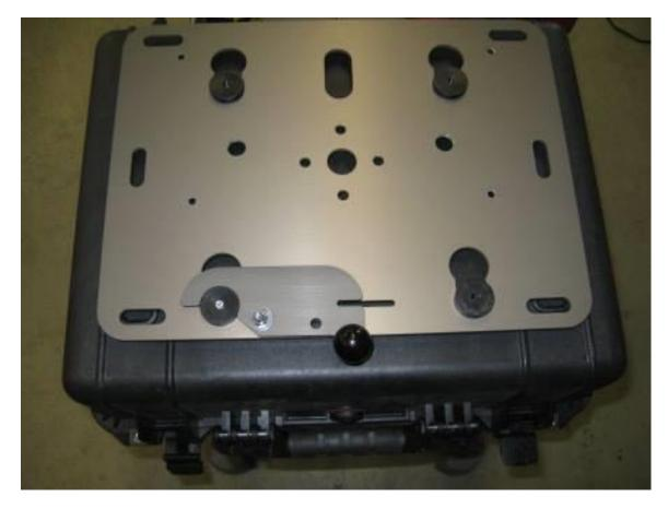
**Step 22** Place the rack with the other 3 pucks onto the master puck and latch it into position. Square up the plate and box to each other (last chance).
