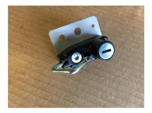
**Step 6** Remove the helmet lock from the motorcycle and attach to the lock relocation bracket with the OEM screw and a BRE supplied M6 lock nut. **Note:** Installing the OEM helmet lock is optional.
