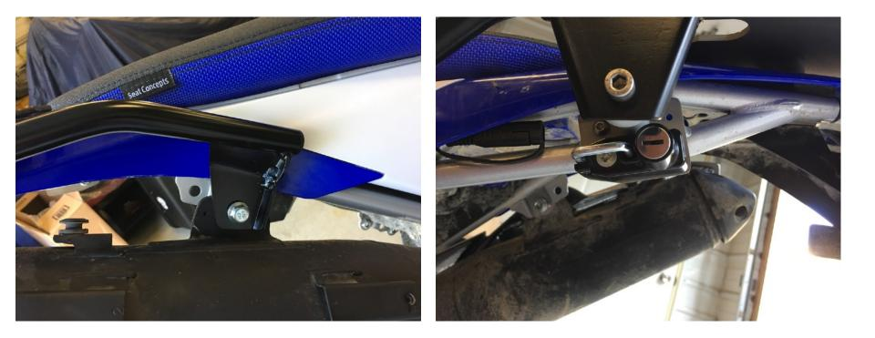
**Step 11** Snug the M8 and M10 tube mounting bolts so their is no clearance between the mounting brackets and the subframe but do not apply final torque.
