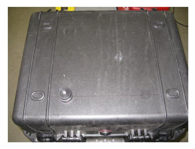
Step 21 Use the 5/16" button head cap screw and 1  $\frac{1}{2}$ " aluminum washer to attach the master puck to the case.
