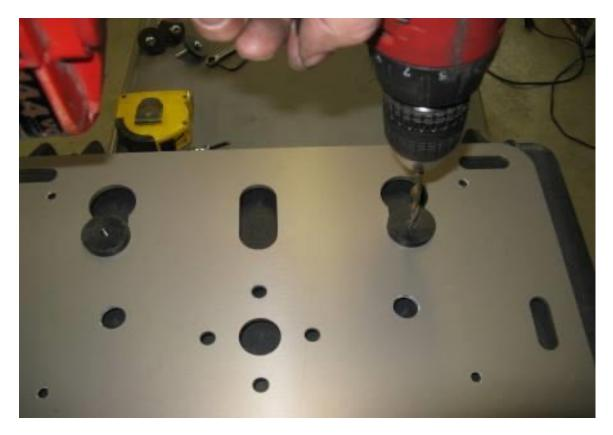
**Step 23** With the <sup>1</sup>/<sub>4</sub>" drill bit, use the puck diagonally across from the master puck as a drill guide and drill a second pilot hole in the box.
