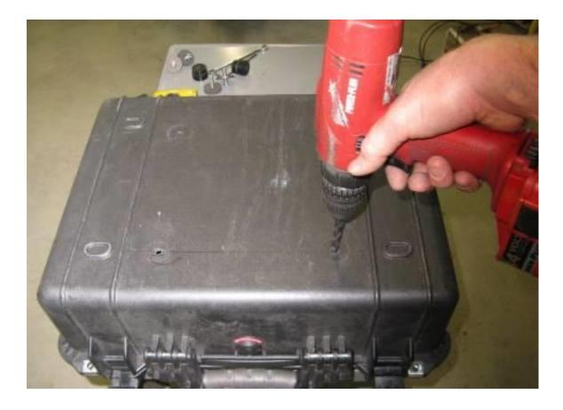
Step 26 Remove the rack and pucks from the box. Use the 21/64" drill bit and electric drill to enlarge the last 2  $\frac{1}{4}$ " pilot holes.
