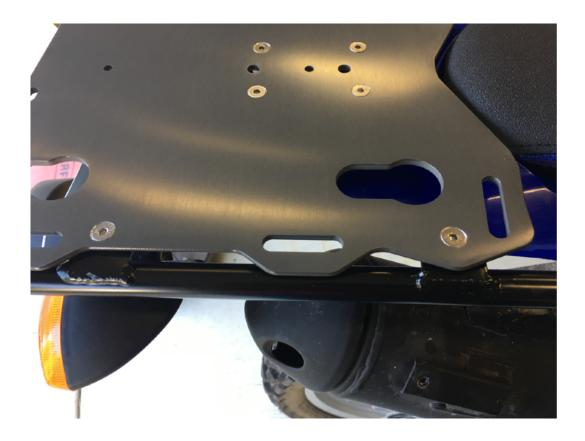
**Step 10** Insert two M6 x 18 flat head screws into the plate and through the mounting tabs on the right hand BRE tube. Install M6 washers and locking nuts do not tighten nuts at this time.
