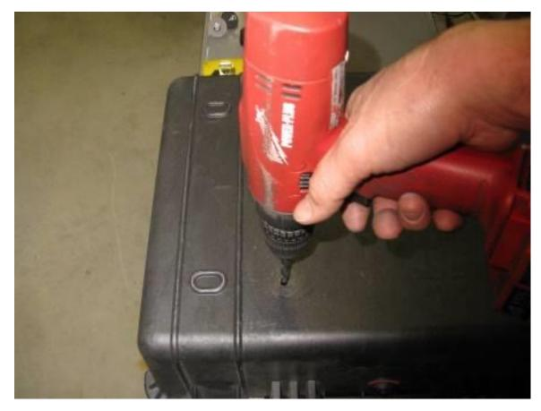
**Step 20** Remove the rack from the box. Use the 21/64" drill bit and electric drill to enlarge the <sup>1</sup>/<sub>4</sub>" pilot hole
