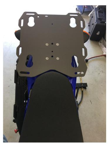
**Step 5** Install the slider plate with the four 60mm flat head screws. Install flat washers and lock nuts on the bottom of the front screws and thread the rear screws into the subframe. Tighten all screws with a 4mm hex driver. A 10 mm wrench or socket will be needed to hold the lock nuts on the front screws.
