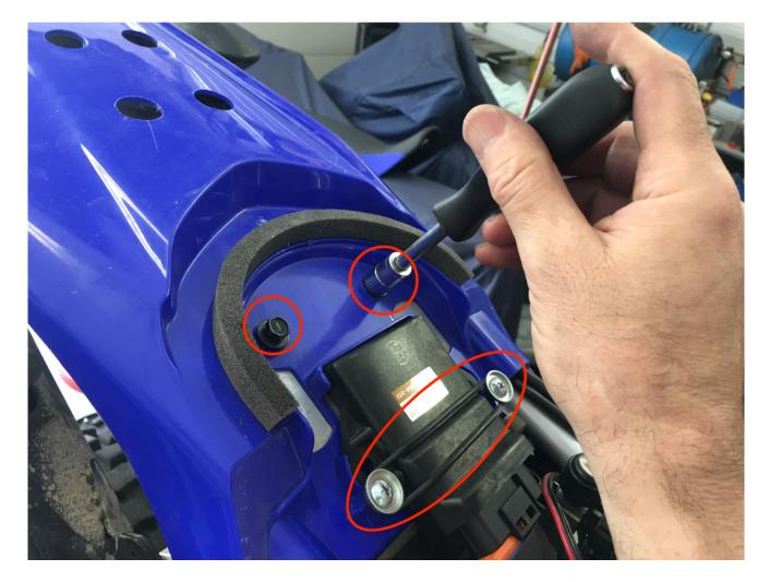
**Step 2** Remove the 2 bolts that retain the fender and remove the rubber o-ring that retains the ECU.
