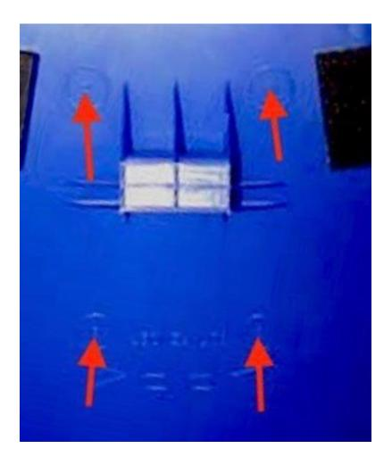
**Step 3** Remove the rear fender and turn upside down. Locate the 4 circular rack mounting markers. Use an 1/8" drill bit to drill the center of each circle. Enlarge the holes with a step drill to 3/4".
