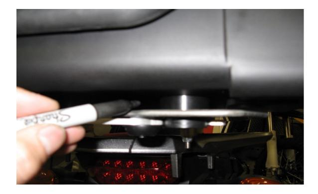
**Step 16** Position the box on top of the pucks. Determine the fore/aft location (side to side will be determined later). Position the box as far forward as possible without interfering with passenger comfort. Also consider if you will be placing any gear on the seat or if you want to be able to remove the seat with the box in place. Use a marker to mark the master puck location on the box.
