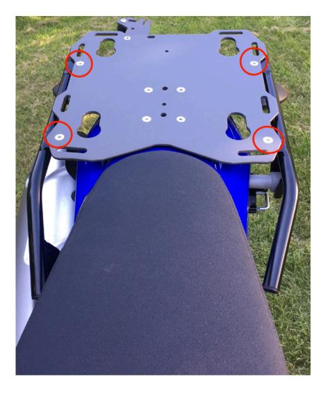
**Step 12** Tighten all 4 M6 flat head screws with 4mm hex wrench and 10mm socket wrench.
