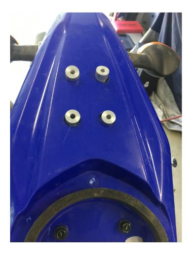
**Step 4** Reinstall the rear fender on the motorcycle and insert the four long 19mm aluminum spacers into the fender holes. Tighten the fender mounting screws and reinstall the ECU o-ring.
