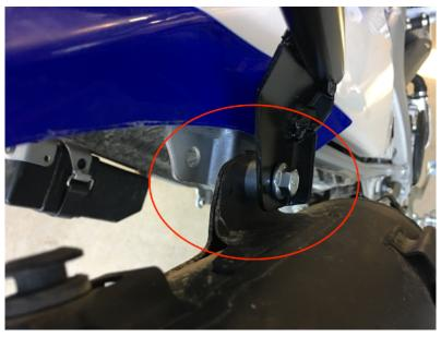
Step 9 Remove the muffler mounting bolt and install BRE right hand tube and 19mm x 12mm aluminum spacer with BRE M10 x 30 muffler mounting bolt, do not completely tighten bolt at this time.
