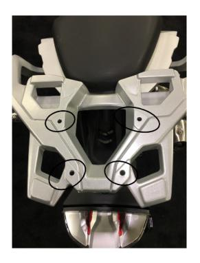
Step 1 Install the slider plate on the rear of the bike by placing the 4 aluminum spacers between the OEM rack and the Slider rack.
