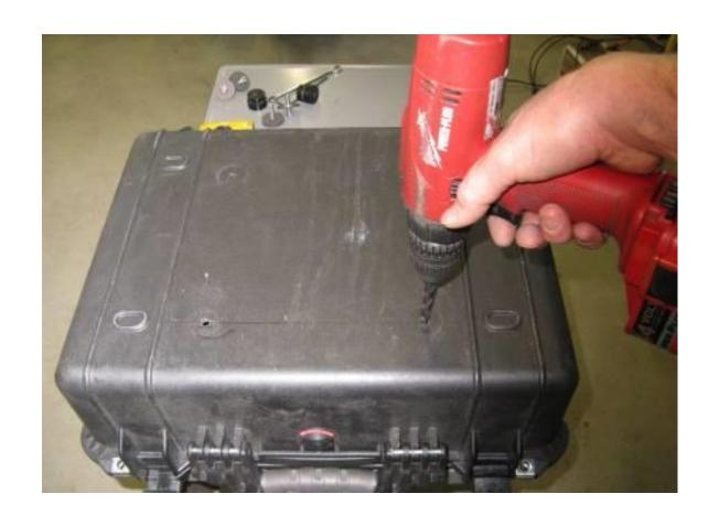
Step 15 Remove the rack and pucks from the box. Use the 21/64" drill bit and electric drill to enlarge the last 2 1/4" pilot holes.
