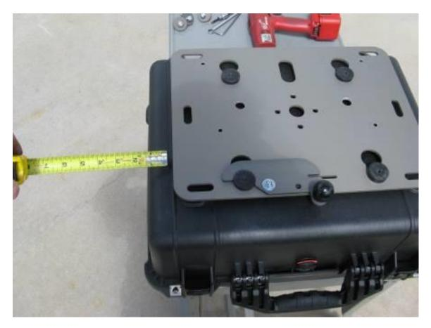
Step 7 Locate the puck marker on the box and align the master puck up with the mark as it was on the bike.
