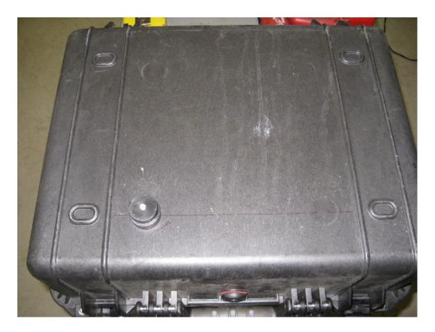
Step 10 Use the 5/16" button head cap screw and 1 ½" aluminum washer to attach the master puck to the box.
