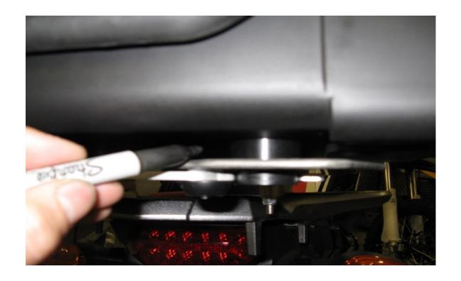
Step 5 Position the box on top of the pucks. Determine the for/aft location (side to side will be determined later). Position the box as far forward as possible without interfering with passenger comfort. Also consider if you will be placing any gear on the seat or if you want to be able to remove the seat with the box in place. Use a marker to mark the master puck location on the box.
