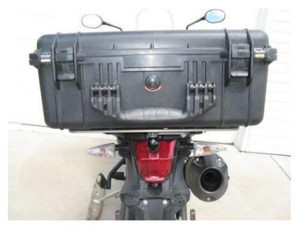
Step 18 Install the box onto rack and latch it into place with the cam lever.
