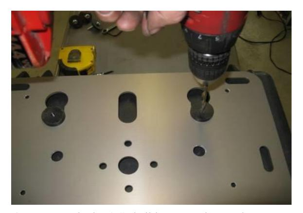
Step 12 With the ¼" drill bit, use the puck diagonally across from the master puck as a drill guide and drill a second pilot hole in the box.
