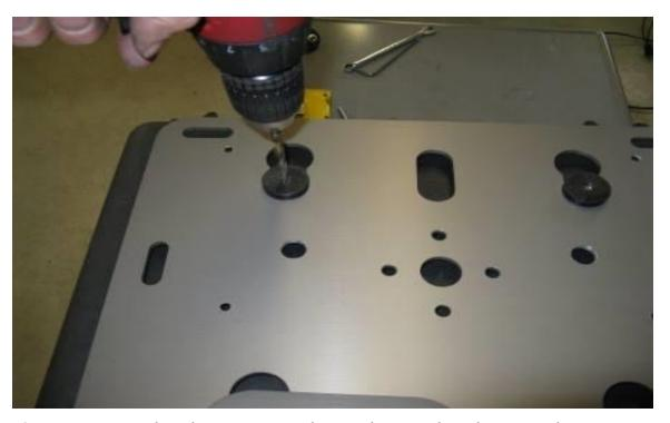
Step 14 Bolt the second puck to the box. Place the rack on the box and latch it into position. With the ¼" drill bit use the 2 remaining pucks as drill guides and drill the last 2 pilot holes.
