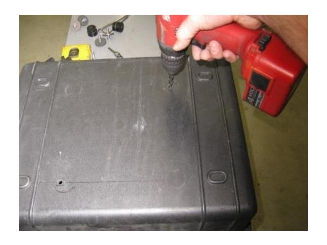
Step 13 Remove the rack and pucks from the box. Use the 21/64" drill bit and electric drill to enlarge the 1/4" pilot hole.
