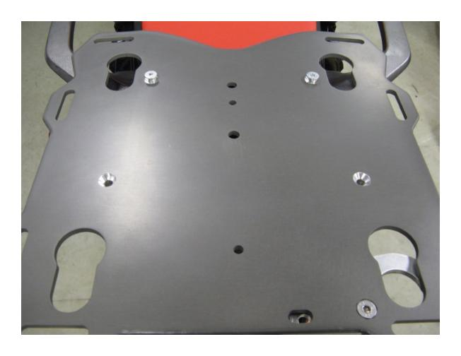
Step 17 Re-install the plate on the spacers. Re-install the M6 flat head screws and M6 lock nuts. Torque to 110 inlbs.
