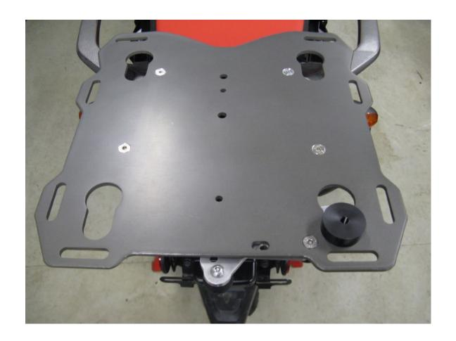
Step 3 Install one of the black plastic pucks into the key hole with the cam lever. Lock the puck into place with the cam lever. This will be referred to as the "Master Puck"
