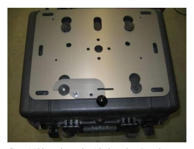
Step 14 Place the rack with the other 3 pucks onto the master puck and latch it into position. Square up the plate and box to each other (last chance).
