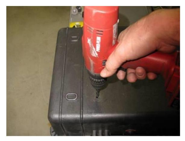
Step 12 Remove the rack from the box. Use the 21/64" drill bit and electric drill to enlarge the 1/4" pilot hole
