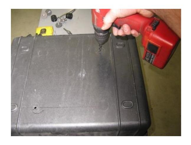
Step 16 Remove the rack from the box. Use the 21/64" drill bit and electric drill to enlarge the ¼" pilot hole
