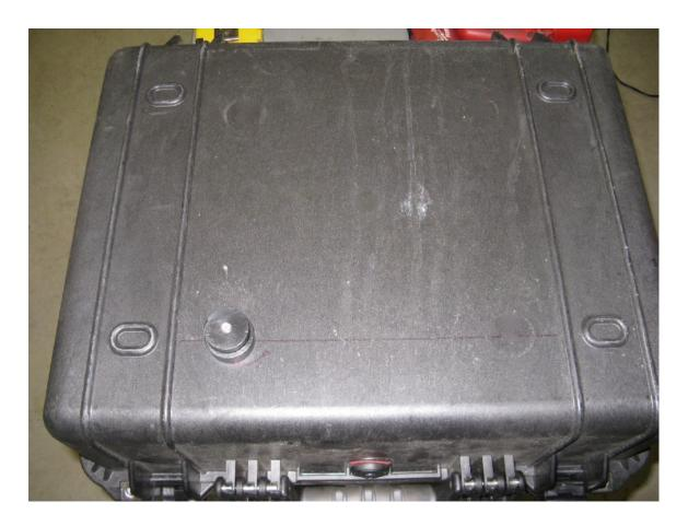
Step 13 Use the 5/16" button head cap screw and 1 ½" aluminum washer to attach the master puck to the box.
