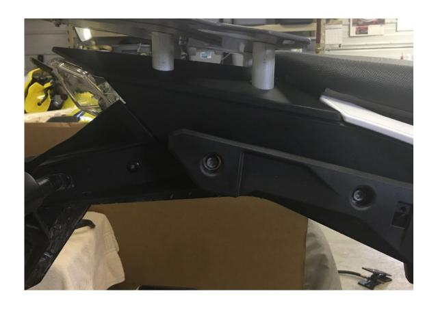
Step 4 Verify the Slider plate sits flush on the angled spacers.
