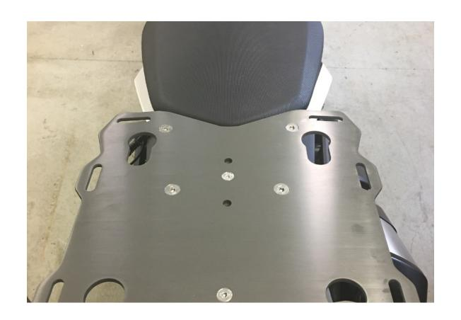
Step 20 Re-install the plate on the spacers. Re-install the M8 flat head screws and torque to 17 ftlbs.
