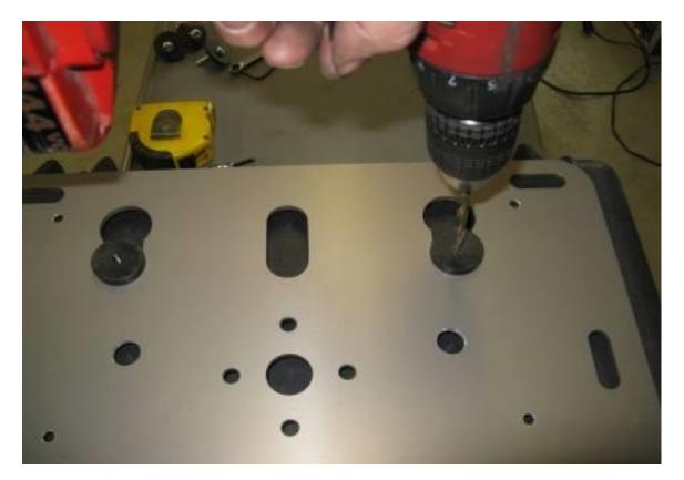
Step 15 With the ¼" drill bit, use the puck diagonally across from the master puck as a drill guide and drill a second pilot hole in the box.
