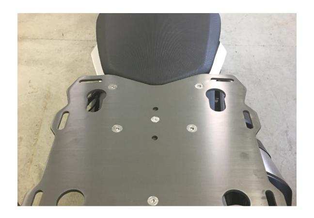
Step 3 Place the Slider plate on top of the spacers and install the longer bolts in the front and the shorter bolts in the rear. Tighten the rear bolts first, verify the bottom of the Slider plate sits flush on the top of the angled spacers. Repeat for the front screws.
