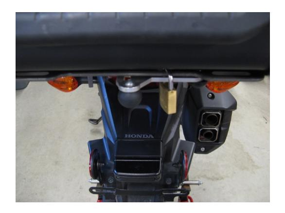
That completes the installation process. Test ride the motorcycle and then check all the fasteners for tightness. Also check the fasteners again after 1000 miles and at every oil change after that.
