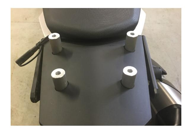
Step 2 Insert the 2 long spacers, angle up, in the forward location and the 2 short spacers, angle up, in the rear location.
