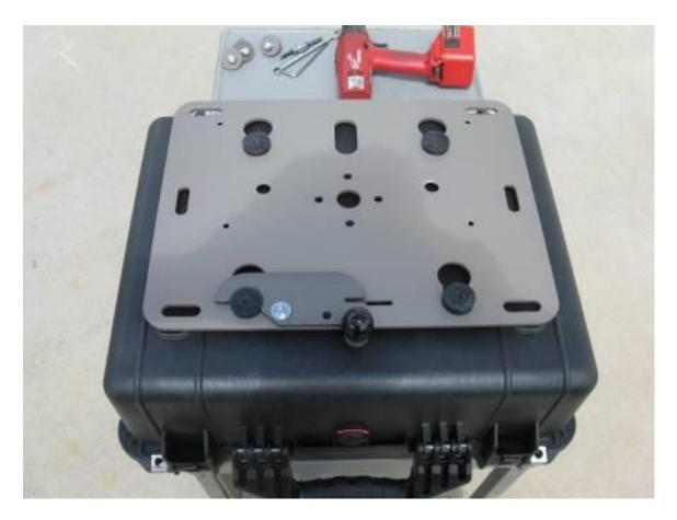
Step 9 Place the box on a table or other work surface. Remove the 4 flat head screws and nuts holding the rack onto the mounting brackets.
