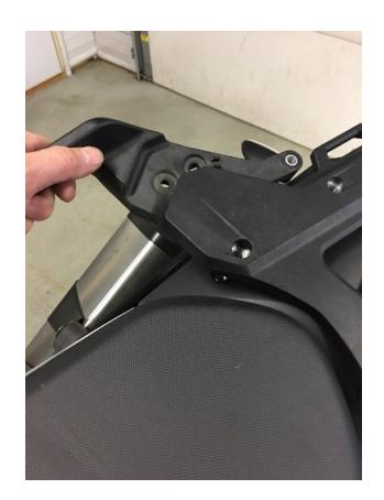
Step 1 Remove the OEM Top Plate and grab handles.
