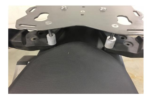
Step 6 Place the long angled spacers over the front holes of the grab handles. The spacer angled end must face upward and with the lowest point of the spacer facing toward the front of the motorcycle. Insert the 2 remaining 80mm BRE screws.
