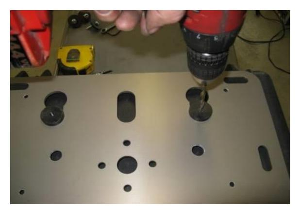
Step 18 With the ¼" drill bit, use the puck diagonally across from the master puck as a drill guide and drill a second pilot hole in the box.
