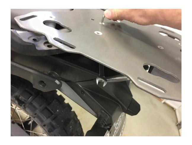
Step 8 Tighten the sub plate's two 6 mm screws and lock nuts using a hex key wrench and a 10mm combination wrench.
