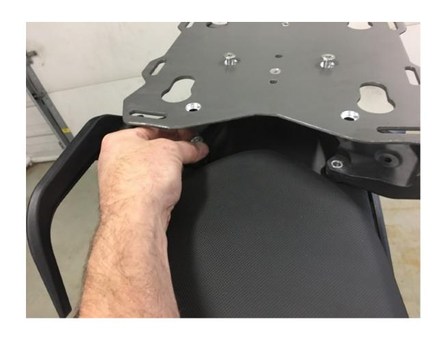
Step 5 Remove the front OEM screws.
