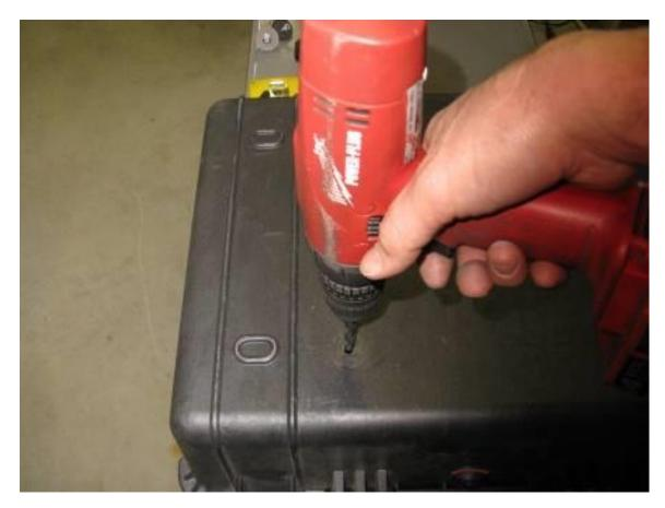
Step 15 Remove the rack from the box. Use the 21/64" drill bit and electric drill to enlarge the 1/4" pilot hole
