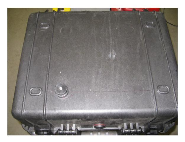
Step 16 Use the 5/16" button head cap screw and 1 ½" aluminum washer to attach the master puck to the box.
