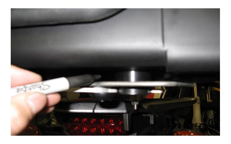
Step 11 Position the box on top of the pucks. Determine the for/aft location (side to side will be determined later). Position the box as far forward as possible without interfering with passenger comfort. Also consider if you will be placing any gear on the seat or if you want to be able to remove the seat with the box in place. Use a marker to mark the master puck location on the box.
