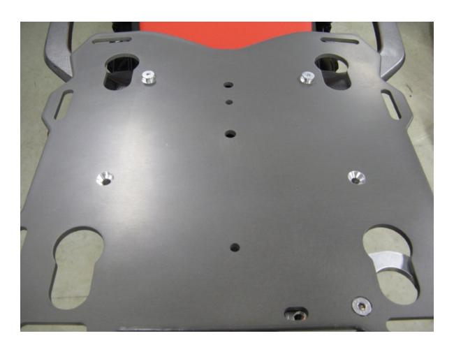
Step 23 Re-install the plate on the spacers. Re-install the M8 flat head screws and torque to 17 ftlbs.
