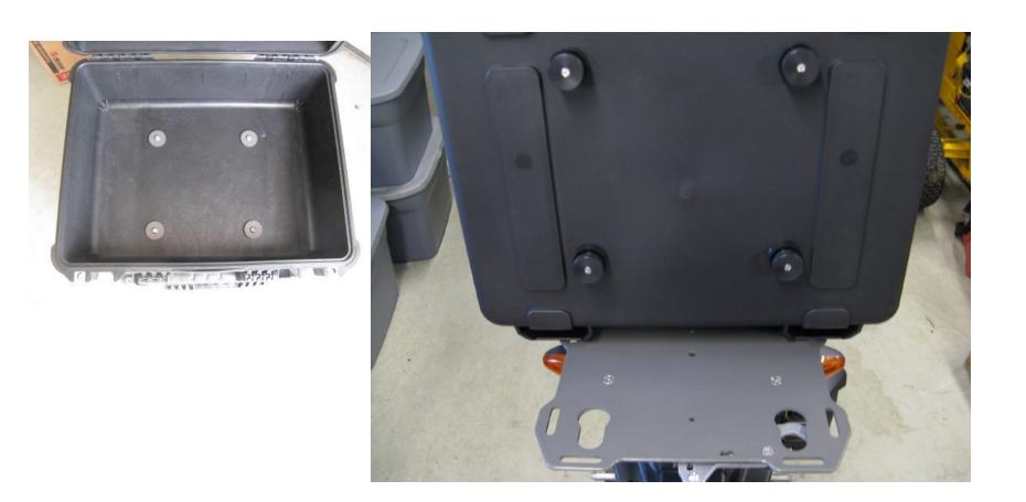
Step 22 Install all pucks onto the box using the 1½" aluminum washers and 5/16" button head cap screws.
