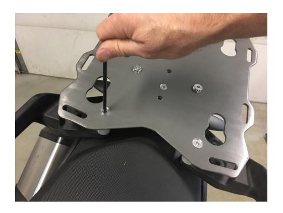
Step 7 Snug the four 80mm flat head screws with a hex wrench. Verify that the angled spacers are positioned correctly with the angled low point facing the front of the motorcycle.
