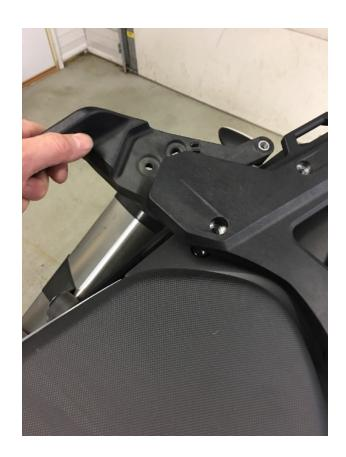
Step 1 Remove the OEM Top Plate and grab handles.
