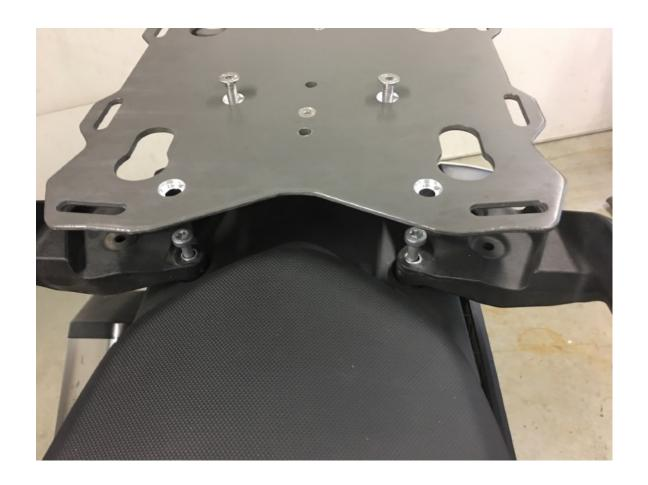
Step 4 Install the plate with the 2 rear BRE 80mm screws. Insert the screws through the spacers and thread into the subframe. Tighten the screws only 2- 3 revolutions at this time.
