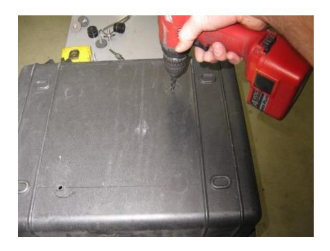
Step 19 Remove the rack from the box. Use the 21/64" drill bit and electric drill to enlarge the 1/4" pilot hole
