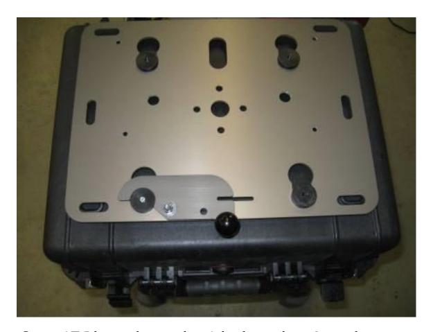
Step 17 Place the rack with the other 3 pucks onto the master puck and latch it into position. Square up the plate and box to each other (last chance).
