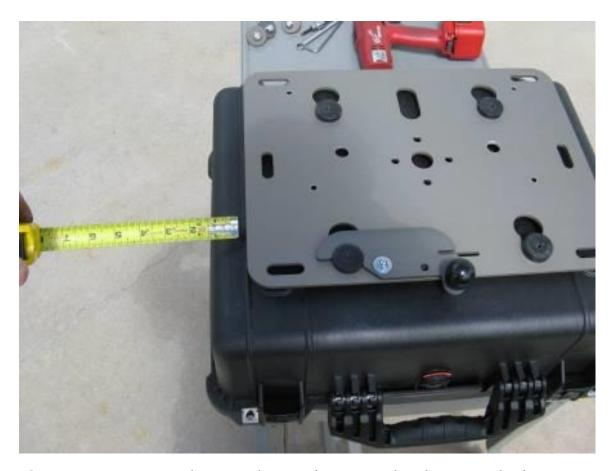
Step 13 Locate the puck marker on the box and align the master puck up with the mark as it was on the bike.
