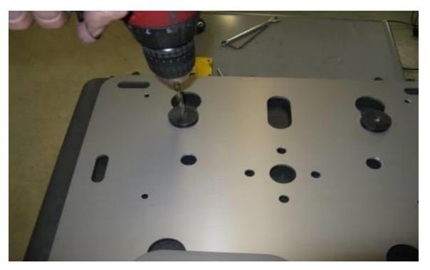
Step 20 Bolt the second puck to the box. Place the rack on the box and latch it into position. With the ¼" drill bit use the 2 remaining pucks as drill guides and drill the last 2 pilot holes.
