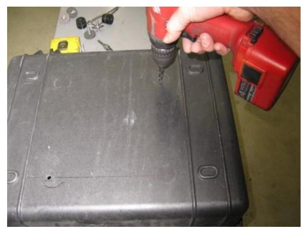
Step 17 Remove the rack from the box. Use the 21/64" drill bit and electric drill to enlarge the ¼" pilot hole
