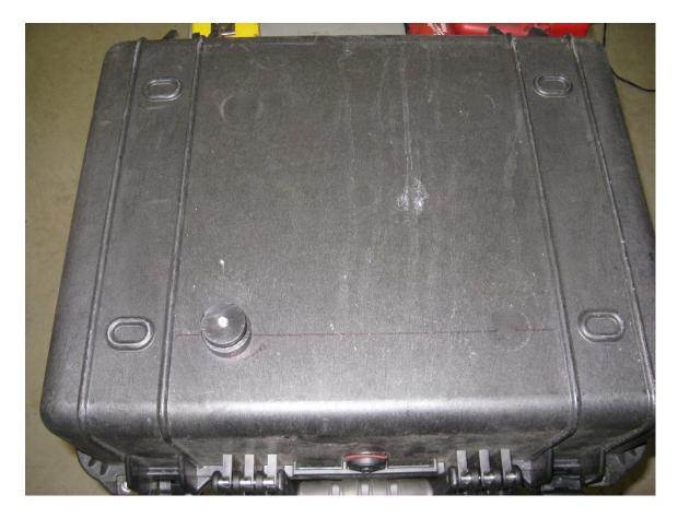
Step 14 Use the 5/16" button head cap screw and 1 ½" aluminum washer to attach the master puck to the box.
