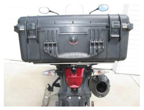
Step 22 Install the box onto rack and latch it into place with the cam lever.
