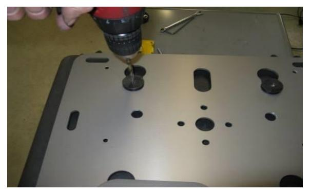
Step 18 Bolt the second puck to the box. Place the rack on the box and latch it into position. With the ¼" drill bit use the 2 remaining pucks as drill guides and drill the last 2 pilot holes.
