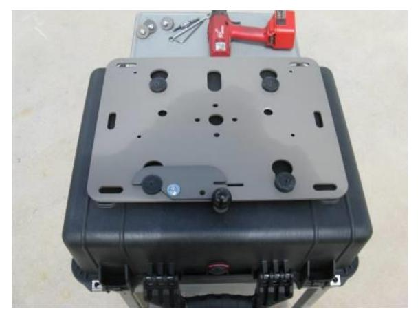
Step 10 Place the box on a table or other work surface. Remove the 4 flat head screws and nuts holding the Slider plate onto the motorcycle.
