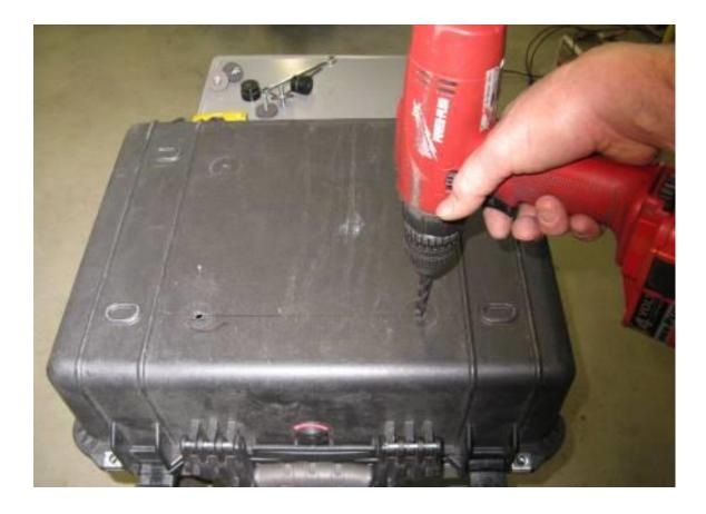
Step 19 Remove the rack and pucks from the box. Use the 21/64" drill bit and electric drill to enlarge the last two ¼" pilot holes.
