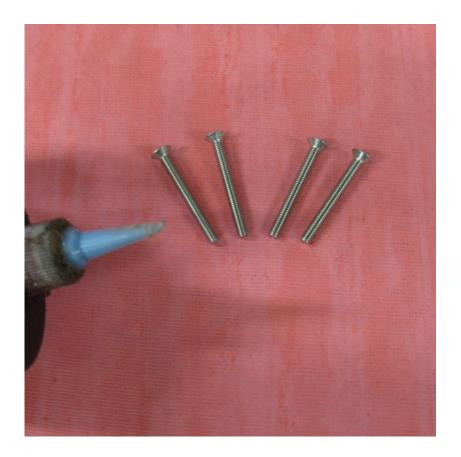
Apply 242 Blue Loctite or similar thread locker to the four M6 x 55 flat head screws.
