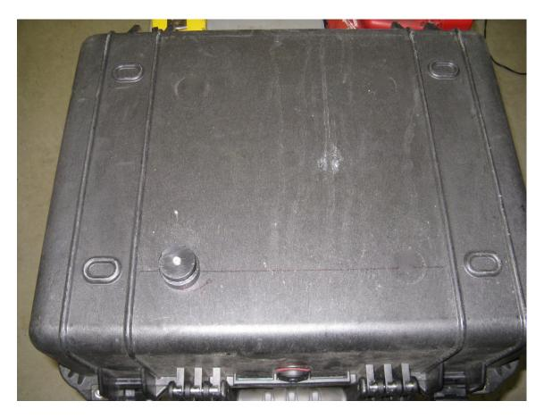
Step 14 Use the long 5/16" button head cap screw and 1 ½" aluminum washer to attach the master puck to the box.
