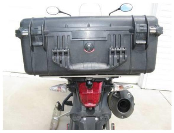
Step 23 Install the box onto rack and latch it into place with the cam lever.
