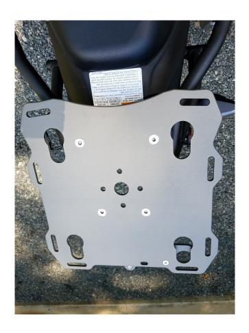
Step 2 Install the 4 spacers underneath the rack. Install the Slider plate over the top of the spacers, insert the flathead screws through the spacers and thread into the subframe. Snug screws at this time.
