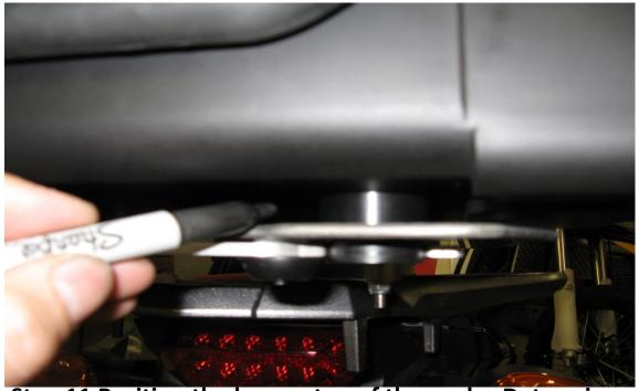
Step 11 Position the box on top of the pucks. Determine the for/aft location (side to side will be determined later). Position the box as far forward as possible without interfering with passenger comfort. Also consider if you will be placing any gear on the seat or if you want to be able to remove the seat with the box in place. Use a marker to mark the master puck location on the box.
