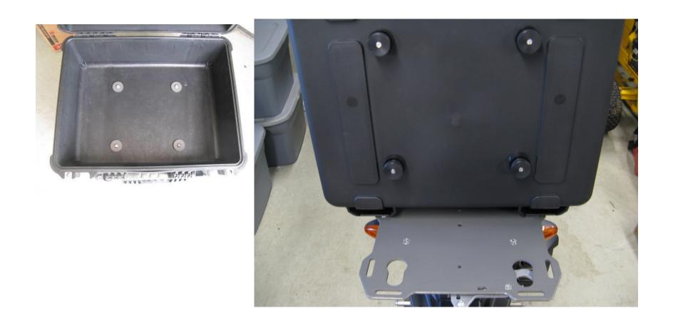
Step 20 Install all pucks onto the box using the 1 ½" aluminum washers and 5/16" button head cap screws.
