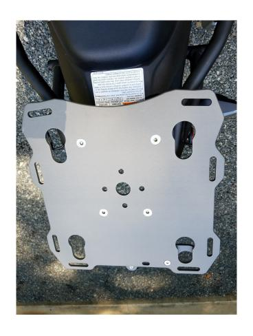
Step 22 Re-install the plate on the spacers and torque the flat screws to 18 ft. lbs.
