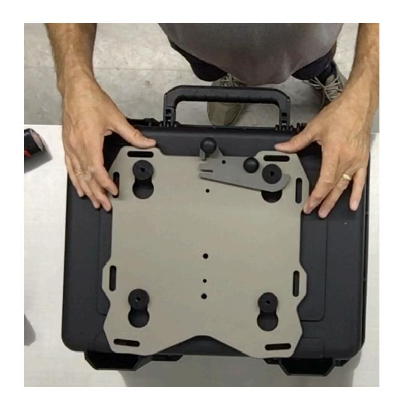
**Step 12** Place the case on a table or other work surface. Remove the 6 M6 flat head screws and nuts holding the Slider plate onto the OEM tube rack. Place the Slider plate with the pucks installed on the case.
