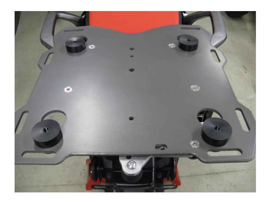
**Step 10** Insert the 3 remaining pucks into the keyholes in the plate.
