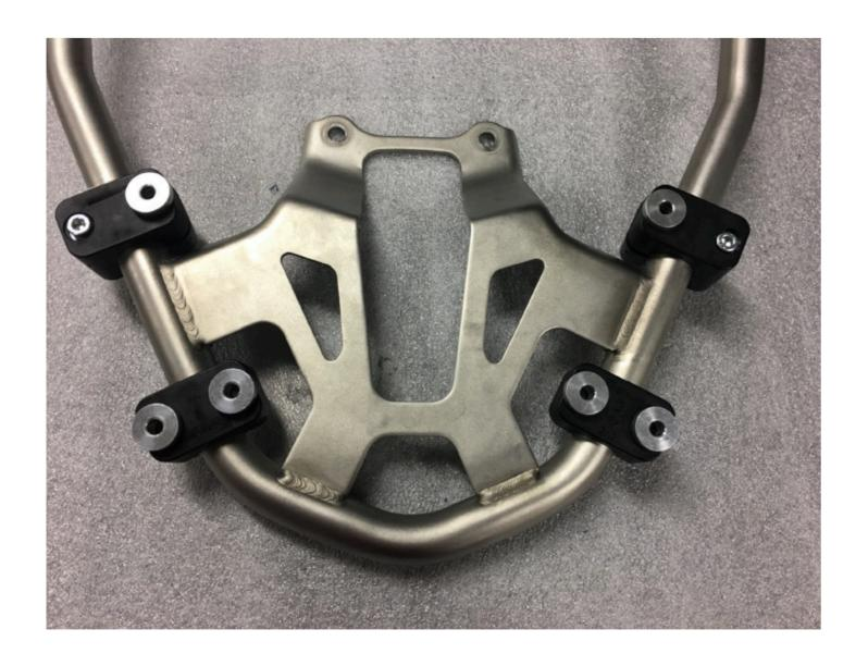
**Step 5** Install 2 clamp halves to the rear of the OEM rack as shown in the photo. Insert the 4 remaining 19 mm stepped spacers as shown.
