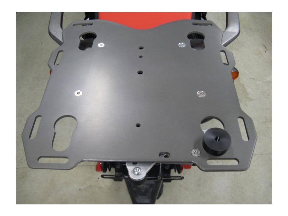
**Step 9** Install one of the black plastic pucks into the key hole with the cam lever. Lock the puck into place with the cam lever. This will be referred to as the "Master Puck" **Note**: Remove the large washer and screw from the puck before putting into the plate. The screws and washers are installed into the pucks for shipment as part of our QA process.
