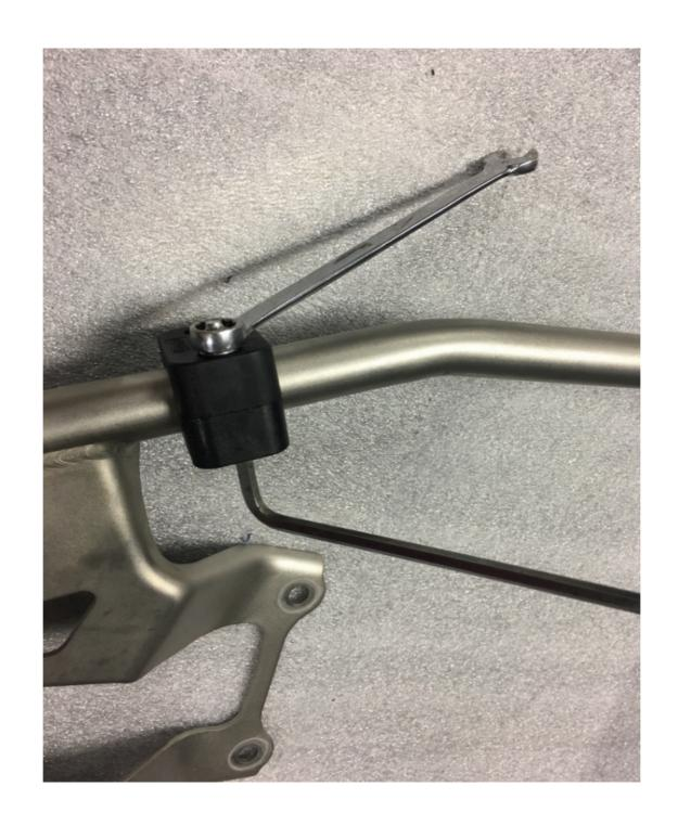
**Step 3** Place the 4mm spacers under the heads of the M6 socket head screw, insert the screw through the outer hole of the clamp. Slip 11 mm spacer over screw and thread the M6 lock nut onto the screw. Tighten the M6 lock nut until the clamp is completely closed as shown in the photo.
