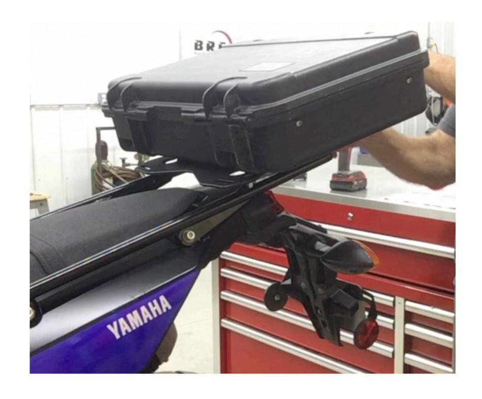
**Step 24** Install the case onto rack and latch it into place with the cam lever.
