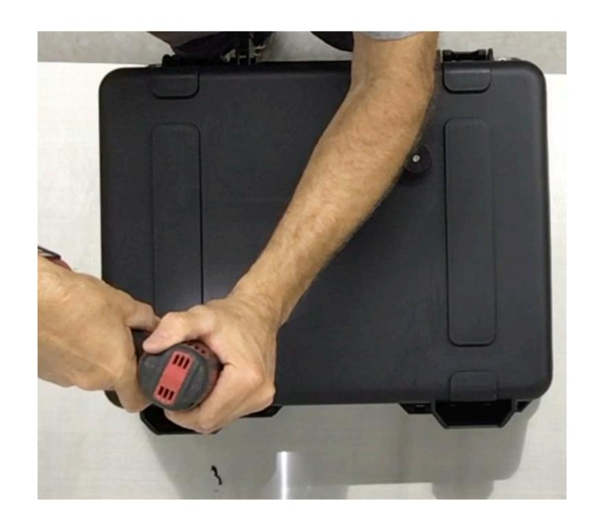
**Step 19** Remove the slider plate from the case and use the 21/64" drill bit to enlarge the second 1/4" pilot hole.
