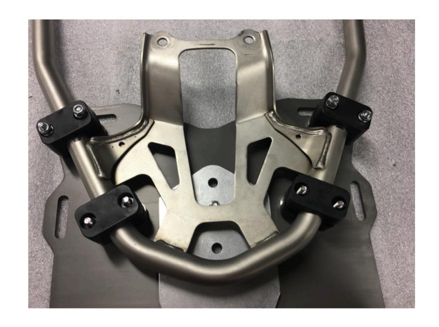
**Step 7** Place the rear clamp halves on as shown. Install the two remaining 11mm spacers and M6 lock nuts on the inner front 60 mm screws.
