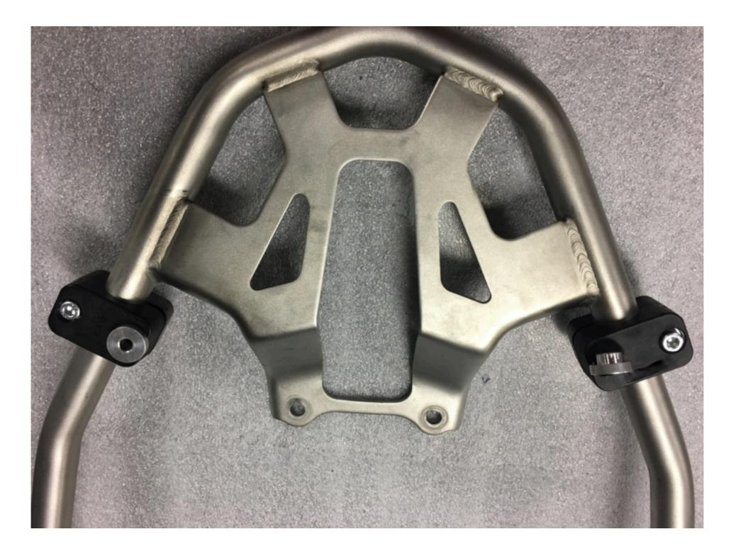
Step 4 Insert a 19mm stepped spacer into each of the inner clamp holes as shown.
