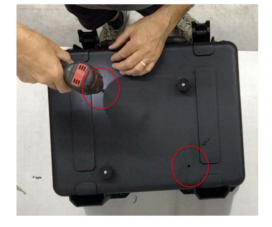
**Step 21** Remove the Slider rack and pucks from the case. Use the 21/64" drill bit and electric drill to enlarge the last two  $\frac{1}{4}$ " pilot holes.
