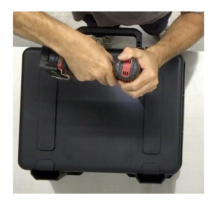
**Step 15** Remove the Slider plate from the case. Use the 21/64" drill bit and electric drill to enlarge the  $\frac{1}{4}$ " pilot hole.
