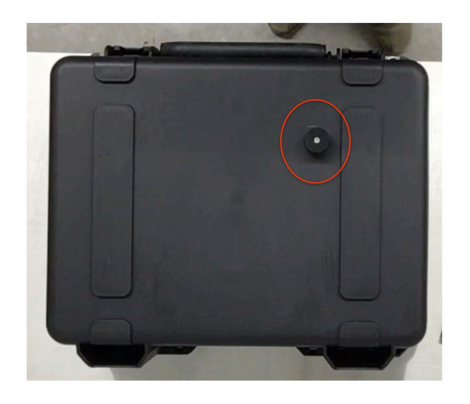
**Step 16** Use a M8 x 38 flat washer and the M8 button head cap screw to attach the master puck to the case.
