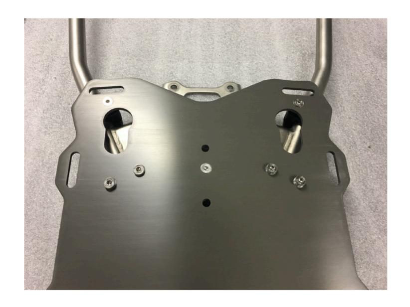
**Step 6** Set the Slider plate on top of the clamps. Insert the six M6 x 60 mm flat head screws through the Slider plate and the clamps as shown.
