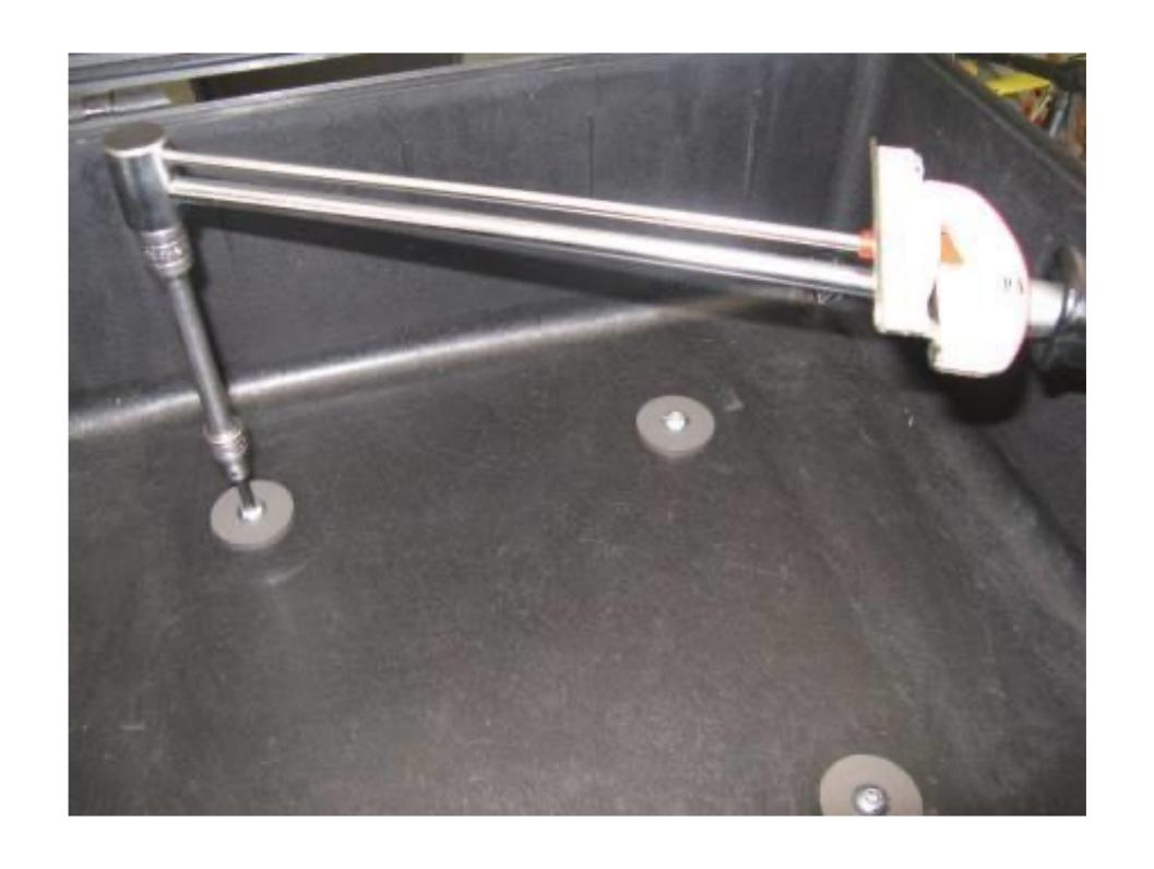
Step 25 Torque the puck screws to 9 ft.lb. or 12.2 Nm.
