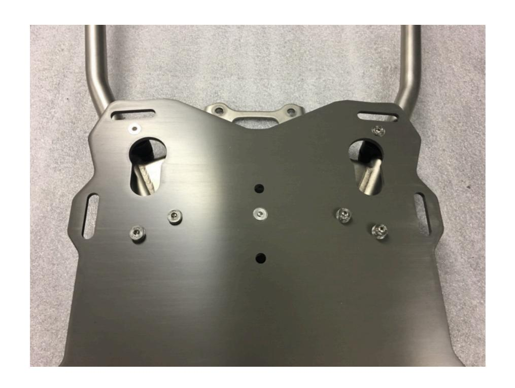
**Step 23** Re-attach the plate using the six M6 x 60 flat head screws, clamp halves and M6 lock nuts. **Torque** the screws to 8ft.lbs.
