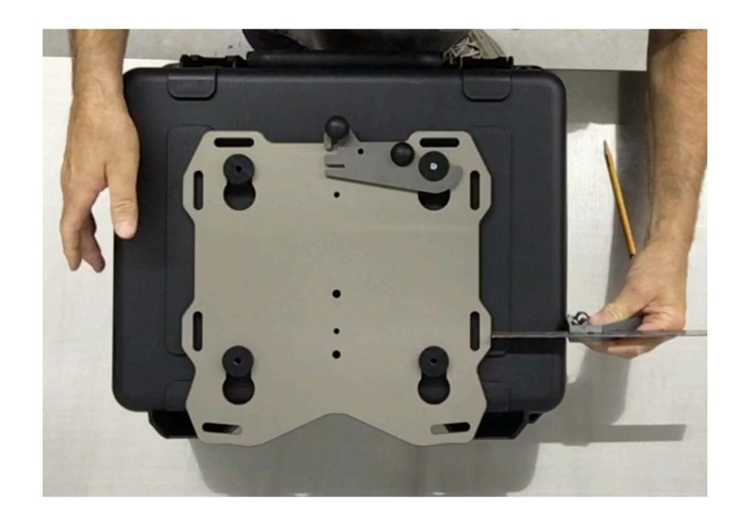
**Step 17** Place the Slider plate with the other 3 pucks onto the master puck and latch it into position. Square up the plate and box to each other (last chance).
