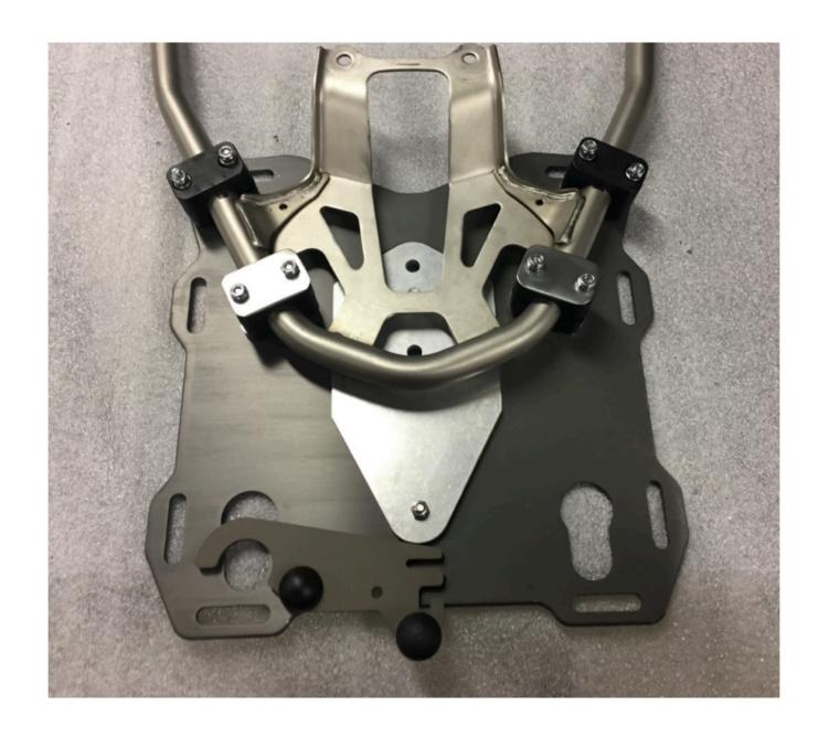
**Step 8** Install the stainless steel clamp plates and M6 lock nuts on the rear clamps as shown. All of the clamp screws can be tightened at this time. There should be no gap between the clamp halves when the M6 lock nuts are properly tightened.
