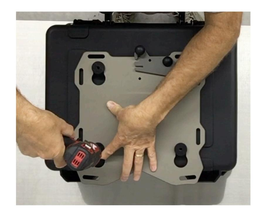
**Step 18** With the  $\frac{1}{4}$ " drill bit, use the puck diagonally across from the master puck as a drill guide and drill a second pilot hole in the case.
