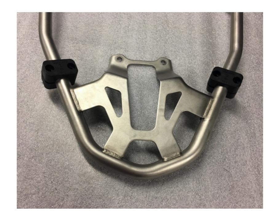
**Step 2** Position the 4 front clamp halves as shown. **Note:** It is not necessary to remove the rack from the motorcycle. For ease of illustration the photos are shown with the rack not installed on the motorcycle.
