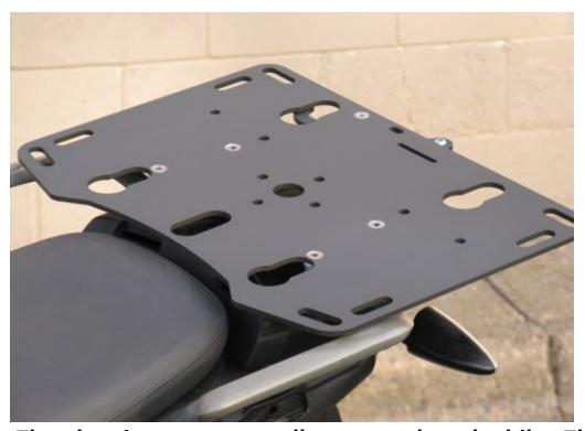
The plate is now temporally mounted on the bike. The next steps explain how to locate and mount the quick connect pucks to the top case. The motorcycle shown in some photos may not be exactly the same as your bike, but the process is the same for all bikes.
