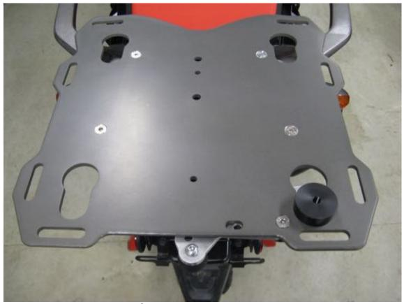
Step 9 Install one of the black plastic pucks into the key hole with the cam lever. Lock the puck into place with the cam lever. This will be referred to as the "Master Puck"
