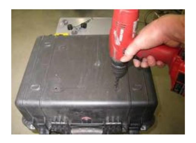
**Step 19** Remove the rack and pucks from the box. Use the 21/64" drill bit and electric drill to enlarge the last 2 ¼" pilot holes.
