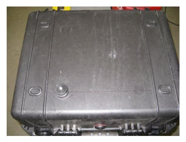
**Step 14** Use the 8mm button head cap screw and 38mm aluminum washer to attach the master puck to the box.
