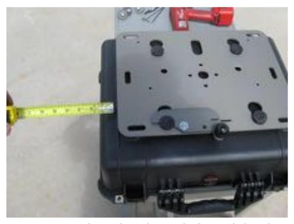
**Step 11** Locate the puck marker on the box and align the master puck up with the mark as it was on the bike.
