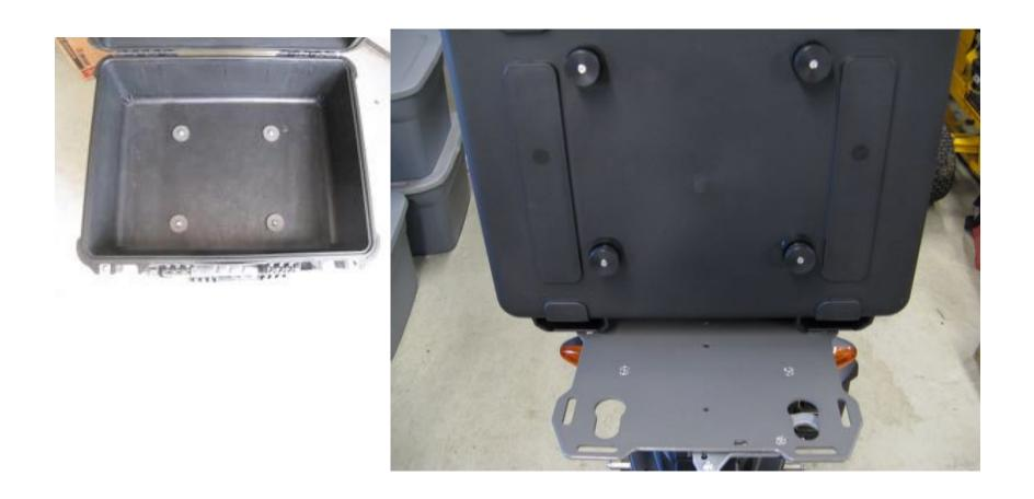
**Step 20** Install all pucks onto the box using the 38mm aluminum washers and 8mm button head cap screws.
