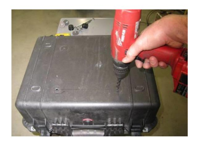
Step 18 Remove the rack and pucks from the box. Use the 21/64" drill bit and electric drill to enlarge the last 2 1/4" pilot holes.
