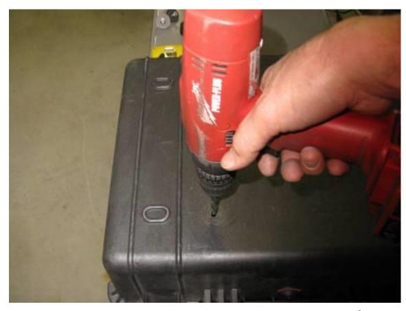
Step 12 Remove the rack from the box. Use the 21/64" drill bit and electric drill to enlarge the ½" pilot hole
