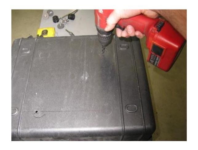
Step 16 Remove the rack and pucks from the box. Use the 21/64" drill bit and electric drill to enlarge the second 1/4" pilot hole.
