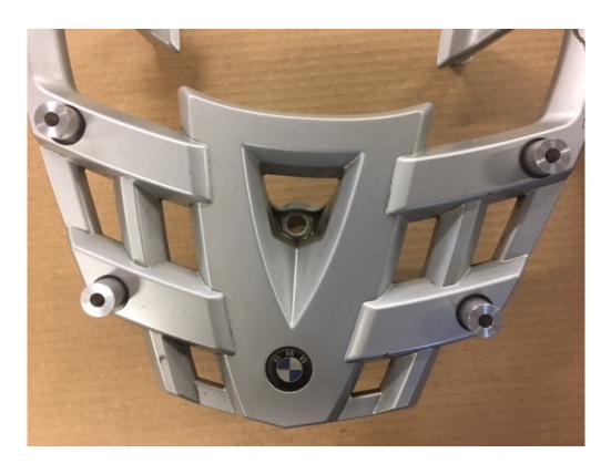
Step 20 Re-install the plate on the spacers. Re-install the M6 flat head screws and lock nuts, torque to 100 inlbs.
