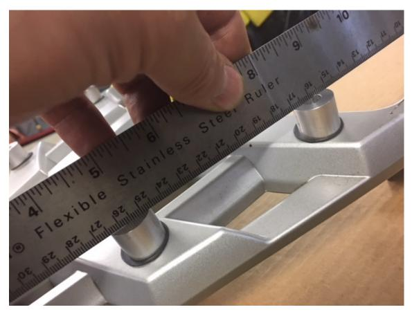
Step 4 The straight edge should also lay flat across the front and rear spacers. Rotate if needed.
