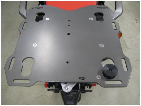
Step 6 Install one of the black plastic pucks into the key hole with the cam lever. Lock the puck into place with the cam lever. This will be referred to as the "Master Puck"
