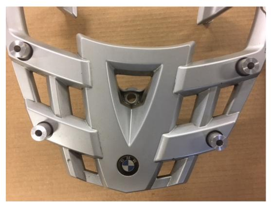
Step 2 Install the supplied aluminum spacers angled side down with the short side of the spacer facing the spacer on the opposite side of the bike.
