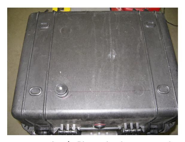
Step 13 Use the 5/16" button head cap screw and  $1 \frac{1}{2}$ " aluminum washer to attach the master puck to the box.
