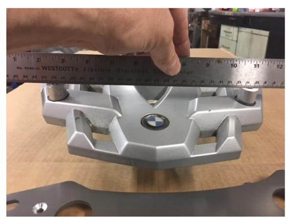
Step 3 use a straight edge to help position the spacers. The straight edge should lay flat across the 2 front spacers and the 2 rear spacers. Rotate the spacers if needed.
