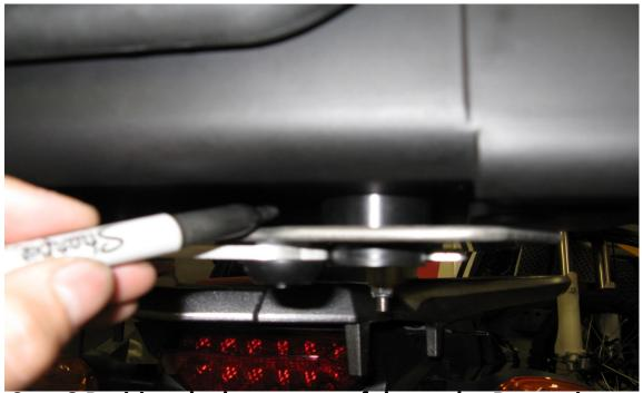
Step 8 Position the box on top of the pucks. Determine the for/aft location (side to side will be determined later). Position the box as far forward as possible without interfering with passenger comfort. Also consider if you will be placing any gear on the seat or if you want to be able to remove the seat with the box in place. Use a marker to mark the master puck location on the box.
