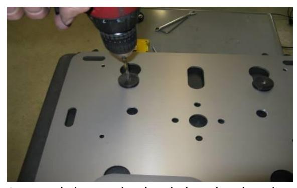
Step 17 Bolt the second puck to the box. Place the rack on the box and latch it into position. With the ¼" drill bit use the 2 remaining pucks as drill guides and drill the last 2 pilot holes.
