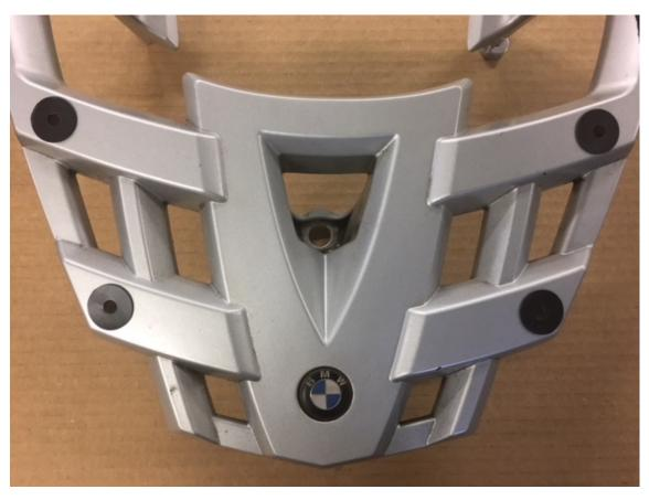
Step 1 Install a supplied rubber washer over each of the 4 holes on the OEM rack.
