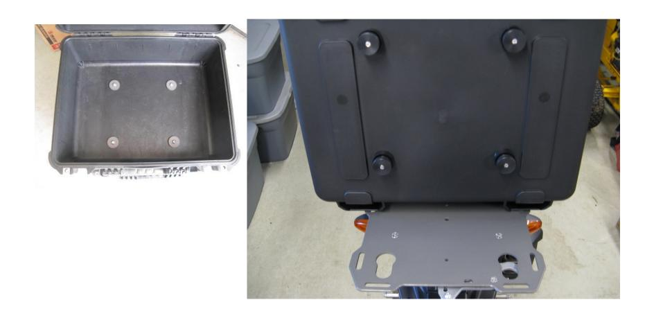
Step 16 Install all pucks onto the box using the 1 ½" aluminum washers and 5/16" button head cap screws.
