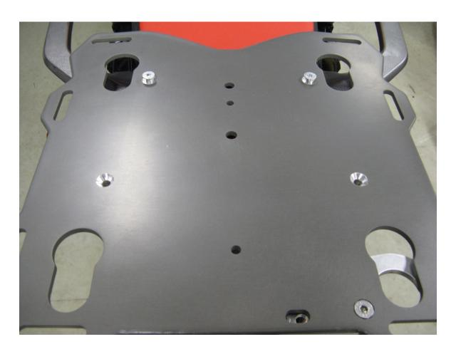
Step 17 Re-install the plate on the spacers. Re-install the M8 flat head screws and torque to 17 ftlbs.
