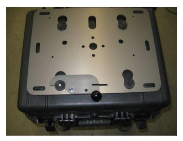
Step 11 Place the rack with the other 3 pucks onto the master puck and latch it into position. Square up the plate and box to each other (last chance).
