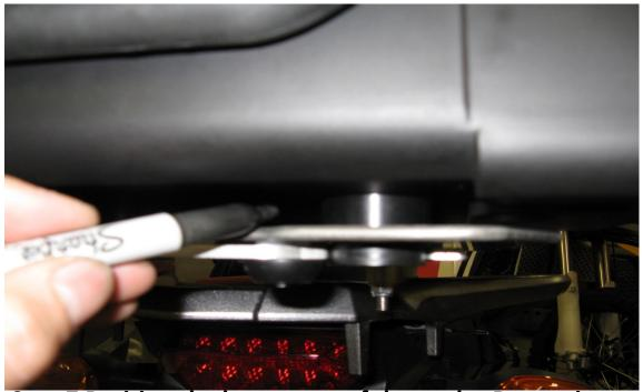
Step 7 Position the box on top of the pucks. Determine the for/aft location (side to side will be determined later). Position the box as far forward as possible without interfering with passenger comfort. Also consider if you will be placing any gear on the seat or if you want to be able to remove the seat with the box in place. Use a marker to mark the master puck location on the box.
