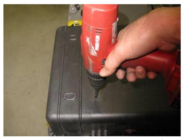
Step 13 Remove the rack from the box. Use the 21/64" drill bit and electric drill to enlarge the ½" pilot hole
