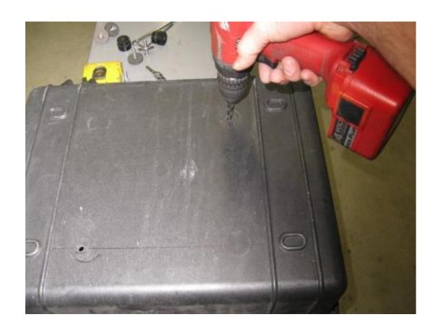
Step 13 Remove the rack and pucks from the box. Use the 21/64" drill bit and electric drill to enlarge the second 1/4" pilot hole.
