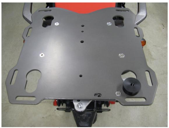
Step 5 Install one of the black plastic pucks into the key hole with the cam lever. Lock the puck into place with the cam lever. This will be referred to as the "Master Puck"
