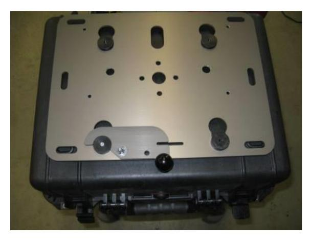
**Step 15** Place the rack with the other 3 pucks onto the master puck and latch it into position. Square up the plate and box to each other (last chance).
