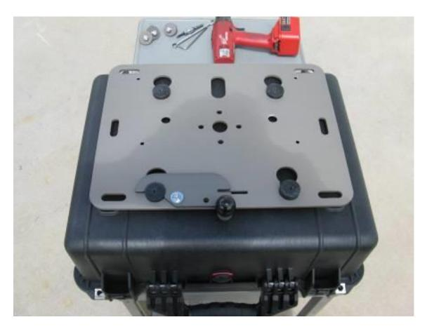
**Step 10** Place the box on a table or other work surface. Remove the 4 flat head screws holding the rack onto the motorcycle.
