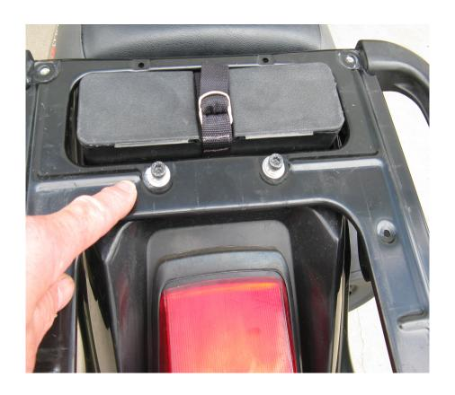
**Step 3** Re-install the 2 socket head 6 mm screws with the original washers, apply 242 blue Loctite. Torque the screws to 105 inch pounds.
