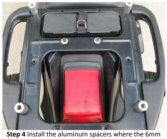
**Step 4** Install the aluminum spacers where the 6mm threaded holes are located.
