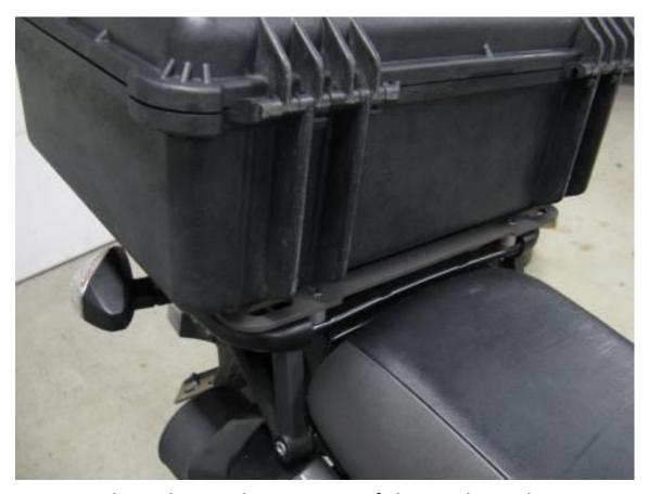
**Step 8** Place the top box on top of the pucks and position it where you would like it located.
