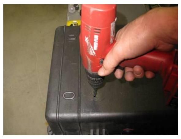
**Step 13** Remove the rack from the box. Use the 21/64" drill bit and electric drill to enlarge the ¼" pilot hole.
