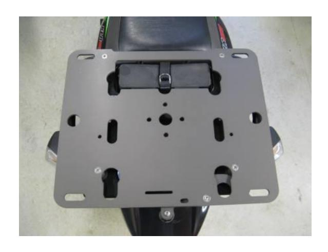
**Step 6** Attach the rack to the motorcycle with the 4 flat head screws as shown. Just snug the screws for now as you will be removing them in a later step.
