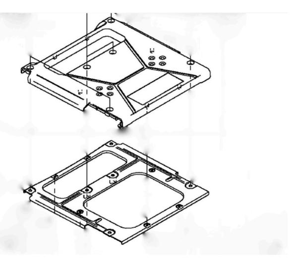
**Step 2** Look at the underneath of the plastic OEM rack. There is a stamped steel plate screwed to the plastic rack. Remove the stamped steel part, **THIS MUST BE INSTALLED BACK ON THE MOTORCYCLE!**
