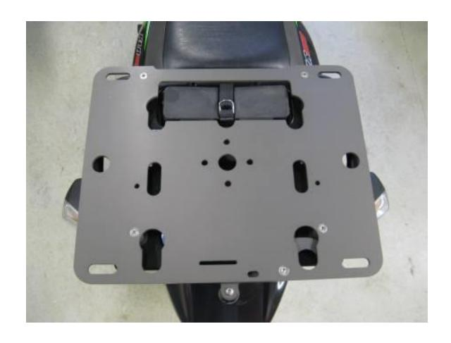
**Step 21** Apply Blue 242 Loctite to the 4 flat head screws and attach the the rack with the screws. Torque the fasteners to 100 inch pounds. This completes the rack installation.
