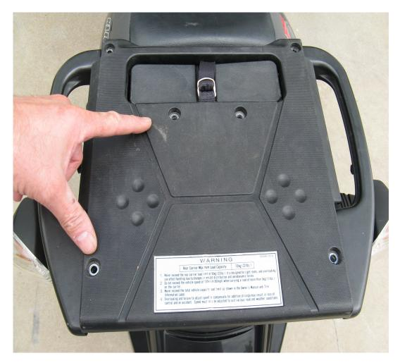
**Step 1** Remove the 4 tail cover screws.
