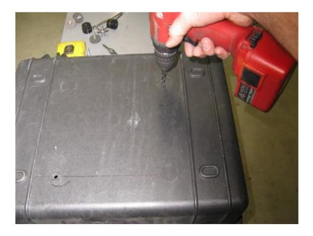
Step 15 Remove the rack and pucks from the box. Use the 21/64" drill bit and electric drill to enlarge the second ¼" pilot hole.
