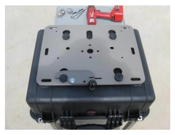
Step 8 Place the box on a table or other work surface. Remove the 4 flat head screws and nuts holding the rack onto the stainless steel brackets.
