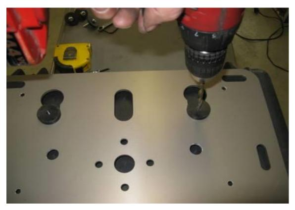
Step 14 With the ¼" drill bit, use the puck diagonally across from the master puck as a drill guide and drill a second pilot hole in the box.
