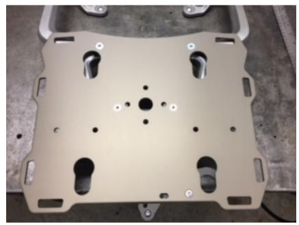
Step 4 Insert the two M8 X 40 screws into the front of the plate, through the spacers and OEM rack. Thread the M8 flange nuts onto the screws. Insert the 2 M6 x 40 screws through the plate, spacers and OEM rack in the rear. Install an M6 washer on each bolt, thread the M6 nuts onto the screws. You will be using the plate as a drill template later so do not apply final torque on these screws now.
