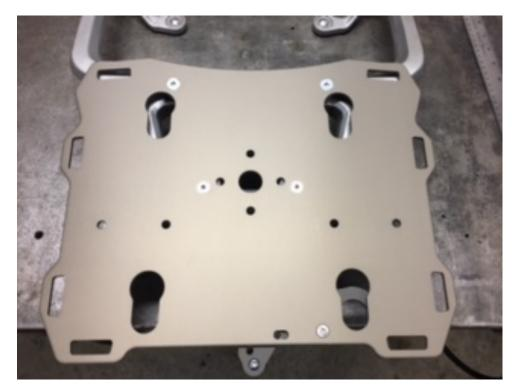
Step 20 Insert the two M8 X 40 screws into the front of the plate, through the spacers and OEM rack. Thread the M8 nuts onto the screws. Insert the 2 M6 x 40 screws through the plate, spacers and OEM rack in the rear. Thread the M6 nuts onto the screws.
