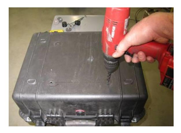
Step 17 Remove the rack and pucks from the box. Use the 21/64" drill bit and electric drill to enlarge the last 2 ¼" pilot holes.
