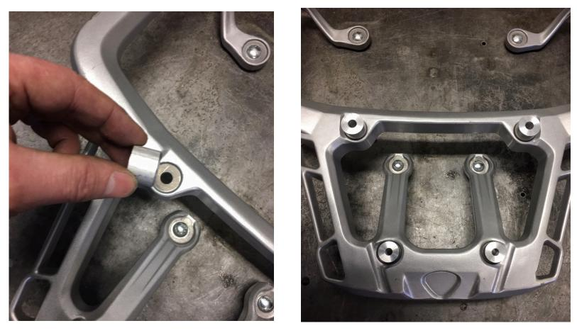
Step 2 Install the 4 aluminum spacers where the screws were. The large diameter spacers go closest to the seat. The spacer has a chamfer on one end, this faces downward.
