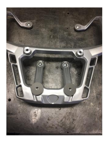
Step 3 Install the two 1.5" aluminum washers on top of the rear spacers.
