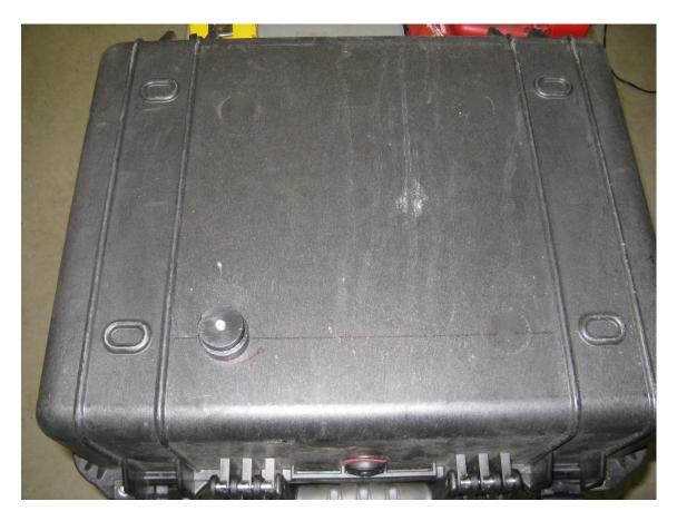
Step 12 Use the long 5/16" button head cap screw and 1 ½" aluminum washer to attach the master puck to the box.
