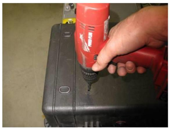
Step 11 Remove the rack from the box. Use the 21/64" drill bit and electric drill to enlarge the ¼" pilot hole
