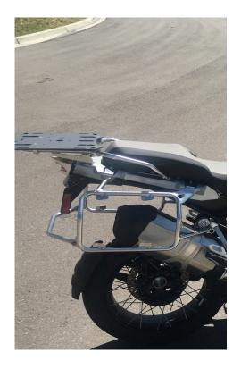
The plate is now temporally mounted on the bike. The next steps explain how to locate and mount the quick connect pucks to the top case. The motorcycle shown in some photos may not be exactly the same as your bike, but the process is the same for all bikes.
