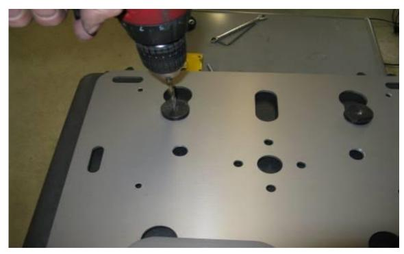
Step 16 Bolt the second puck to the case. Place the plate on the case and latch it into position. With the ¼" drill bit use the 2 remaining pucks as drill guides and drill the last 2 pilot holes.
