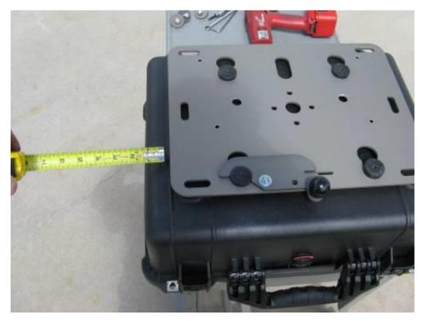
Step 9 Locate the puck marker on the box and align the master puck up with the mark as it was on the bike.
