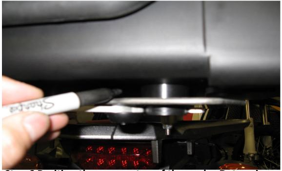
Step 6 Position the case on top of the pucks. Determine the for/aft location (side to side will be determined later). Position the case as far forward as possible without interfering with passenger comfort. Also consider if you will be placing any gear on the seat or if you want to be able to remove the seat with the case in place. Use a marker to mark the master puck location on the case.
