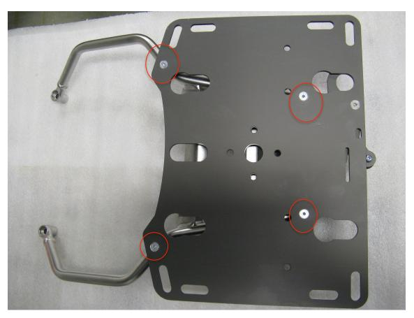
Step 2 Note tube rack is shown removed from the bike, it is *not* necessary to remove from the bike for installation. Loosen the 4 collar retaining screws just enough so you can <u>rotate</u> the collars. Place the plate with the collars onto the tube rack.
