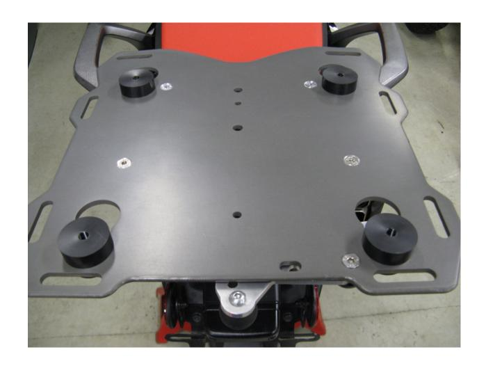
Step 5 Insert the 3 remaining pucks into the keyholes in the plate.
