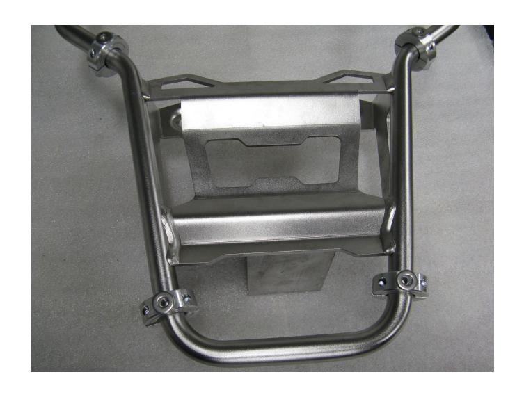
Step 19 Re-install the Slider plate on the washers and mounting collars.
