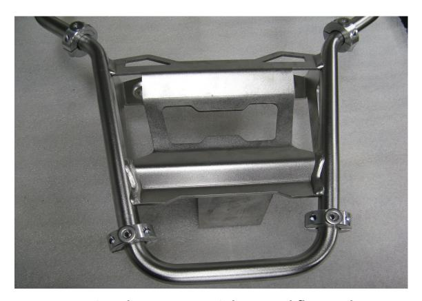
Step 7 Caution there are 4 stainless steel flat washers that will be exposed during this next step, do not loose them! Remove the 4 flat head screws from the Slider plate and remove the plate. The collars will be firmly clamped into the correct position on the tube rack. Remove the 4 stainless steel washers from the collars.
