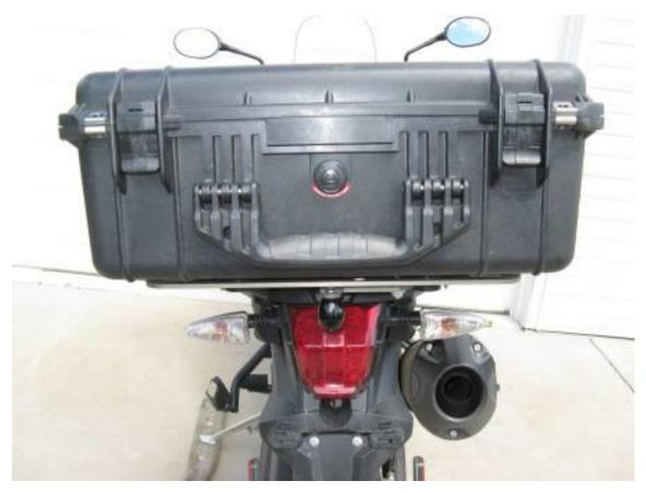
Step 21 Install the box onto rack and latch it into place with the cam lever.
