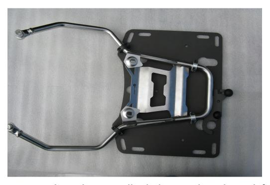
Step 3 Adjust the top collar halves so the tube rack fits snugly in the collars. The Slider plate should be positioned on the tube rack as shown in the photo. Install the bottom collar halves back onto the top collars. Using a 3/16" hex key wrench hand tighten the screws. Once the rack is positioned correctly and the collars fit snug to the tube rack, torque the 8 screws to 120 in. lbs.
