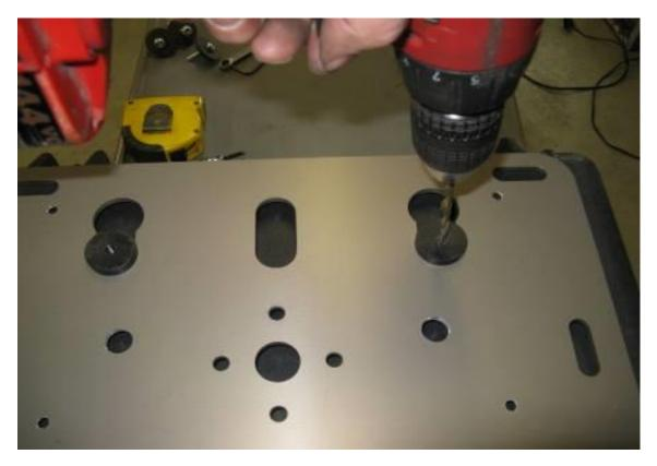
Step 14 With the ¼" drill bit, use the puck diagonally across from the master puck as a drill guide and drill a second pilot hole in the case.
