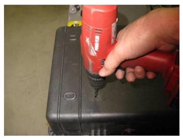
Step 11 Remove the plate from the case. Use the 21/64" drill bit and electric drill to enlarge the  $\frac{1}{4}$ " pilot hole
