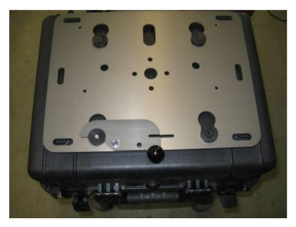
Step 13 Place the plate with the other 3 pucks onto the master puck and latch it into position. Square up the plate and case to each other (last chance).
