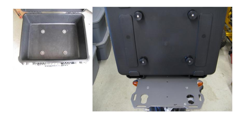
Step 18 Install all pucks onto the case using the 1 ½" aluminum washers and 8 mm button head cap screws.
