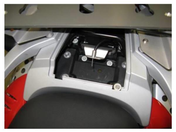
Step 23 Insert cable end into cable bracket as shown.
