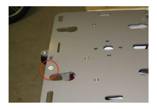
Step 24 Tighten the M6 lock nut on the lever pivot bolt to adjust lever force. Lever should be snug but rotate without great effort.
