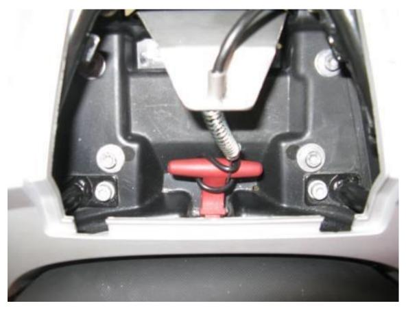
Step 27 Loop the retaining 0-ring around the cable loop and seat latch as shown.
