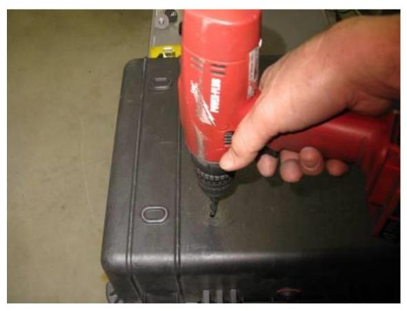
Step 7 Remove the rack from the box. Use the 21/64" drill bit and electric drill to enlarge the ¼" pilot hole
