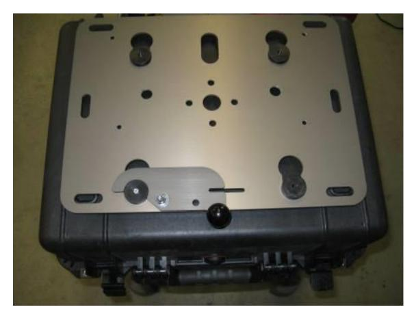
Step 9 Place the rack with the other 3 pucks onto the master puck and latch it into position. Square up the plate and box to each other (last chance).
