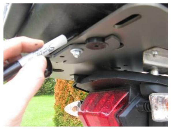
Step 3 Mark the location of the master puck onto the top box with a marker.
