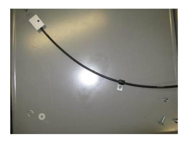
Step 14 Install the loop clamp onto the cable.
