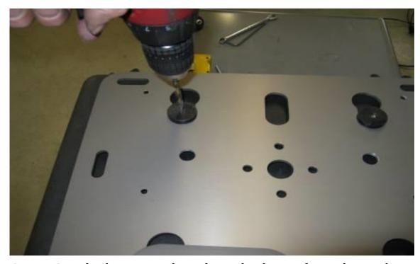
Step 12 Bolt the second puck to the box. Place the rack on the box and latch it into position. With the ¼" drill bit use the 2 remaining pucks as drill guides and drill the last 2 pilot holes.
