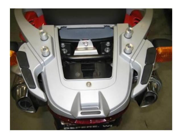
Step 4 Install the aluminum spacers on grab handles.
