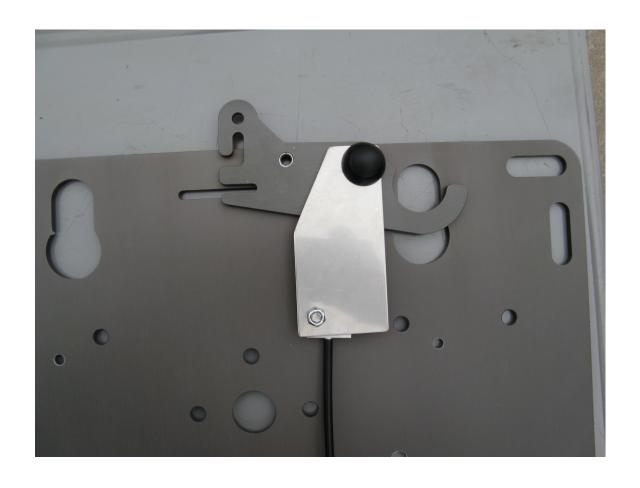
By hand, press the black plastic cap into cap base.
