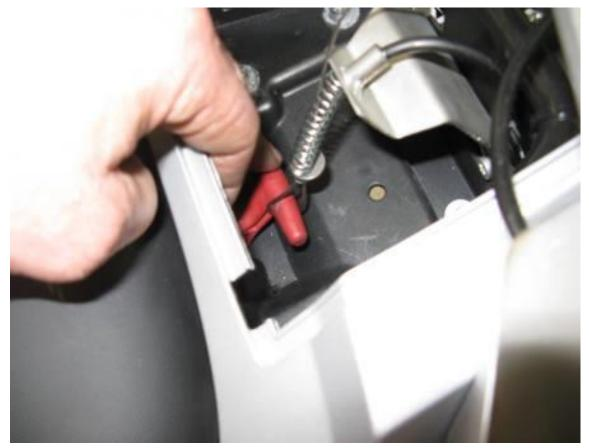
Step 26 Verify the seat latch is in the fully downward position. Adjust the loop on the cable so it hooks around the latch as shown. Then tighten the set screw on the cable clamp. Cut off the excess cable with a side cutter.
