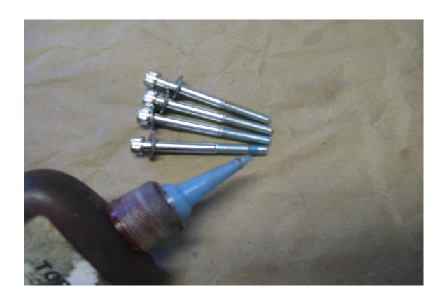
Step 5 Install the four 6mm washers on the M6 x 60 socket head screws. Apply thread locker to the screws.
