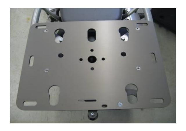
Step 15 Attach the rack to the stainless steel brackets with the 6mm flat head screws and 6 mm lock nuts.
