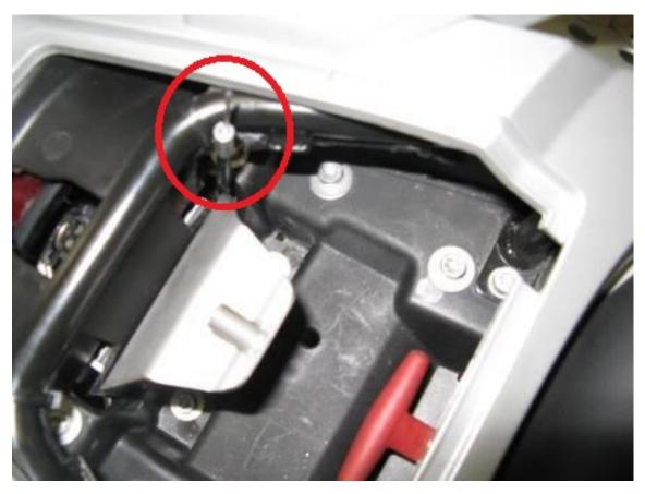
Step 20 Insert the free end of the cable through the previously identified hole.
