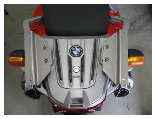
Step 6 Install the 2 stainless steel brackets with four 6mm x 60 (5 mm head) socket head screws. Note: The bracket with the inner hole closest to the edge is located toward the front of the bike.
