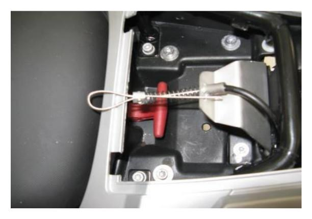
Step 25 Install the spring and cable clamp, loop the cable and thread it back through the cable clamp as shown.
