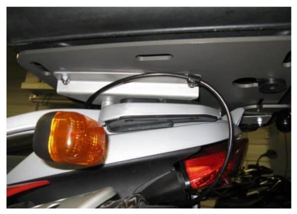
Step 28 Route the cable as shown. Attach the cable loop clamp to the rear LH plate bolt as shown. Install the assembled plate to the stainless steel brackets as shown.
