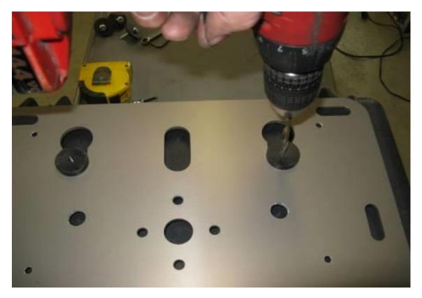
Step 10 With the ¼" drill bit, use the puck diagonally across from the master puck as a drill guide and drill a second pilot hole in the box.
