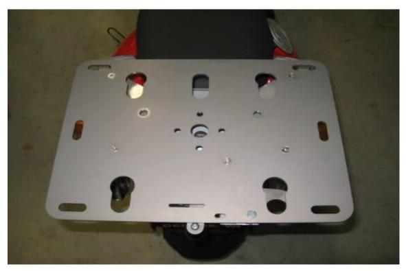
The rack installation is complete. Test the seat latch mechanism. The seat should be able to be removed when the lever is fully opened and when the lever is closed the seat should not come off the bike.
