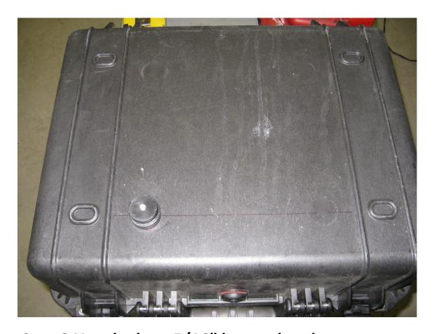
Step 8 Use the long 5/16" button head cap screw and 1 ½" aluminum washer to attach the master puck to the box.
