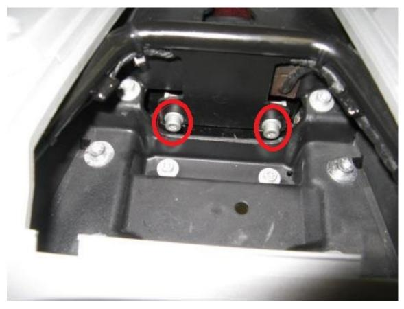
Step 2 Remove the trunk cover then remove the 2 M6 torx head screws shown.
