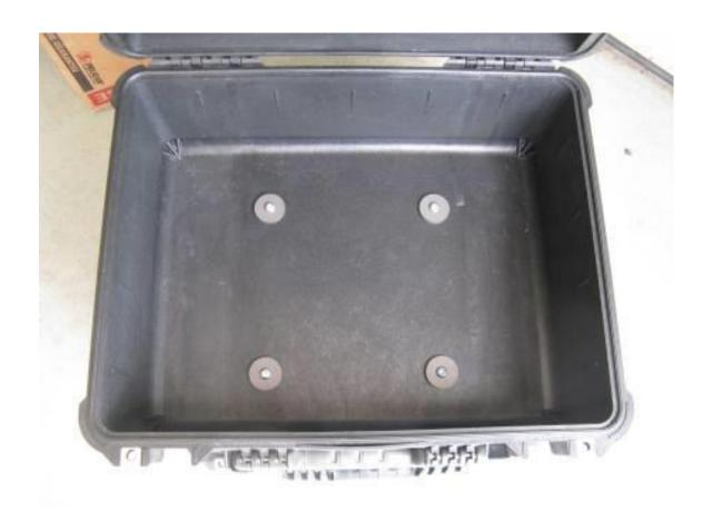
Step 14 Install all pucks onto the box using the 1 ½" aluminum washers and 5/16" button head cap screws.
