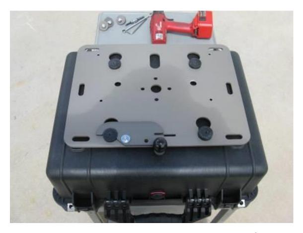
Step 4 Place the box on a table or other work surface. Remove the 4 flat head screws and nuts holding the rack onto the stainless steel brackets.
