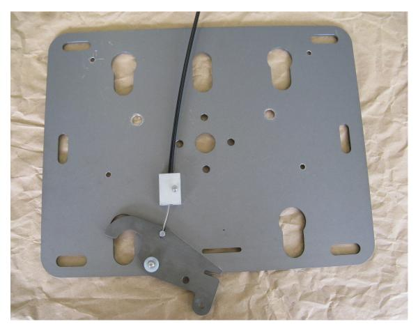
Step 17 Install the lever onto flat head bolt as shown. Attach the cable to the lever as shown. Install the second nylon washer onto the flat head bolt.
