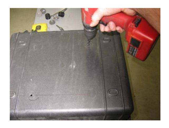
Step 11 Remove the rack and pucks from the box. Use the 21/64" drill bit and electric drill to enlarge the second 1/4" pilot hole.
