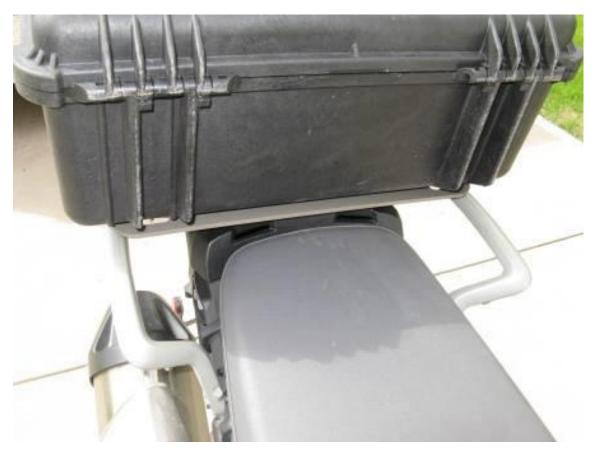
Step 2 Place the top box on top of the pucks and position it where you would like it located.
