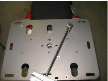
Step 8 Torque the 4 stainless steel bracket cap screws to 100 in. lbs. Use the front keyholes and access holes to reach the screw heads as shown.
