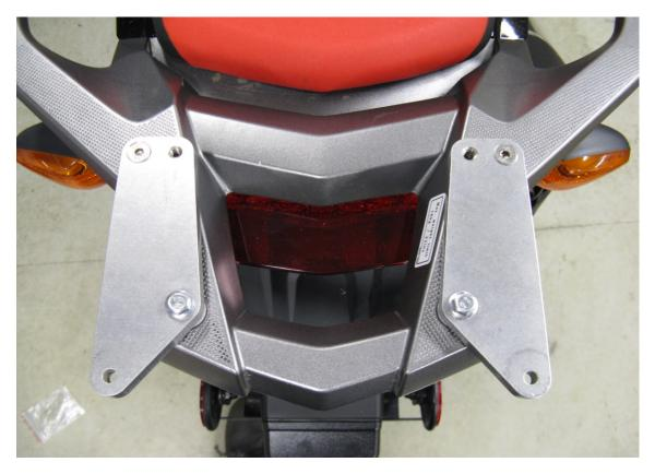
Step 2 Install the mounting brackets as shown. There is a RH and a LH mounting bracket. The counter sunk holes in the brackets go towards the front and outside of the bike. Insert 2 of the long 6mm flat head screws (front) and the 2 flange hex head screws (rear). Go to next step.
