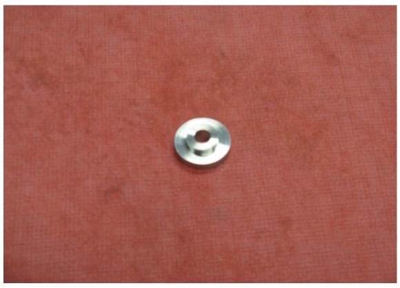
Step 3 Install the 4 hat shaped spacers underneath the OEM rack. These slip over the 4 screws installed in Step 2. The small diameter of the spacer faces upward and slips into the hole in the OEM rack. Install a 6mm lock nut on each of the screws. Do not fully tighten the nuts at this time.
