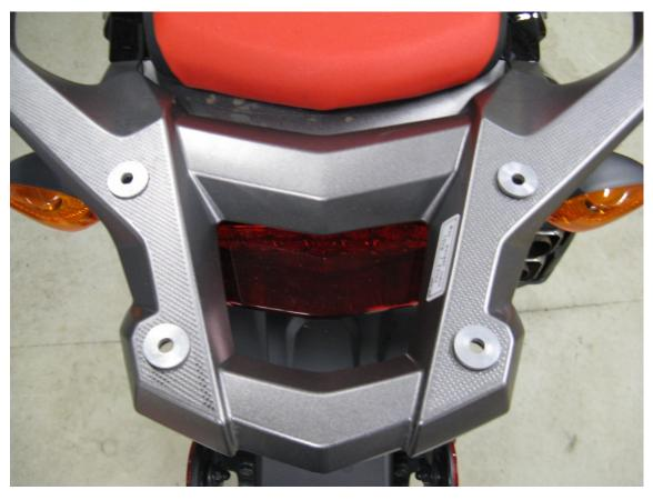
Step 1 Install the 4 short spacers into the holes on the OEM rack as shown.
