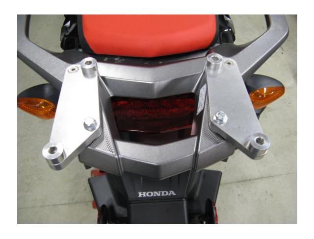
Step 4 Place a long spacer over each of the holes in the mounting brackets as shown.
