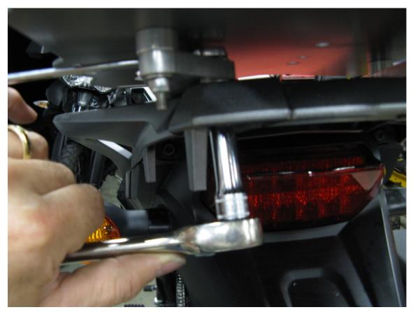
Step 8 Using a 10 mm open end wrench hold the flange hex head screws while tightening the 2 rear 6 mm lock nuts.
