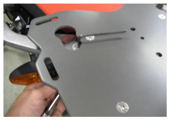
Step 7 The mounting brackets are still slightly loose at this time, check the position of the the plate on the bike, adjust the position if necessary (the amount of movement is very small, you are just trying to perfectly square the plate to the bike now.) Using a hex key wrench and 10 mm socket and ratchet tighten the 2 front lock nuts.
