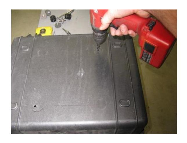
Step 17 Remove the rack and pucks from the box. Use the 21/64" drill bit and electric drill to enlarge the second 1/4" pilot hole.
