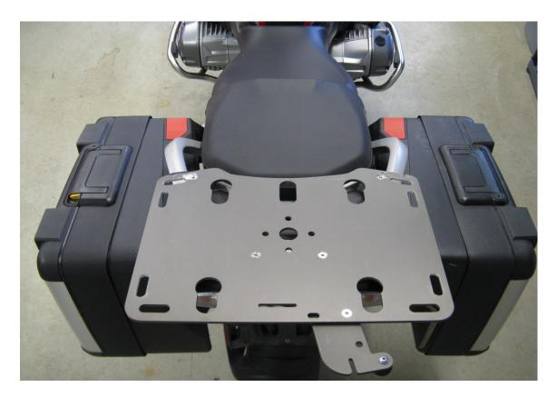
Step 5 Install the BRE rack using the four 6 mm x 40 mm flat head screws. Torque the four 6mm screws to 7.5 ft lbs (90 in lbs). Do not torque at this time if you are just test fitting for top box placement.
