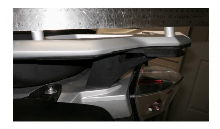
Step 4 Rotate the aluminum spacers so that the angles create a flat surface that is parallel to the OEM rack.
