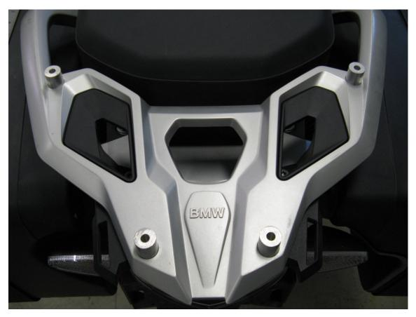
Step 3 Install the four aluminum spacers with the turned end inserted into the OEM rack.
