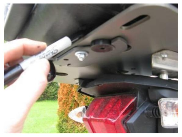
Step 8 Mark the location of the master puck onto the top box with a marker.
