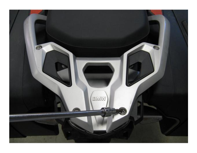
**Step 1 Remove the 4 OEM Torx head fastners.**
