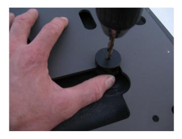
17. Bolt the remaining 2 pucks onto box using the remaining 5/16" button head cap screws and thick gray washers. Torque all 4 puck button head cap screws to 12 foot pounds.
