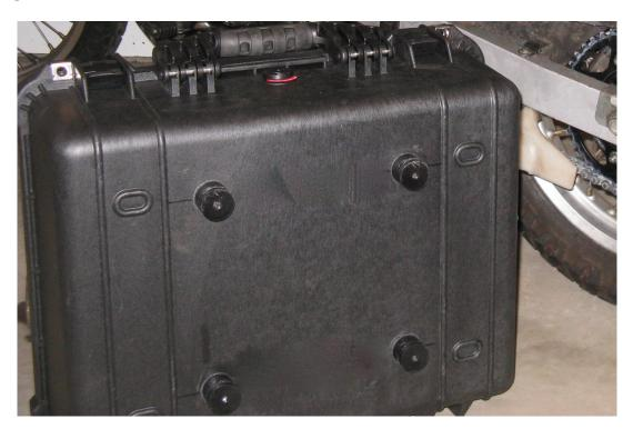
18. Fasten the rack to the motorcycle with the four 6 mm button head cap screws with the four flat washers. (Blue 242 Loctite is recommended on the treads) Torque the fasteners to 100 inch pounds. (Note: tool kit has been removed in this photo, the tool kit can remain in tact while mounting the rack.). This completes the rack installation.
