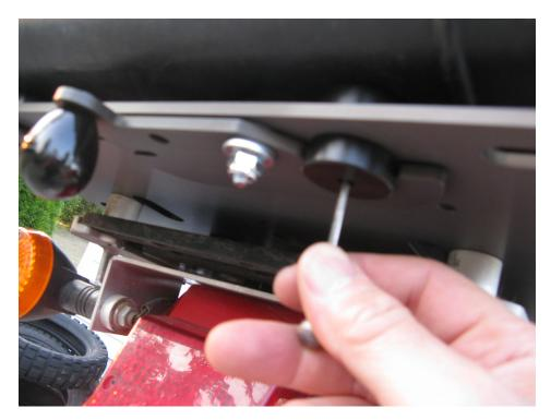
9. Remove the top box from the motorcycle and place it upside down on a flat work surface. Remove the rack from the motorcycle and place it on top of the box.
