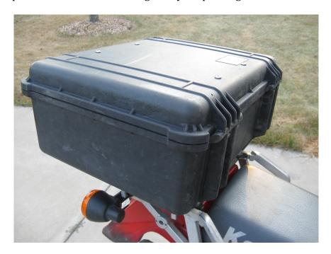
7. Use a tape measure to aid in positioning the top box. Positioning does not have to
