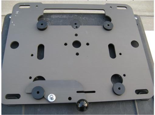
10. Locate the scribe mark and align the center hole of the latched puck with the scribe mark.
