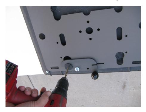
13. Remove the rack from the box. Use a 21/64" drill bit to enlarge the 1/4 " hole to a 21/64" hole. Remove the latched puck from the rack. Use the long 5/16" button head cap screw and a thick gray washer to fasten the thick puck to the box.
