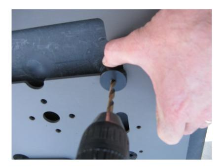
15. Unlatch and remove the rack from the box. Use a 21/64" drill bit to enlarge the 1/4" hole. Use a 5/16" button head cap screw and thick gray washer to mount the puck to the box (large diameter of the puck faces the box).
