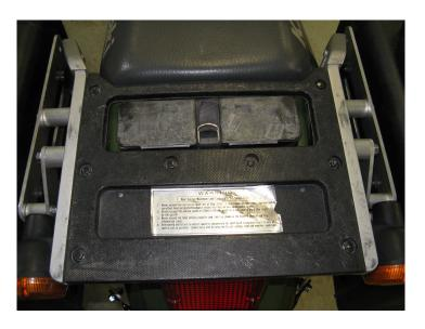
2. Insert the four aluminum spacers over the locations where the screws were removed.
