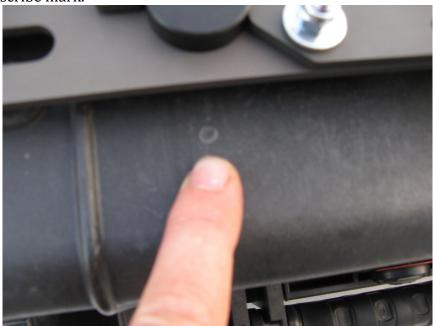
11. Make the final adjustments to the location of the box on the rack. Use a tape measure to center the box side to side, use the scribe location to locate the box front to rear.
