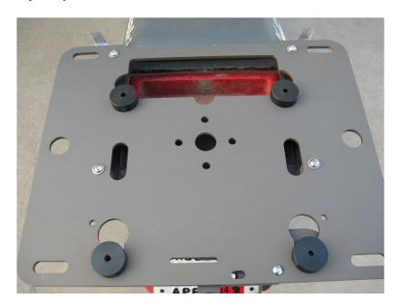
6. Set your top box on top of the pucks on the rack. Position the box where you want it to be mounted. When locating your top box it should be mounted as far forward as possible with out interfering with your passenger or seat removal.
