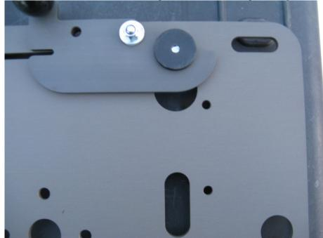
14. Seat the puck farthest from the mounted and latched puck into its keyhole. Have a helper hold the rack squarely on the box. Check with a square or tape measure to verify the rack and box are square to each other. Using the ¼" drill bit, drill the second hole in the box using the puck as a drill guide.
