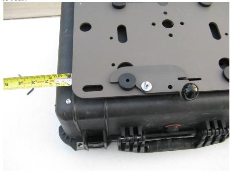
12. Have a helper hold the rack firmly in place on the box. Use a ¼" drill bit and an electric drill to drill through the box. Use the latched puck as a drill guide. This hole is the master hole, be certain the box is located correctly.
